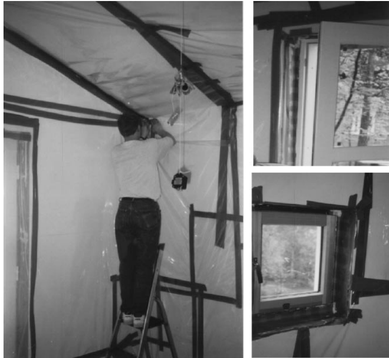
Fig. 2.3 Sealing the test room with polyethylene plastic (from Simonson et al., 2004)
