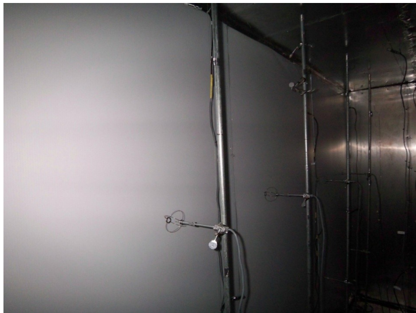
Fig. 4.1 Non-hygroscopic test: wood panels were covered by plastic sheets (Plaskolite 4 mm x 1220 mm x 2435 mm)
