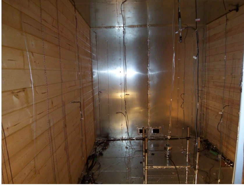
Fig. 4.2 Hygroscopic test: wood panels were subjected to moisture loads generated inside the room.
