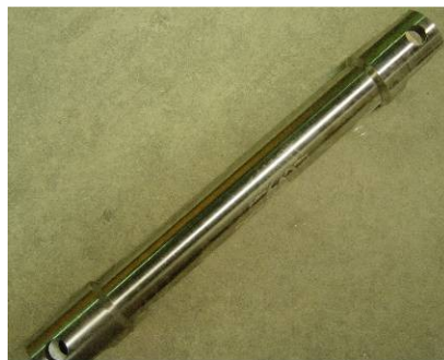
Figure 3.17: Manufactured lateral load cell for the test setup. Load cell was made by installing four strain gauges and then calibrated before the conducting the first test
