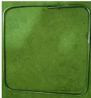
Figure 3.13: Steel ties, prepared using steel bars with the diameter of 4.75 mm
