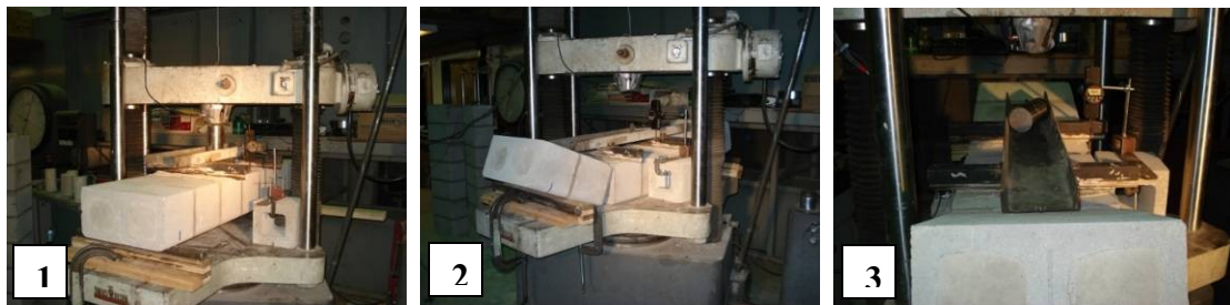
Figure 3.8: (1) test setup to obtain tensile strength of masonry assemblage ( f_t ), (2) and (3) 7 blocks prisms under third point loading at failure.
