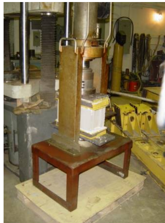
Figure 3.2: Obtaining compressive strength of concrete masonry units
