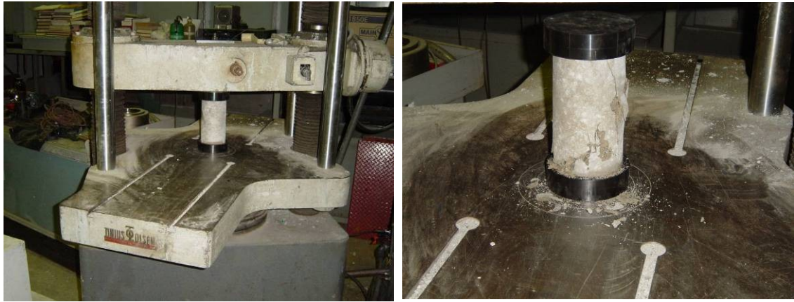
Figure 3.4: Obtaining compressive strength of grout cylinders
