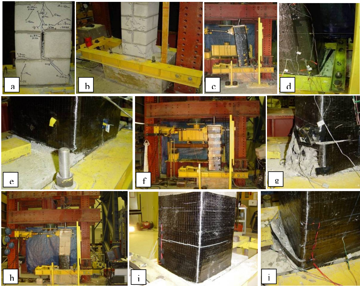
Figure 4.3: Performance of the CFRP-wrapped columns at different stages of the tests including observed cracking pattern and behaviour at failure
