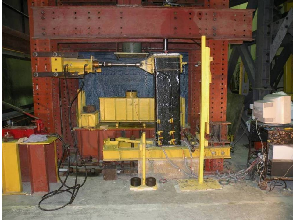
Figure 3.18: Test setup and lateral loading system in experimental program. This picture was taken from the test setup of column RMC-CW-3
