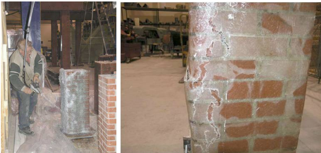
Figure 2.10: (left) GFRP spray process, (right) Failure of GFRP laminates (Shaheen and Shrive, 2005)
