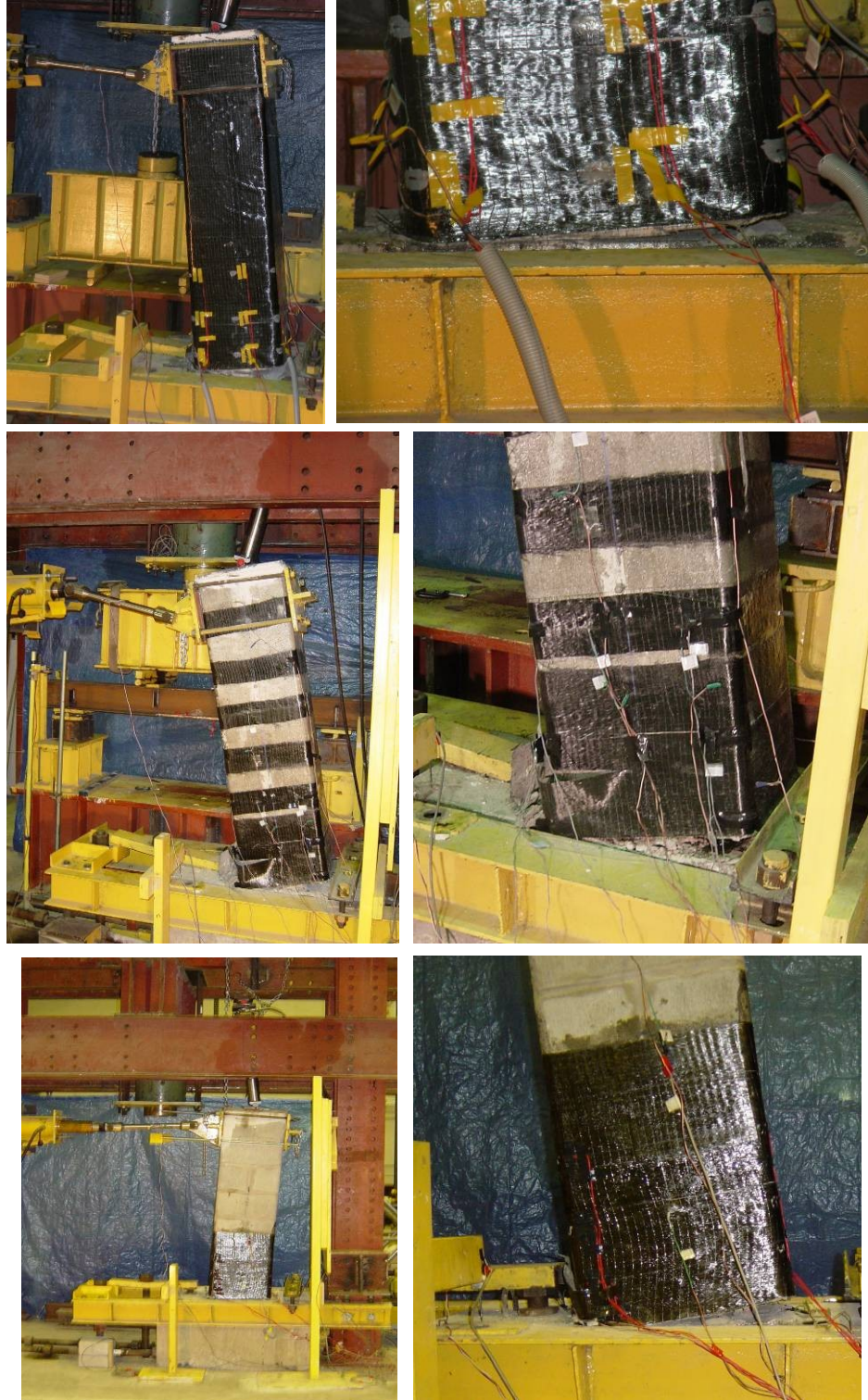
Figure 6.3: Occurrence of bond-slip at column-footing interface at high lateral drifts in columns C-CW-3, RMC-W-1S, and RCM-CW-1P
