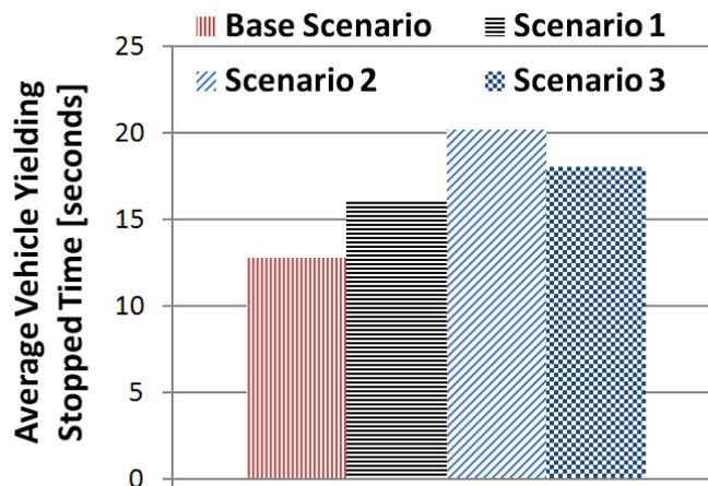
Figure 5.9: Effect of yielding maneuver on vehicle stopped time
