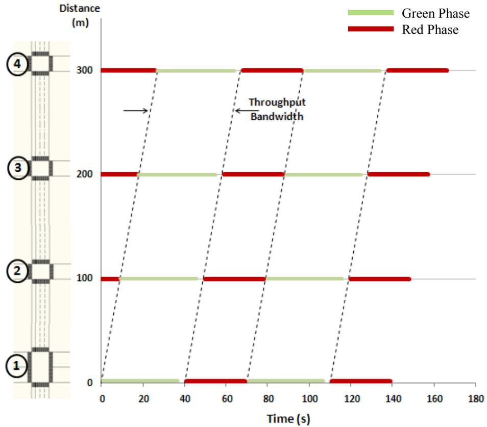
Figure 5.12: Signals coordinated to promote vehicle progression along 4-intersection corridor
