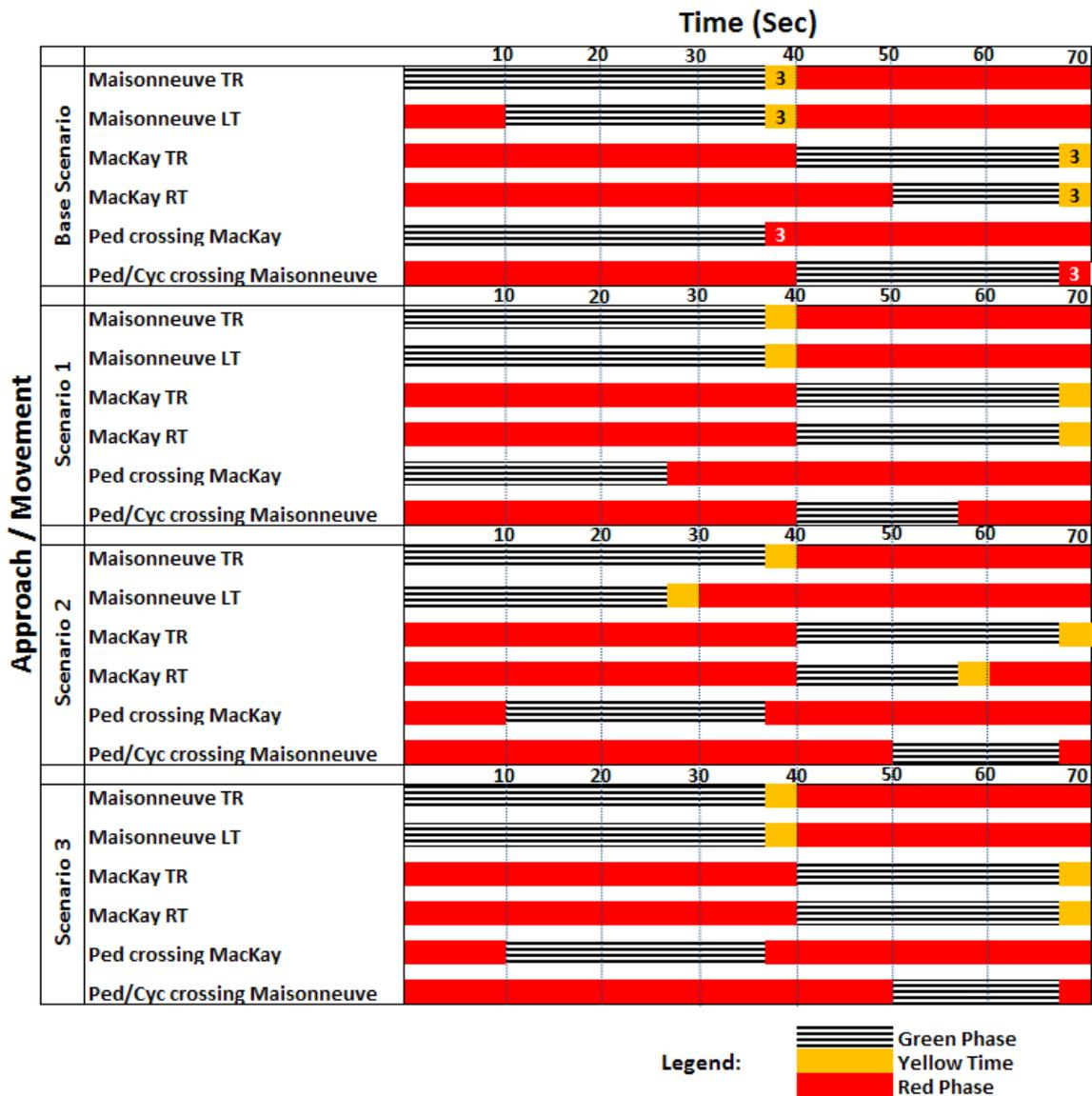
Figure 5.5: Signal timing plan scenarios
