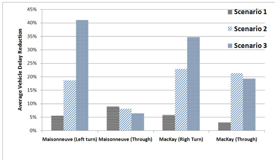
Figure 5.8 : Reduction in average vehicle delay for the alternative signal timing plans
