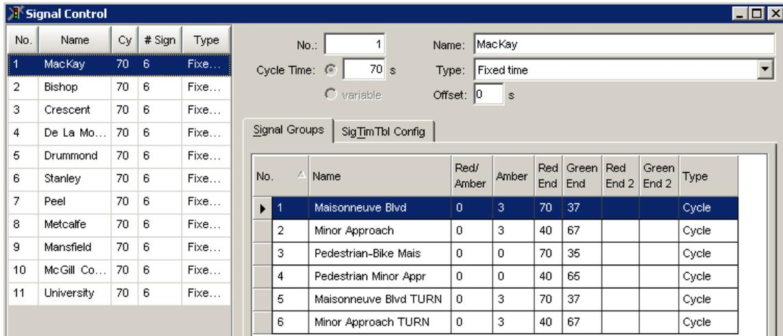
Figure 5.14: Implementation of Signal Controllers in VISSIM
