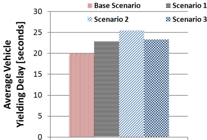
Figure 5.7: Effect of yielding maneuver on vehicle delay
