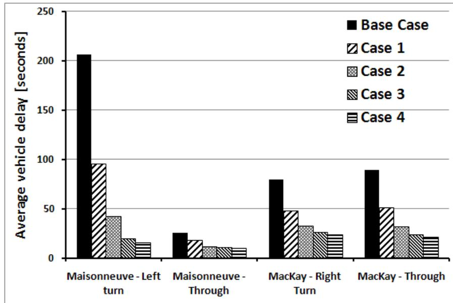
Figure 5.2: Effect of alternative pathways on the vehicle delay
