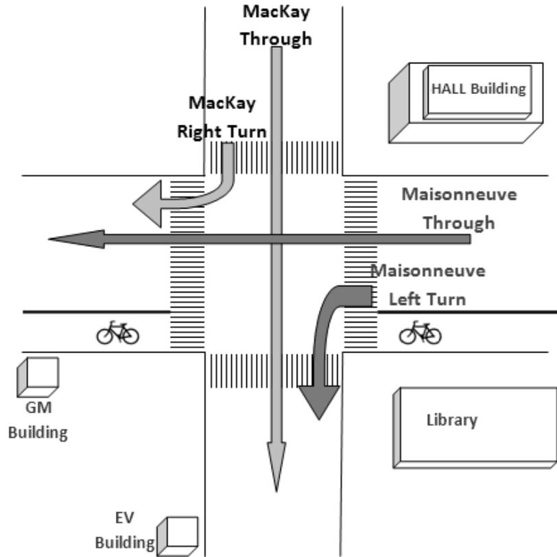
Figure 4.2: Layout of critical intersection & vehicle movements
