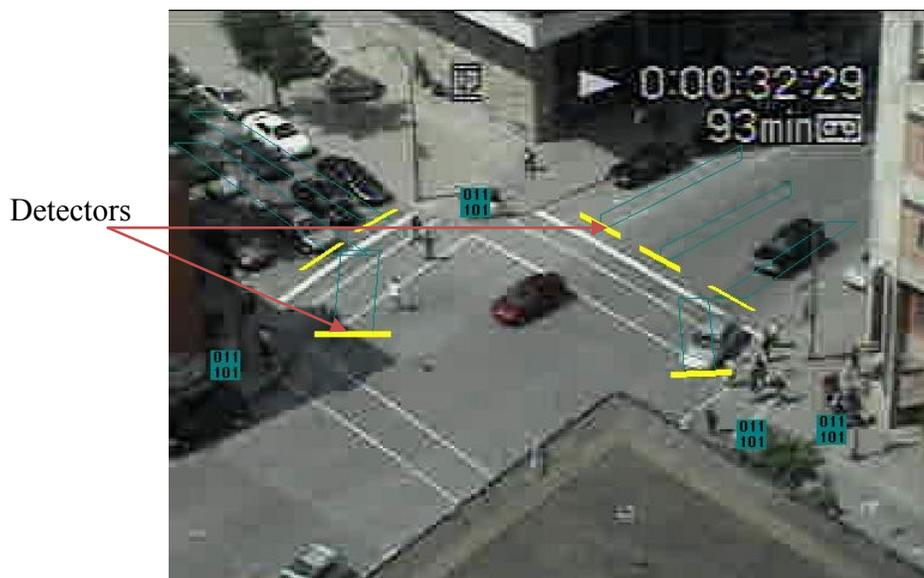
Figure 4.4: Defining detectors for Autoscope
