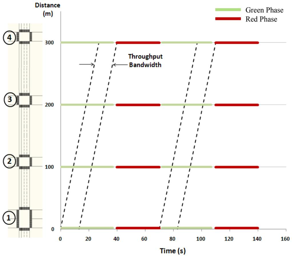
Figure 5.11: Independent signal timing plans along 4-intersection corridor
