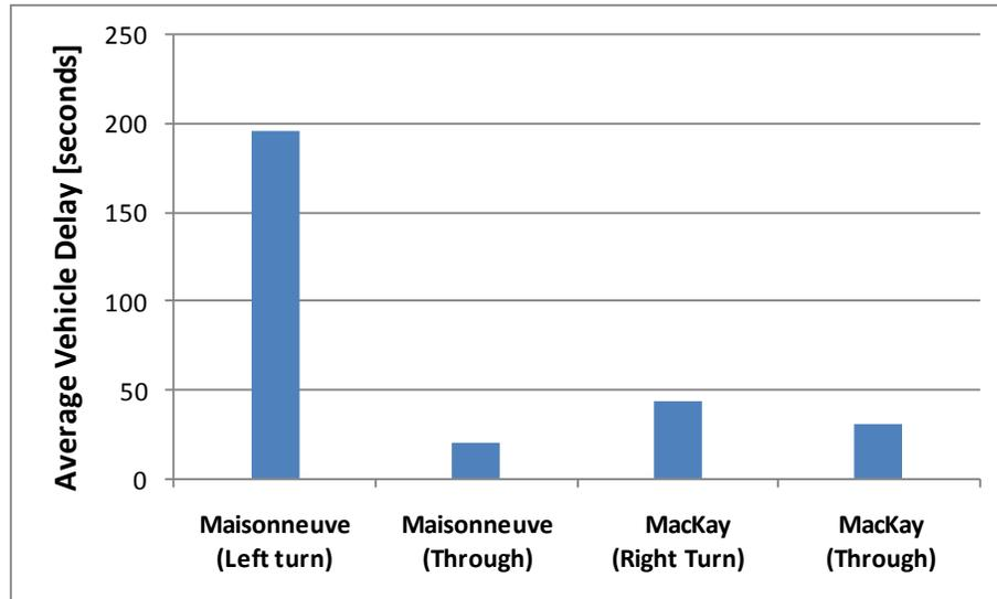
Figure 5.6: Base scenario average vehicle delay for each movement
