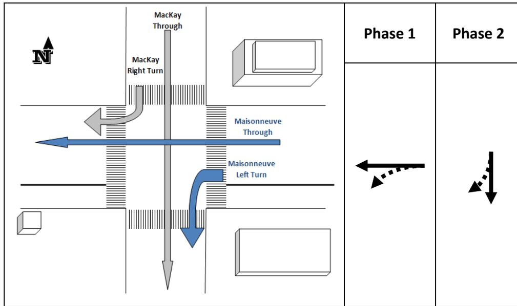
Figure 5.1: Signal plan for critical intersection
