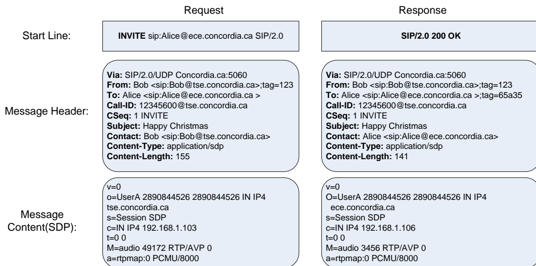
Figure 2.9 Structure of SIP Request and Response
