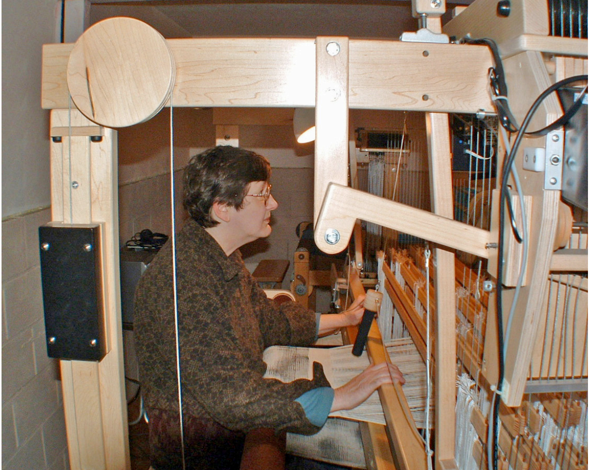
Fig. 14. North American Weaver Using Computer-assisted Loom (2005). She still sits close to the work, and operates the lifting, throwing, and beating with her body. The loom mechanism extends her memory by ‘storing’ the pattern. She can feel the tension of the threads when she presses the beater, throws the shuttle, and presses the treadles to lift the threads. Photo by Beryl Moody.
