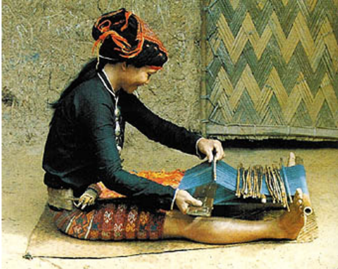
Figure 13. Vietnamese Backstrap Weaver (n.d). Her body provides the tensioning frame for the loom, while the mechanism of sticks with string heddles attached to warp threads provides the ‘memory’ for making the complex pattern in the cloth. (Ministry of Foreign Affairs, Government of Vietnam.)
