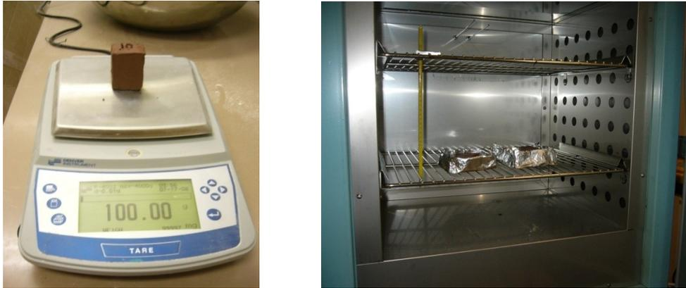
Figure 3.1 Verification of percentage of water content for specimen
