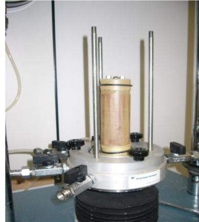
3.5 Airtight specimen in latex sleeve (Graph source: Das, 2005)
