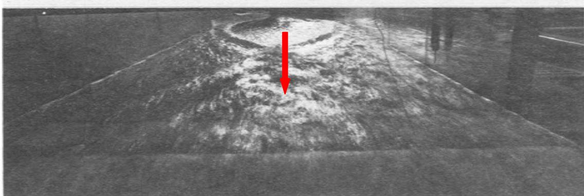
Figure 3.2 Visible shock waves emerging downstream of a channel expansion. The flow is from the top to the bottom, as indicated by the thick arrow. The flow approaching the expansion is supercritical with the Froude number greater than one (adopted from Mazumder and Hager, 1993).
