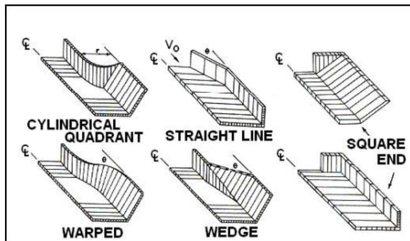
Figure 2.1 Channel expansion types (from U.S. Department of Transportation 1983, Chapter 4). All the expansions have geometry symmetric about the centreline.
