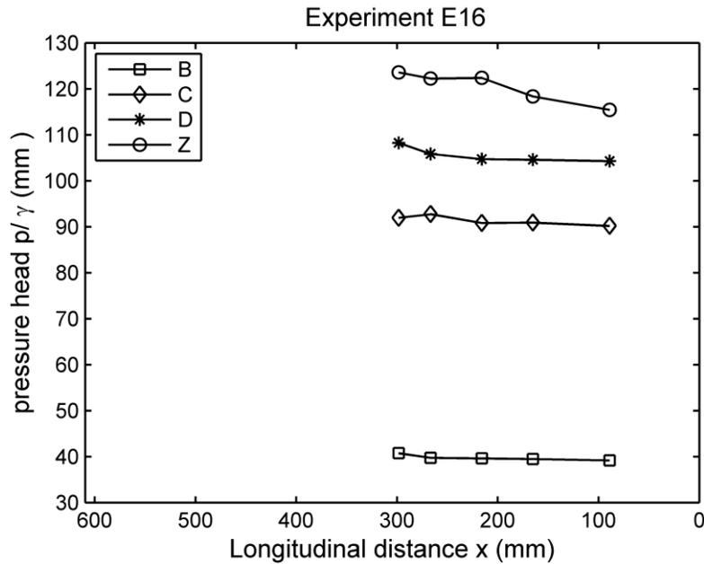
Figure 5.4 Longitudinal variations in pressure head shown for selected experiments. The flow is from right to left. The conditions of the experiments are listed in Table 5.1. The upstream and downstream ends of the expansion are located at  $x = 0$  and 304.8 mm, respectively. A sudden increase in pressure head is possibly due to eddy motion.
