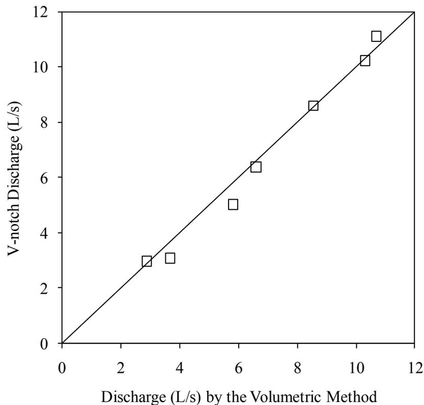
Figure 5.1 Correlation of discharge measurements using the V-notch weir and the volumetric method.
