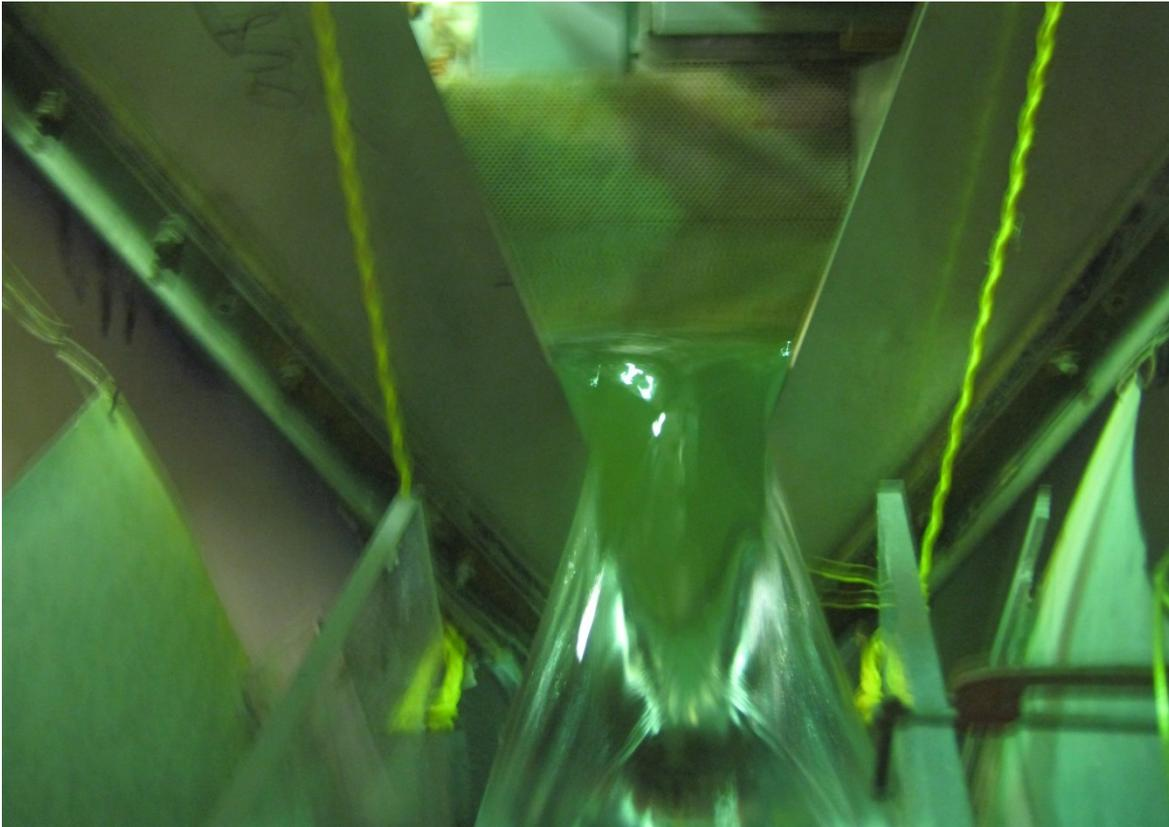
Figure 4.4 The 30° V-notch weir used in the laboratory for discharge measurements.
