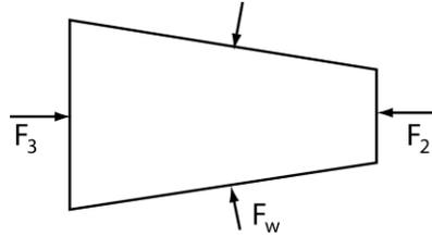
Figure 3.5 Free body diagram for momentum analysis.
