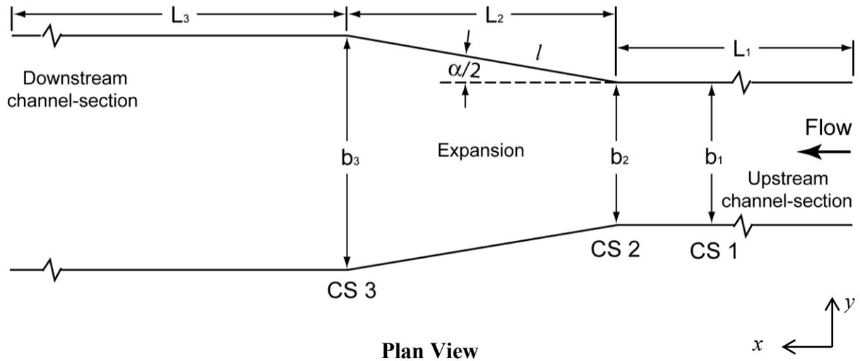
Figure 3.1 Definition diagram of a channel expansion, showing the length of the expansion and the lengths of the upstream and downstream channel-sections. The expansion has a divergence angle  $\alpha$ , with its width changing from  $b_1$  at its upstream end (CS 2) to  $b_3$  at its downstream end (CS 3). The corners are blunt. The flow is from right to left.
