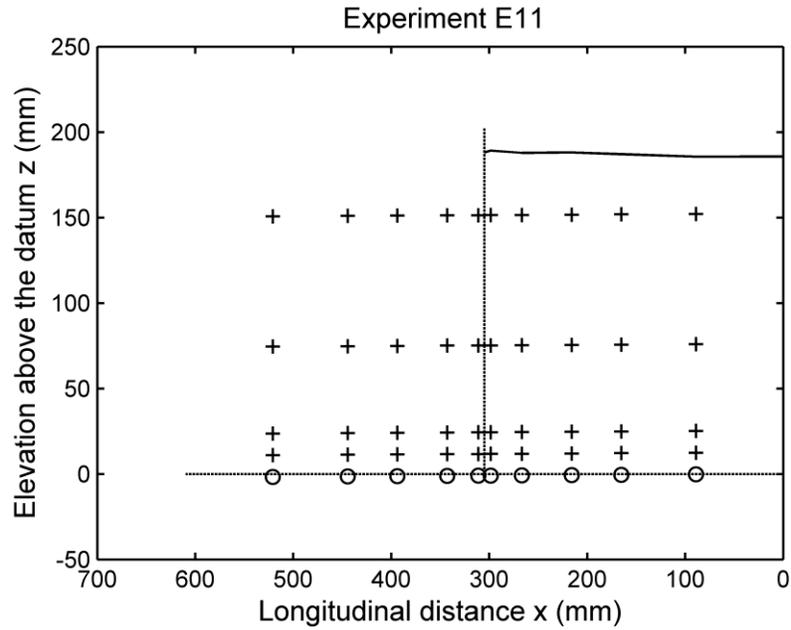
Figure 5.3 Positions of pressure taps drilled through the sidewall (marked by the symbol +) of the expansion and at the channel bottom (marked by the symbol o). The flow is from right to left.
