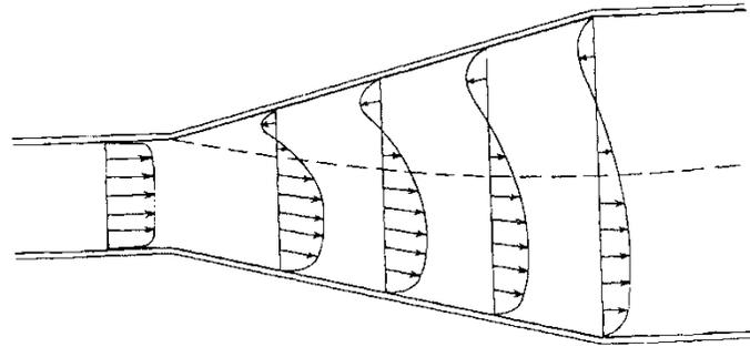
Figure 2.2 Plan view velocity distribution for a rapid expansion:  $B/b = 3.0$  (Smith and Yu 1966).
