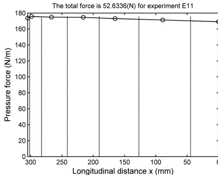
Figure 5.8 Subdivided areas for the calculation of the pressure force on the sidewall of the expansion. The sidewall force for experiment E11 is  $F_w = 52.6$  N.
