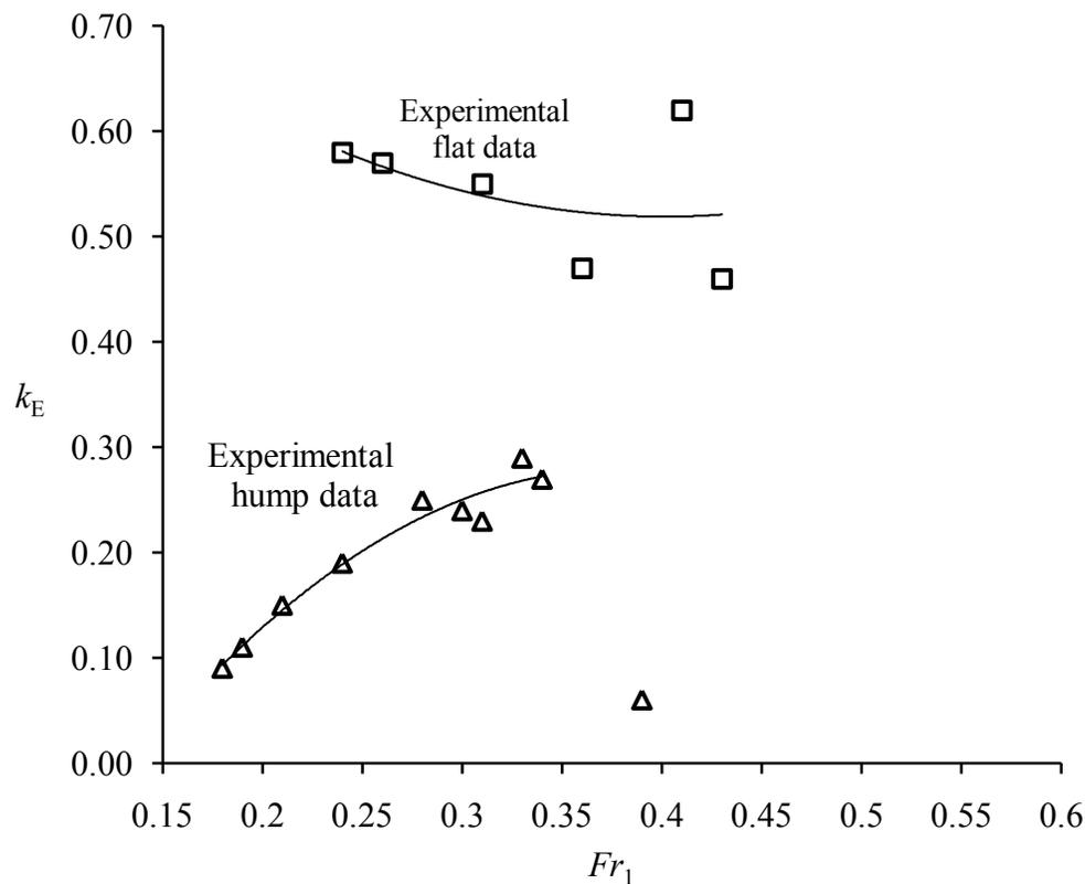
Figure 6.1 Energy loss coefficients (indicated by the symbol  $\Delta$ ) for the experiments with the hump. The energy loss coefficients (indicated by the symbol  $\square$ ) for the experiments without the hump are plotted for comparison.
