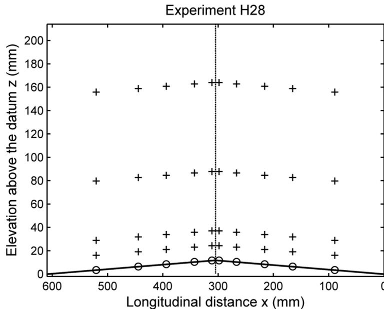
Figure 6.2 Positions of the pressure openings. The expansion is between  $x = 0$  and  $x = 323.3$  mm
