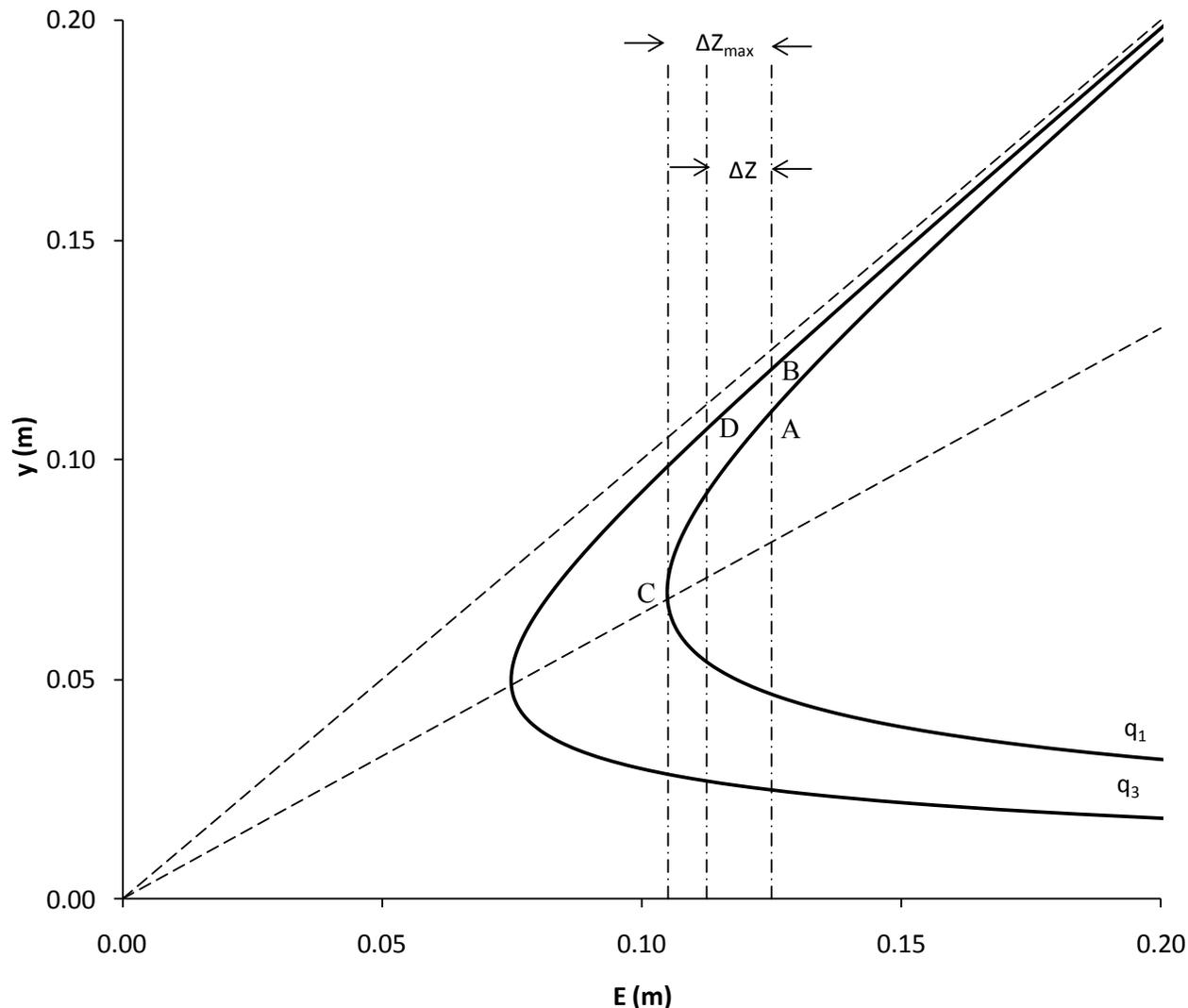
Figure 3.3 Specific energy diagram for flow in a channel expansion. The E-y curve to the right (the  $q_1$  curve), shows all possible depths of flow and corresponding specific energy, with a per-unit-width discharge of  $q_1$ . The  $q_3$  curve is similar to the  $q_1$  curve, but the per-unit-width discharge is  $q_3 < q_1$ . In the limit of zero energy loss in a horizontal channel, the depth of subcritical flow increases in the direction of the flow.
