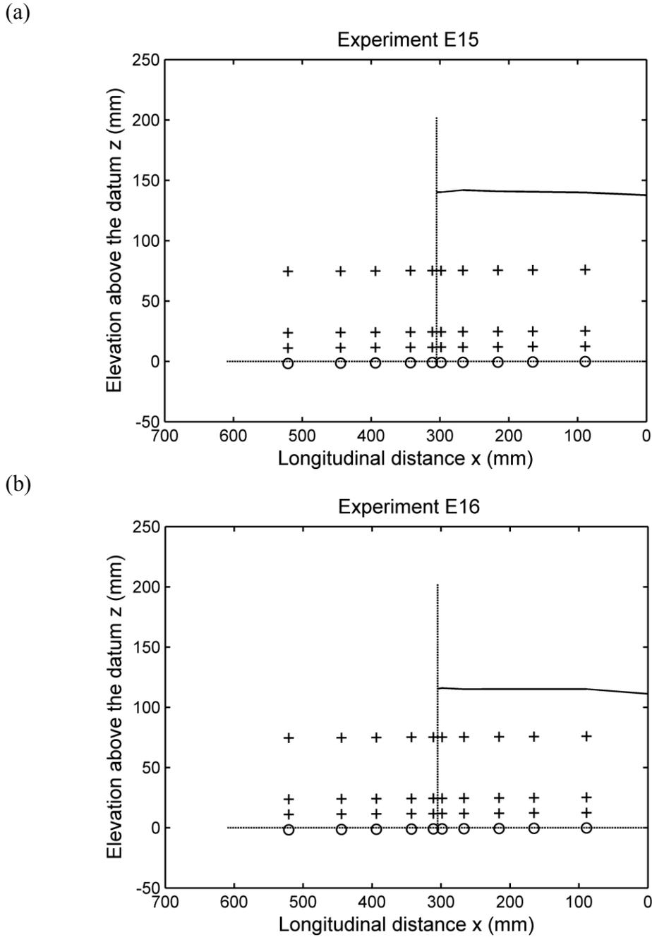
Figure 5.5 Water surface profiles shown as the solid curves above the pressure taps. The sidewall pressure taps are marked by the symbol +, and the bottom pressure taps are indicated by the symbol o.
