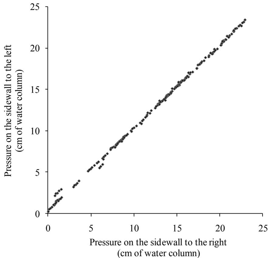
Figure 6.3 Comparison between water pressures measured at corresponding pressure openings through the sidewall to the left and the sidewall to the right (facing downstream). The pressure is expressed in height (cm) of water column.
