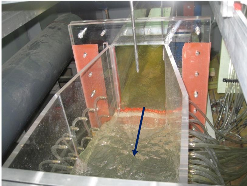
Figure 4.2 Channel expansion and 1/16" wall pressure taps through the wall and connected to piezometers. This photo shows the expansion with a hump fitted on the channel bottom.
