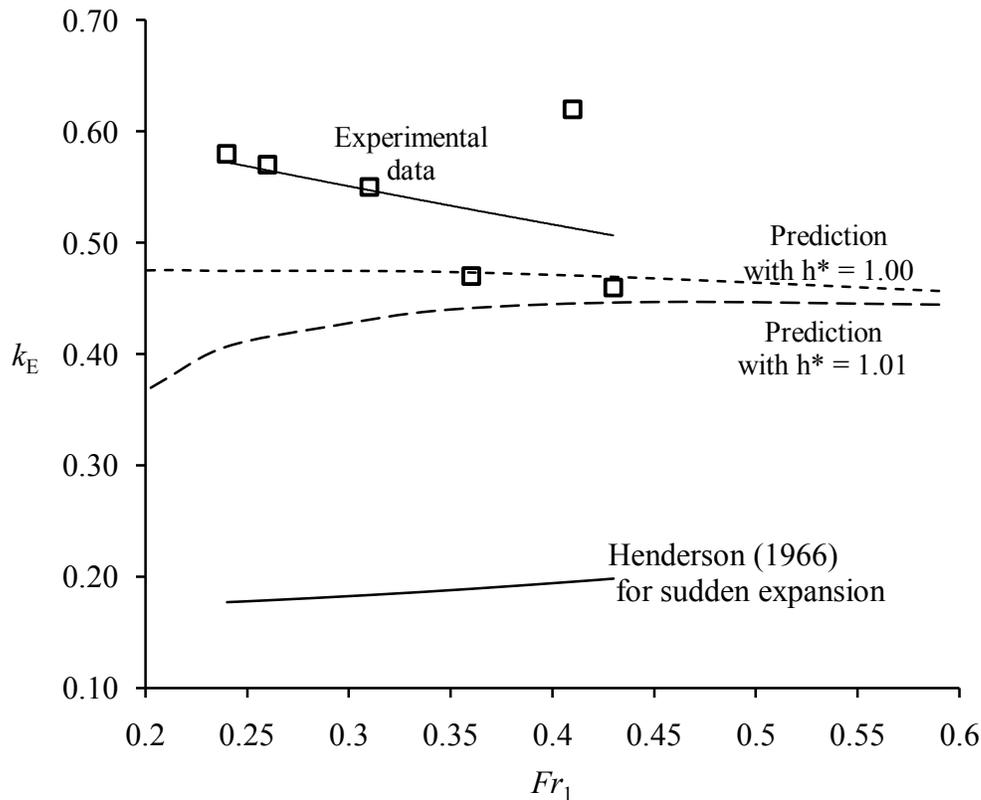
Figure 5.2 Comparisons of the coefficient of energy head loss between experiments and theoretical predictions. In the experiments the Froude number ranges from 0.24 to 0.43, and the coefficient is between 0.46 and 0.62. The dependence of  $k_E$  on the Froude number appears to be weak.
