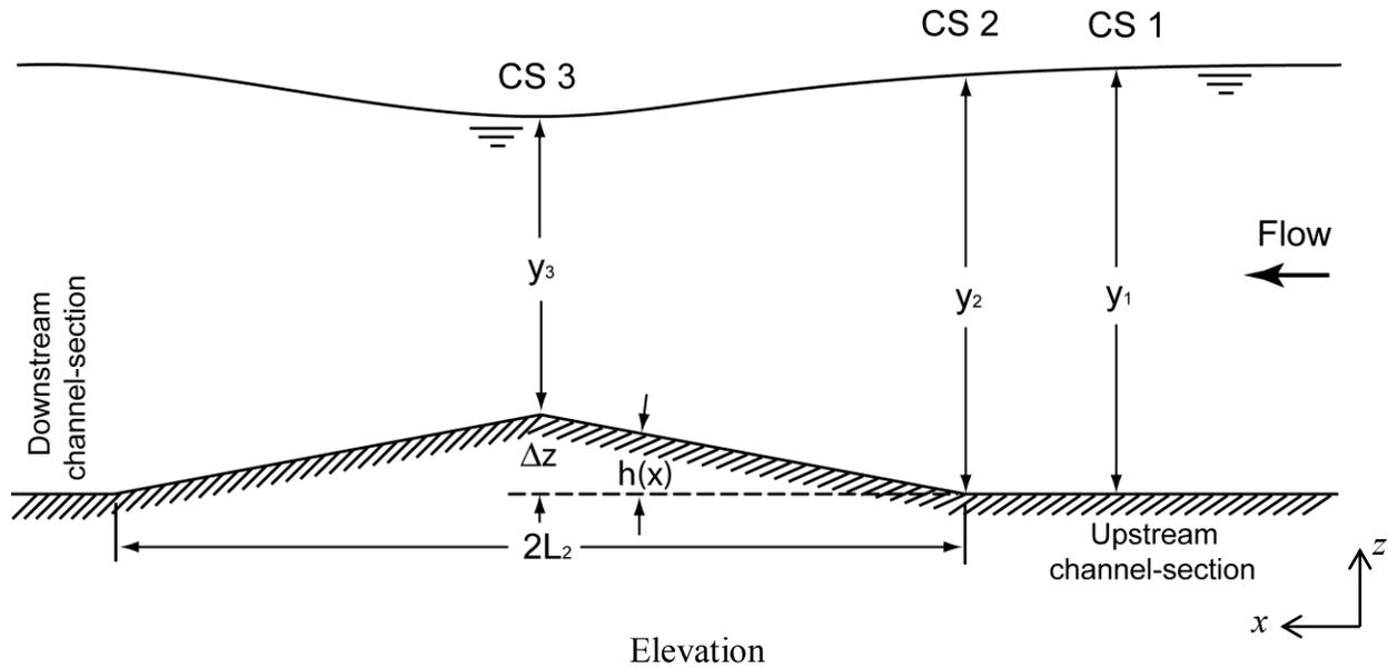
Figure 3.4 Water surface profile for flow over a hump fitted on the bottom of a uniform channel. From cross section CS 2 to cross section CS 3 the water pressure is decreasing while the flow accelerates up-slope. From CS 3 toward downstream the water pressure is increasing while the flow decelerates down-slope. On the basis of the energy principle, the depth of flow decreases over the hump.
