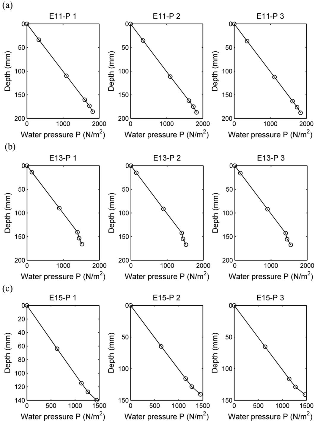
Figure 5.6 Measured pressures varying with depth below the water surface. The top, middle and bottom panels are for experiments E11, E13 and E15, respectively. For each of the experiments, P1, P2 and P3 correspond to pressure taps A1–Z1, A2–Z2, and A3–Z3, respectively.
