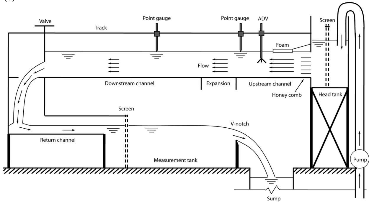
Figure 4.1 (a) Experimental setup used to conduct experiments in this study. (b) Schematic illustrations of the upstream channel-section, the expansion and the downstream channel-section. Measurement devices include point gauges, flow meters and a sharp-crested V-notch weir.
