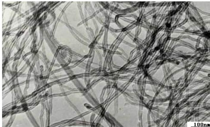
Figure 3.1 TEM for purified multiwall carbon nanotubes (MWCNTs) [87]
