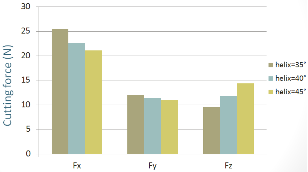
Figure 5.4. The plot of the maximum cutting force curve at different helical angles.
