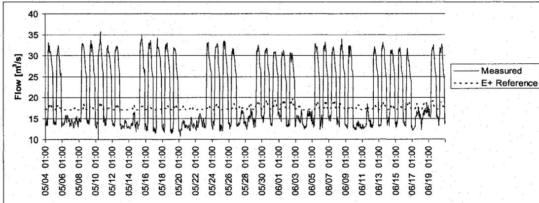
Figure 6.2: Airflow Rate Variation from May 4<sup>th</sup> to June 20<sup>th</sup>; Sectors B & C
