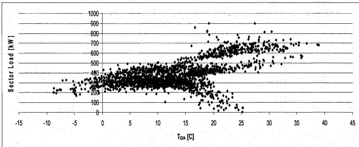
Figure 5.9: Sector Cooling Load versus Outdoor Air Temperature for the Spring Season; Sector A
