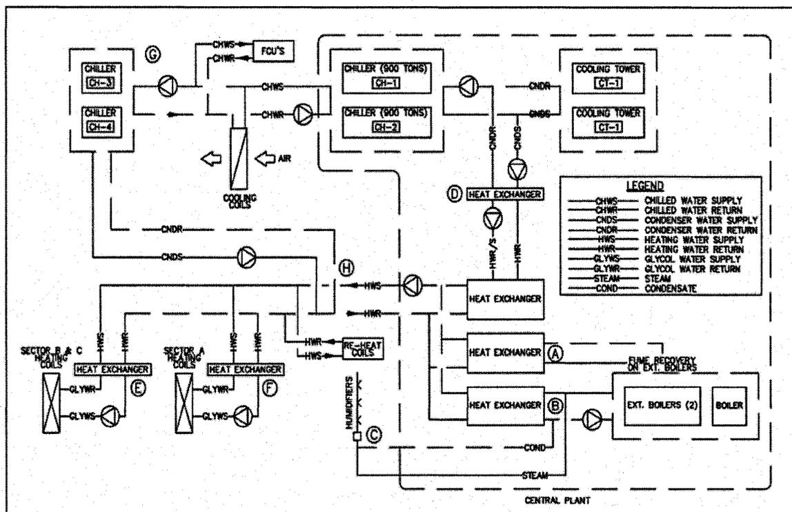
Figure 4.2: Simplified Schematic of HVAC Systems and Central Plant
