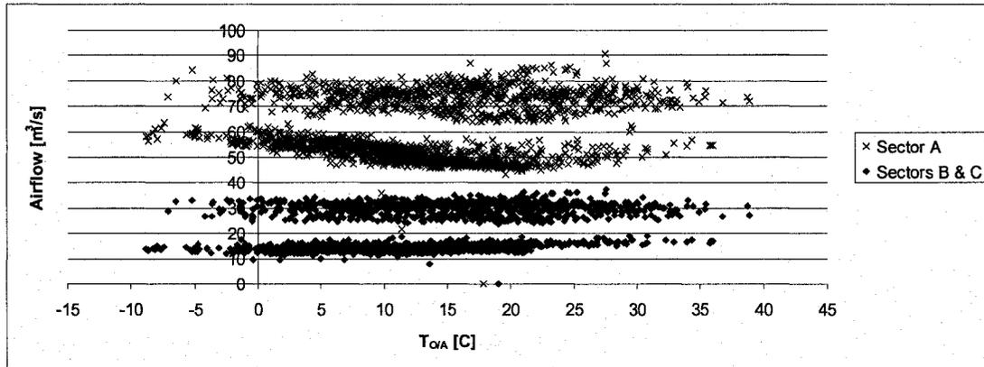
Figure 5.5: Variation of the Supply Airflow Rate with Outdoor Air Temperature for the Spring Season
