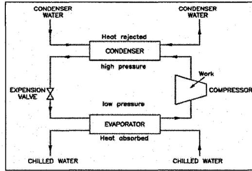
Figure 2.2: Diagram of Chiller [11]
