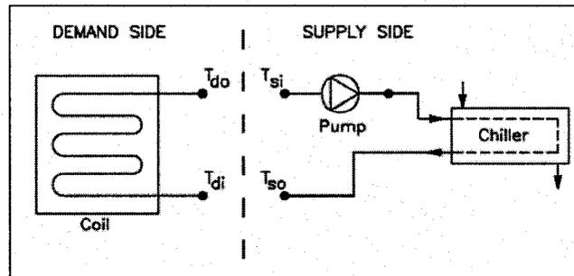
Figure 3.4: Example of Plan Loop Schematic [30]
