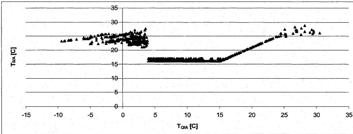
Figure 6.23: Predicted Supply Air Temperature versus Outdoor Air Temperature from March 20<sup>th</sup> to May 3<sup>rd</sup>; Sectors B & C
