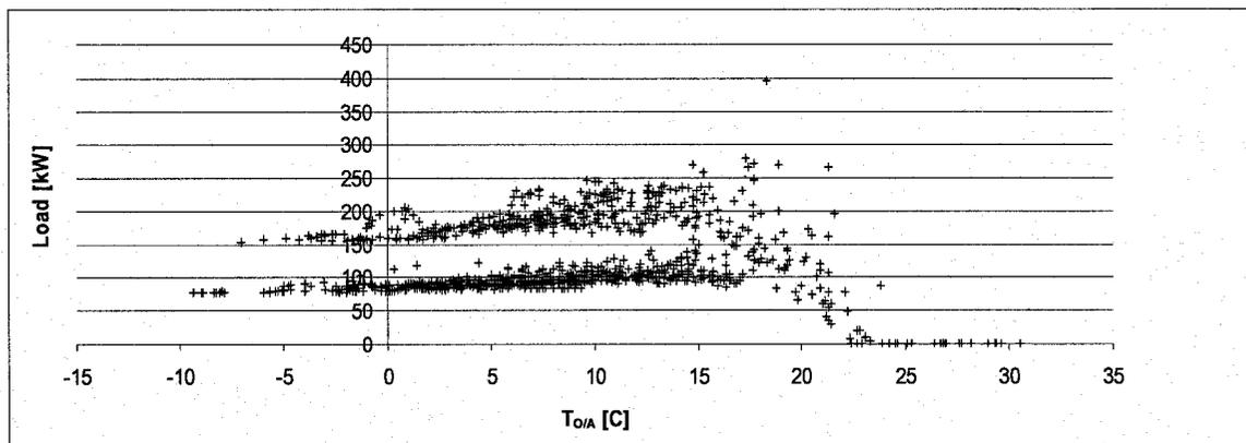
Figure 6.29: Estimated Sector Air-Side Thermal Load versus Outdoor Air Temperature from March 20<sup>th</sup> to May 3<sup>rd</sup>; Sectors B & C
