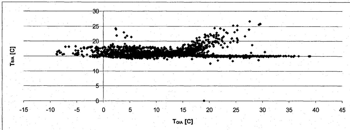
Figure 5.6: Hourly Values of Supply Air Temperature versus Outdoor Air Temperature for the Spring Season; Sectors B & C
