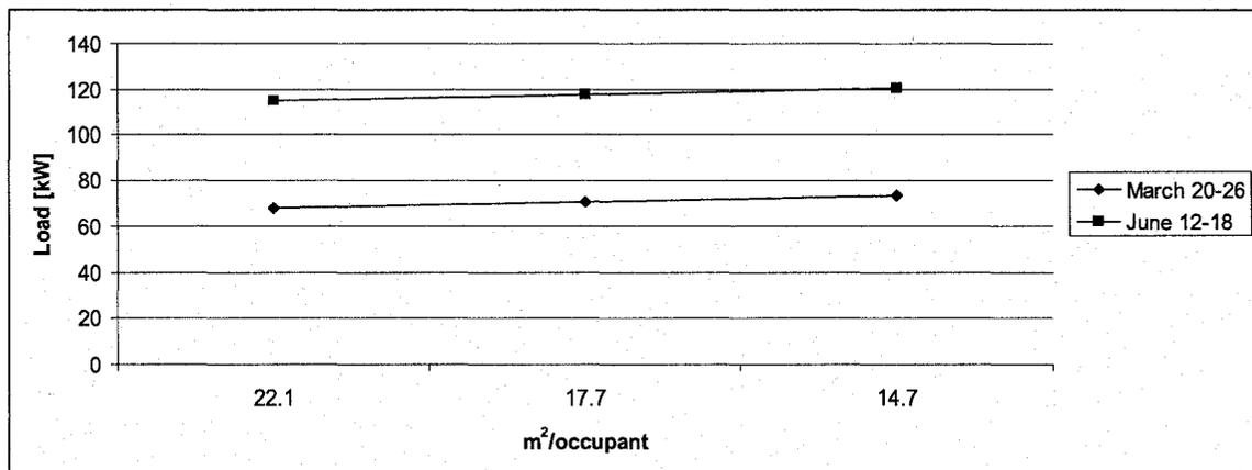
Figure 6.46: Variation of the Cooling Air-Side Thermal Load with Occupancy Level; Sectors B & C
