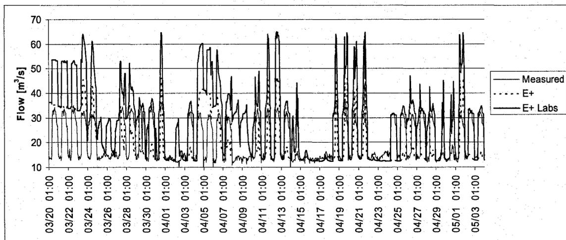
Figure 6.20: Airflow Rate Variation from March 20<sup>th</sup> to May 3<sup>rd</sup>; Sectors B & C
