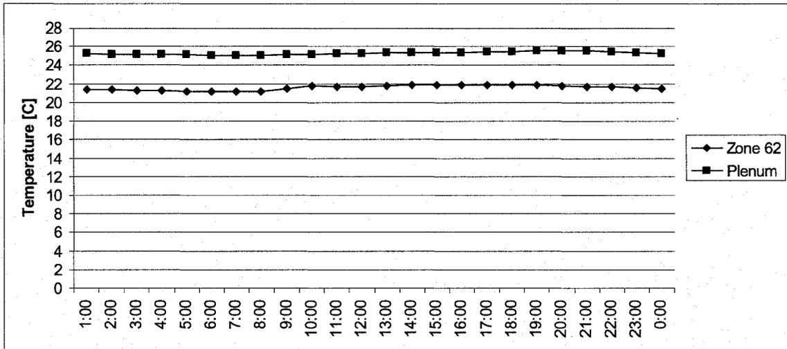
Figure 4.6: Direct Exhaust Plenum and Zone Temperature Variation during the Summer Design Day
