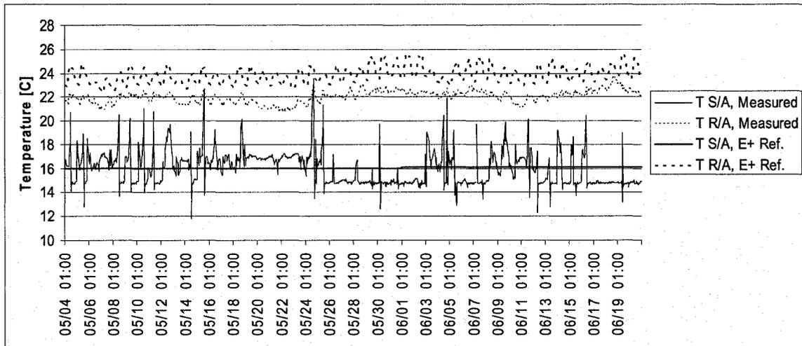
Figure 6.12: Air Temperature Variation from May 4<sup>th</sup> to June 20<sup>th</sup>; Sector A
