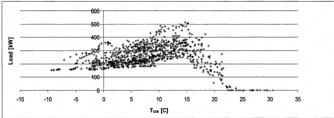
Figure 6.35: Estimated Sector Air-Side Thermal Load versus Outdoor Air Temperature from March 20<sup>th</sup> to May 3<sup>rd</sup>; Sector A
