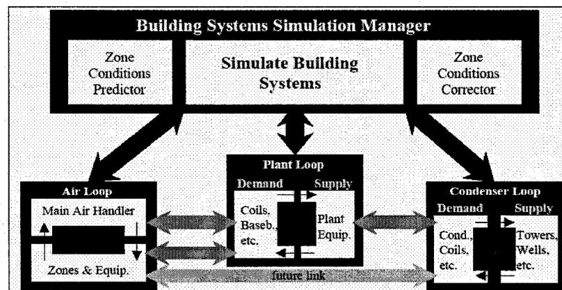
Figure 3.6: Loops Interaction for EnergyPlus Sizing [28]
