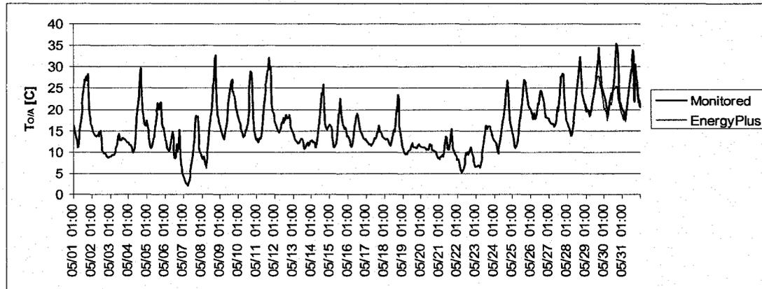
Figure 6.1: Revised Outdoor Air Temperature for the Month of May
