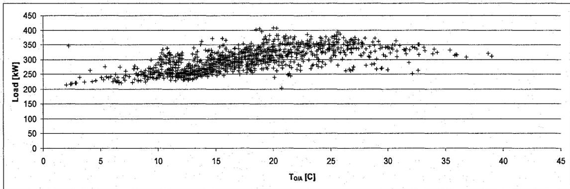
Figure 6.17: Estimated Sector Air-Side Thermal Load versus Outdoor Air Temperature from May 4<sup>th</sup> to June 20<sup>th</sup>; Sector A
