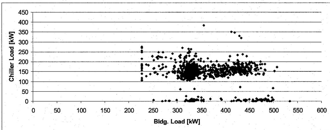
Figure 5.14: Chiller Load versus Building Load; March 20<sup>th</sup> to May 4<sup>th</sup>, 2006
