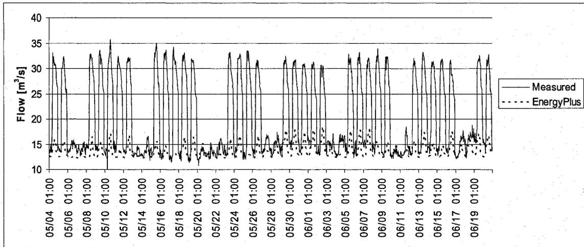
Figure 6.5: Revised Airflow Rate Variation from May 4<sup>th</sup> to June 20<sup>th</sup>; Sectors B & C
