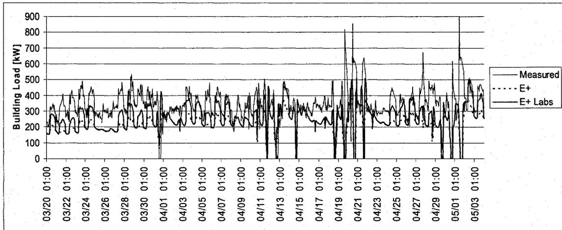
Figure 6.34: Sector Air-Side Thermal Load from March 20<sup>th</sup> to May 3<sup>rd</sup>; Sector A
