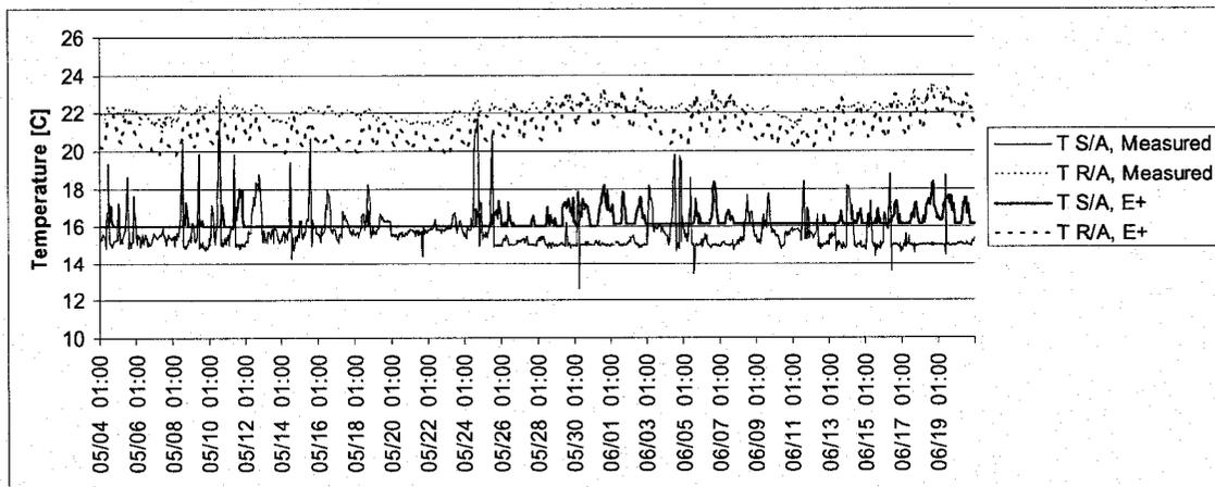
Figure 6.4: Revised Air Temperature Variation from May 4<sup>th</sup> to June 20<sup>th</sup>; Sectors B & C
