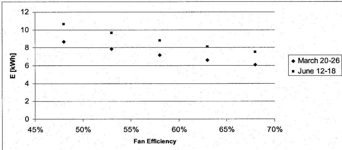
Figure 6.50: Variation of the Return Fan Electricity Consumption with Fan Efficiency; Sectors B & C
