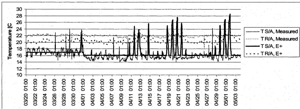
Figure 6.25: Revised Air Temperature Variation from March 20<sup>th</sup> to May 3<sup>rd</sup>; Sectors B & C
