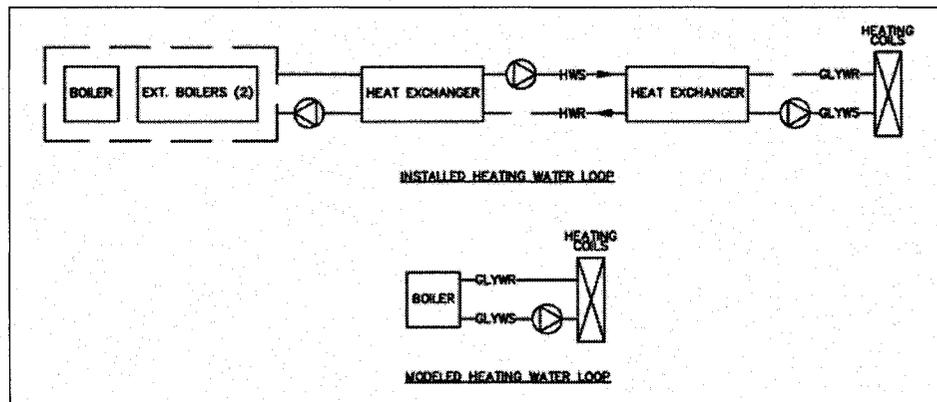
Figure 4.12: Heating Water Loop Schematic
