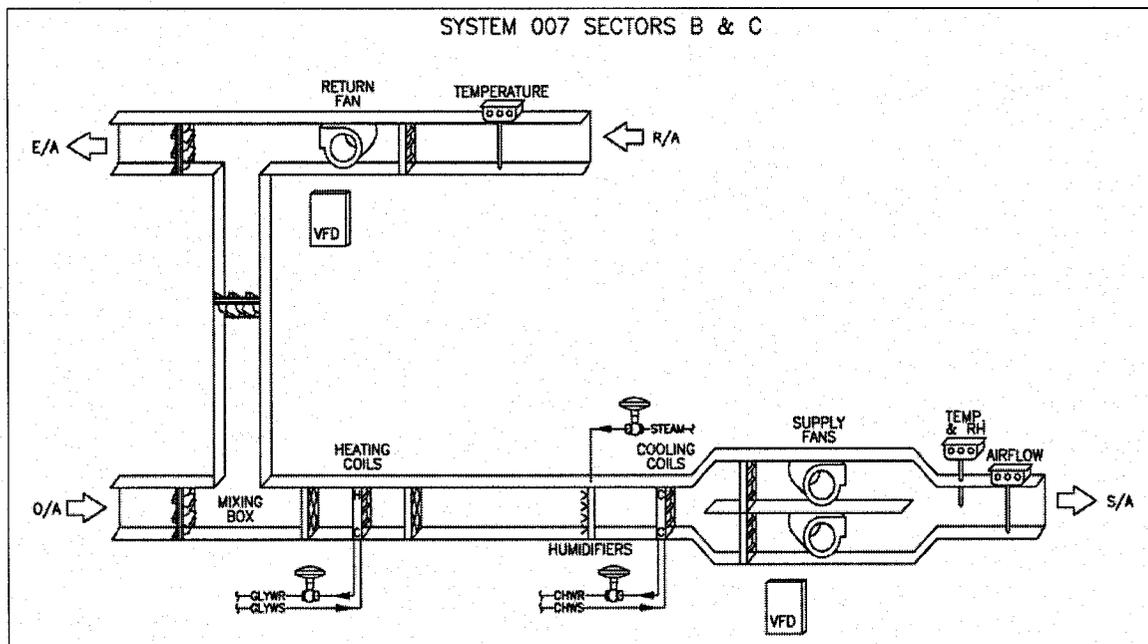
Figure 5.2: Capture of Display Software for Sectors B & C Air Handling Unit
