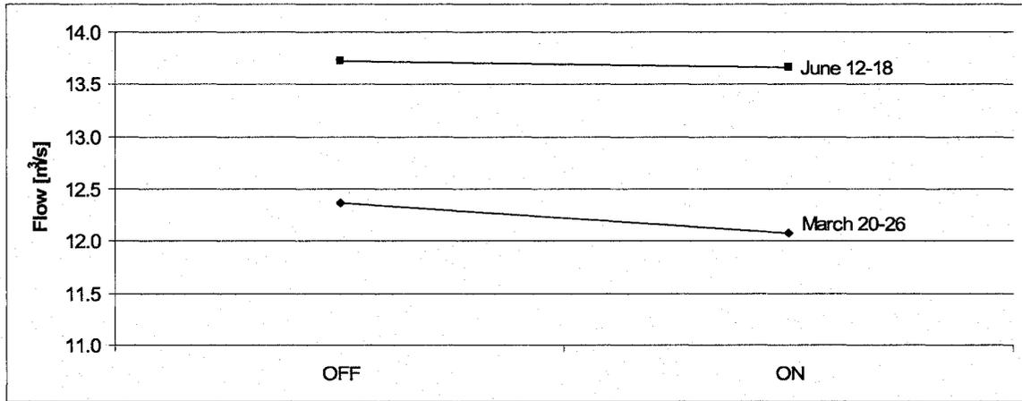
Figure 6.39: Variation of the Supply Airflow Rate without and with Air Infiltration; Sectors B & C
