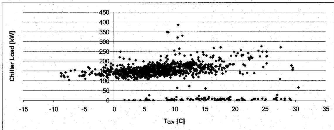
Figure 5.15: Chiller Load versus Outdoor Air Temperature; March 20<sup>th</sup> to May 4<sup>th</sup>, 2006
