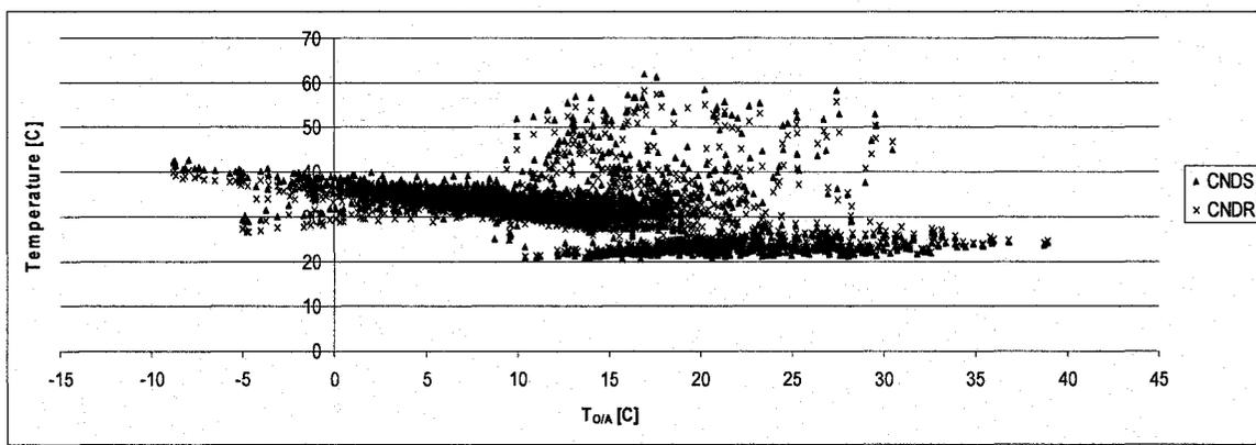
Figure 5.18: Condenser Water Temperature versus Outdoor Air Temperature over the Spring Season
