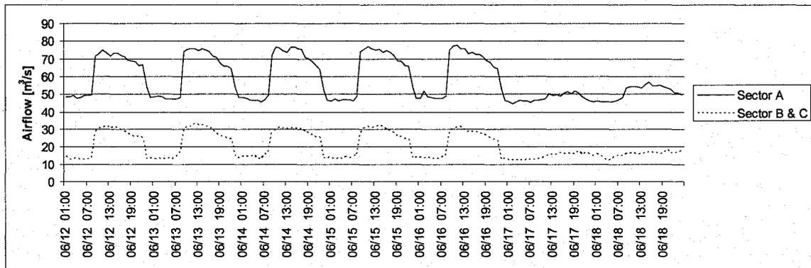
Figure 5.37: Airflow Variation for the Week of June 12<sup>th</sup> to June 18<sup>th</sup>
