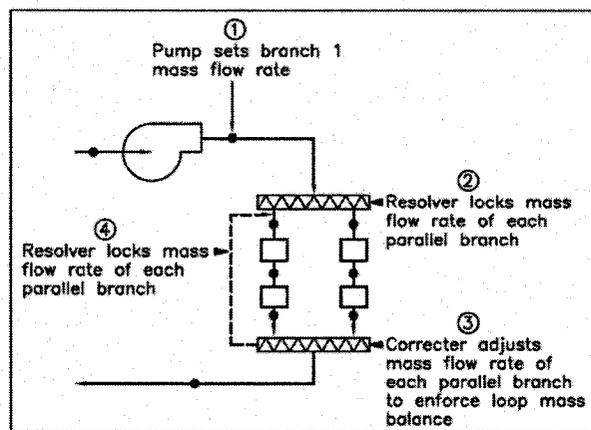
Figure 3.5: Plant Supply-Side Solution Scheme [29]
