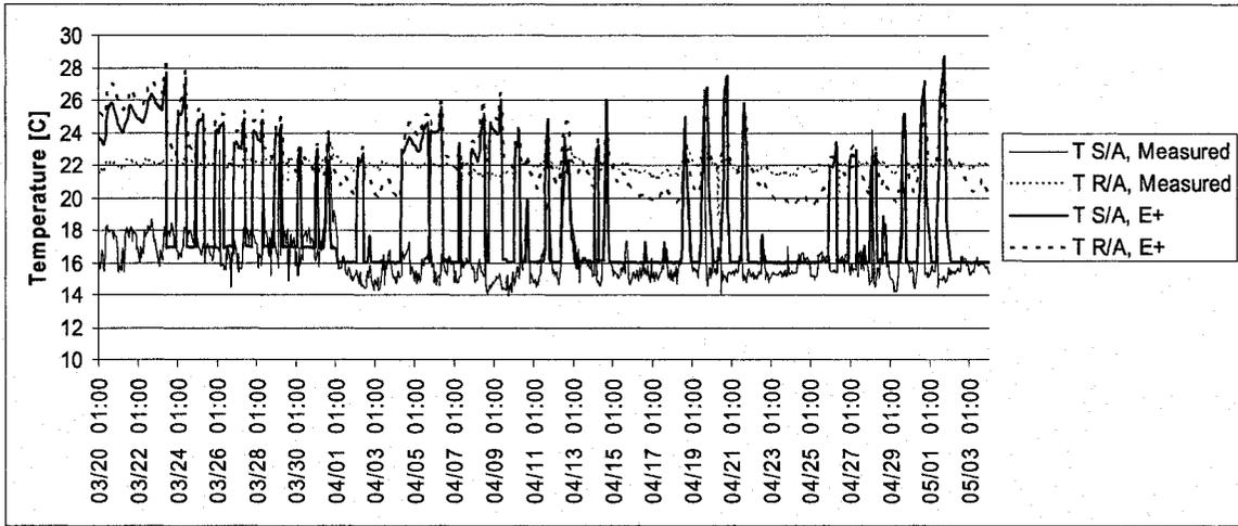
Figure 6.22: Air Temperature Variation from March 20<sup>th</sup> to May 3<sup>rd</sup>; Sectors B & C
