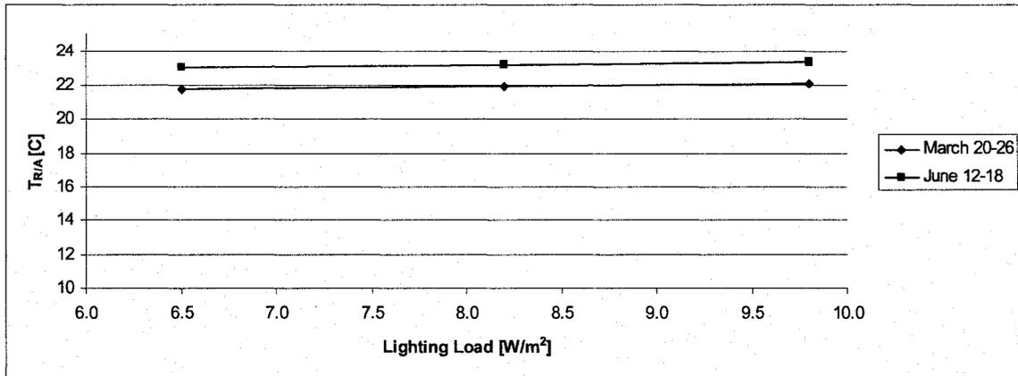
Figure 6.43: Variation of the Return Air Temperature with Lighting Load; Sectors B & C
