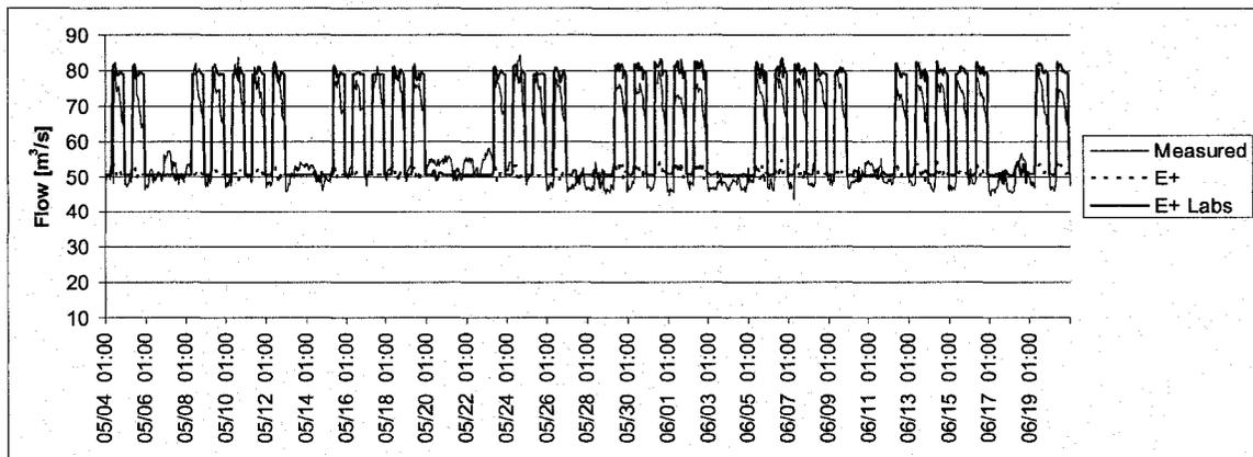
Figure 6.15: Airflow Rate including Laboratories Requirements from May 4<sup>th</sup> to June 20<sup>th</sup>, Sector A
