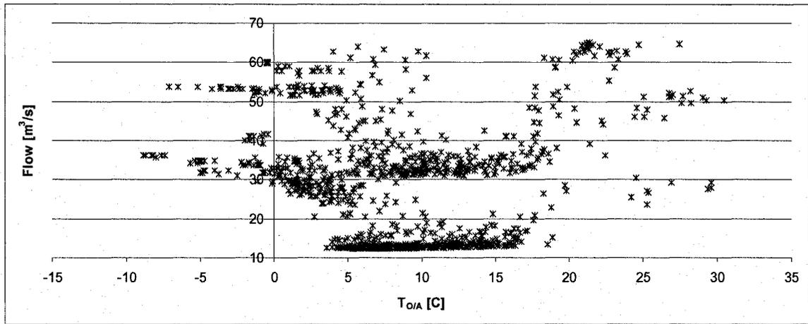
Figure 6.21: Predicted Airflow Rate versus Outdoor Air Temperature from March 20<sup>th</sup> to May 3<sup>rd</sup>; Sectors B & C
