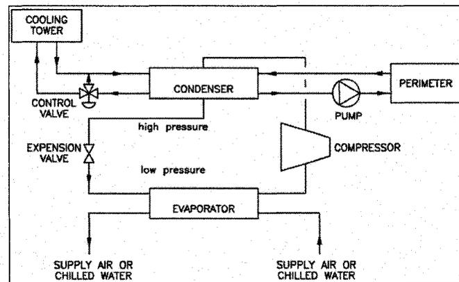
Figure 3.7: Diagram of Vapour Compression Chiller: Electric with Heat Recovery [29]
