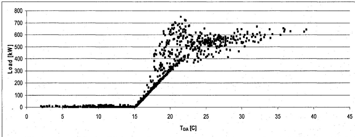
Figure 6.19: Estimated Cooling Coil Load versus Outdoor Air Temperature from May 4<sup>th</sup> to June 20<sup>th</sup>; Sector A
