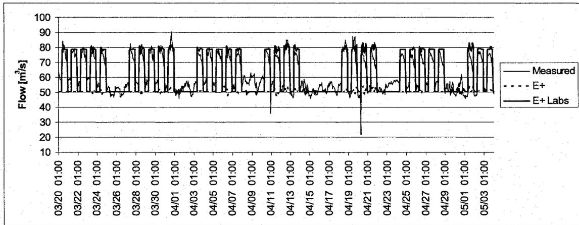
Figure 6.31: Airflow Rate Variation from March 20<sup>th</sup> to May 3<sup>rd</sup>; Sector A
