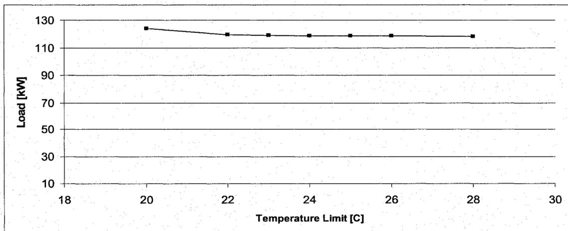
Figure 6.48: Variation of the Cooling Coil Load with Economizer Cut-Off Temperature; Sectors B & C
