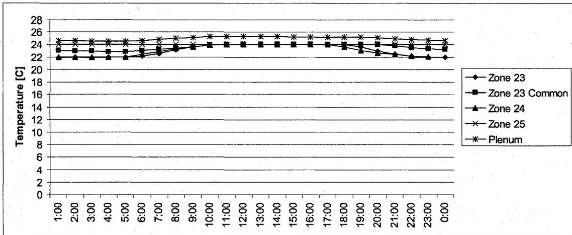
Figure 4.4: Plenum and Zone Temperature Variation during the Summer Design Day
