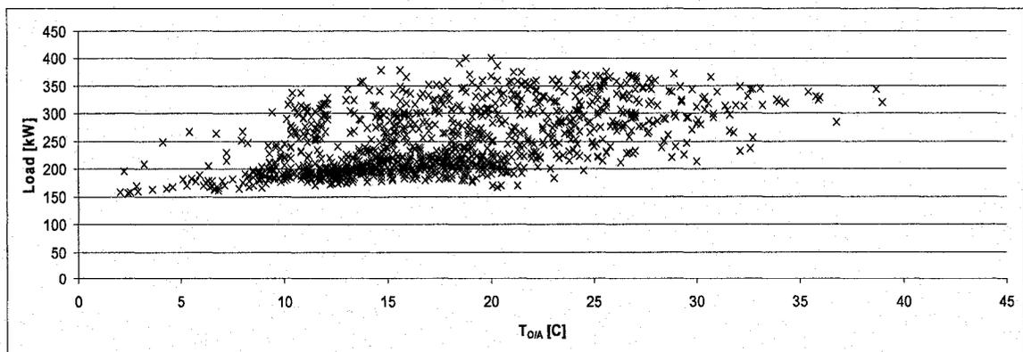
Figure 6.18: Estimated Thermal Load of all Zones versus Outdoor Air Temperature from May 4<sup>th</sup> to June 20<sup>th</sup>; Sector A
