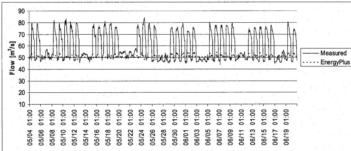
Figure 6.14: Revised Airflow Rate Variation from May 4<sup>th</sup> to June 20<sup>th</sup>; Sector A
