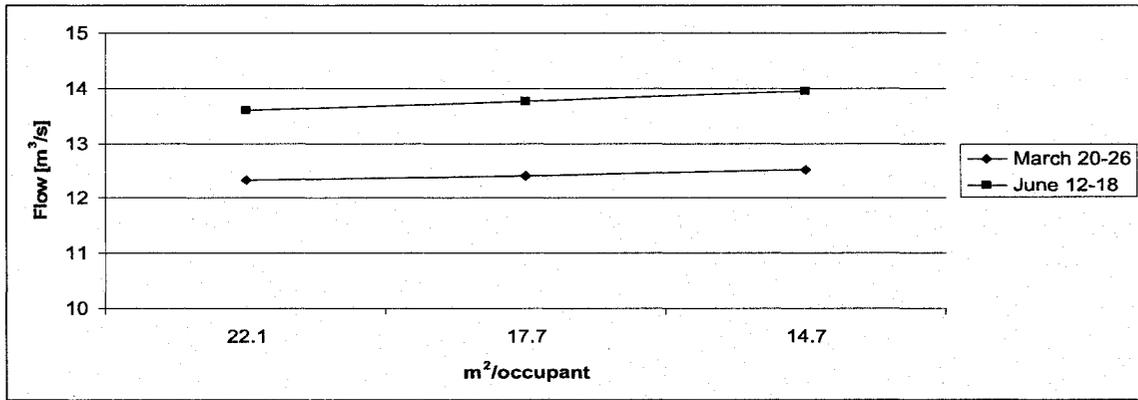
Figure 6.44: Variation of the Supply Airflow Rate with Occupancy Level; Sectors B & C
