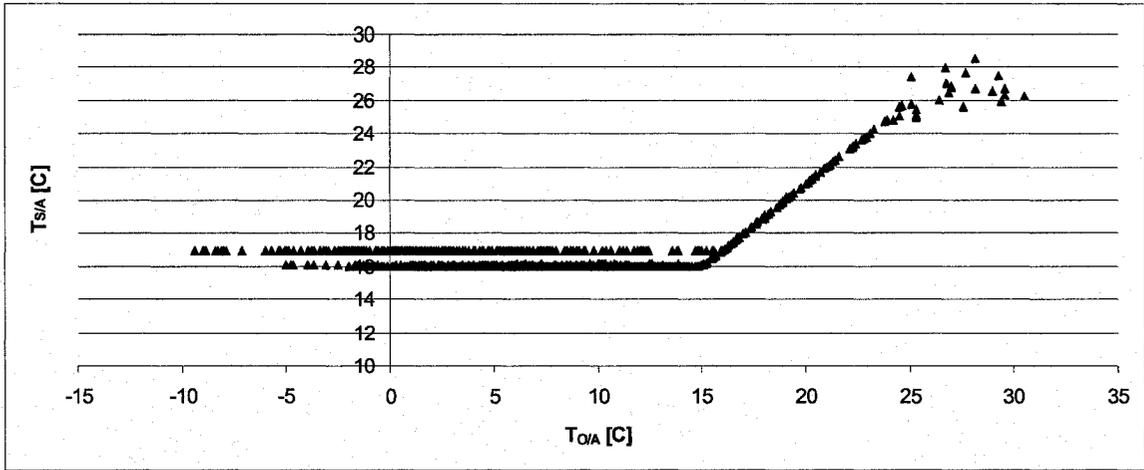
Figure 6.27: Revised Predicted Air Temperature versus Outdoor Air Temperature from March 20<sup>th</sup> to May 3<sup>rd</sup>; Sectors B & C
