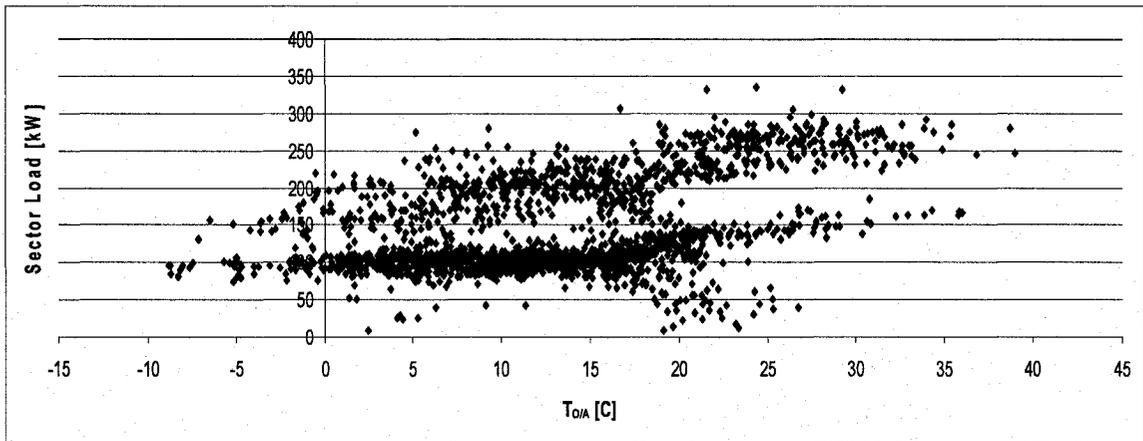
Figure 5.8: Sector Cooling Load versus Outdoor Air Temperature for the Spring Season; Sectors B and C
