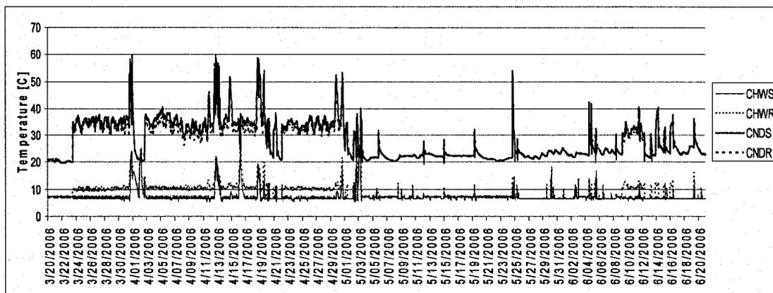
Figure 5.11: Water Temperatures at Chiller CH-4 over the Spring Season
