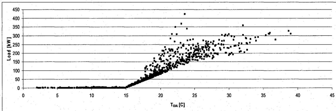
Figure 6.10: Estimated Cooling Coil Load versus Outdoor Air Temperature from May 4<sup>th</sup> to June 20<sup>th</sup>; Sectors B & C
