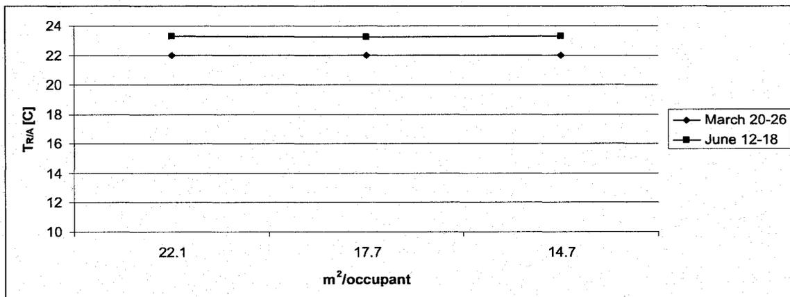
Figure 6.45: Variation of the Return Air Temperature with Occupancy Level; Sectors B & C
