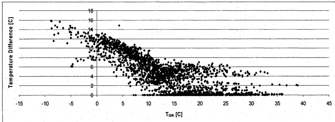
Figure 5.22: Glycol Temperature Difference versus Outdoor Air Temperature over the Spring Season; Sector A
