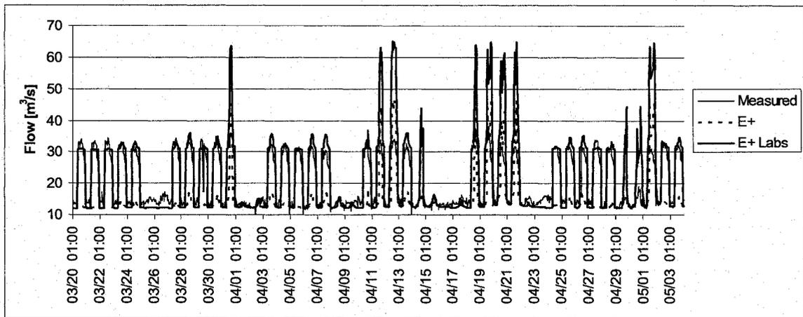
Figure 6.24: Revised Airflow Rate Variation from March 20<sup>th</sup> to May 3<sup>rd</sup>; Sectors B & C
