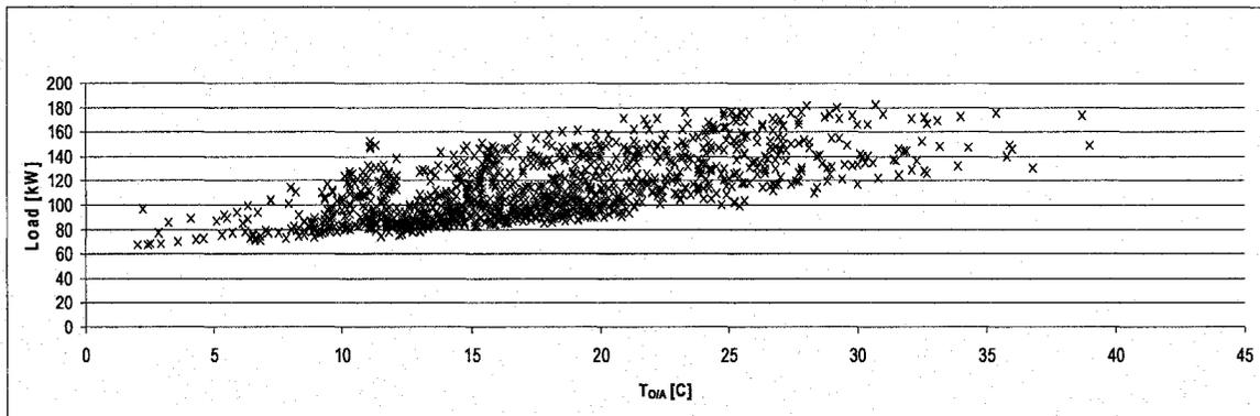
Figure 6.9: Estimated Zone Thermal Load of all Zones versus Outdoor Air Temperature from May 4<sup>th</sup> to June 20<sup>th</sup>; Sectors B & C
