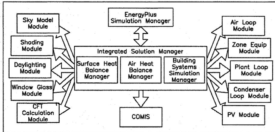
Figure 3.2: Solution Manager for the Heat Balance Method in EnergyPlus [28]
