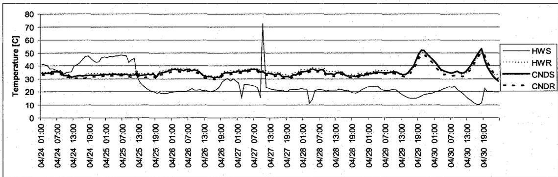
Figure 5.30: HW and CND Water Temperature Variation for the Week of April 24<sup>th</sup> to April 30<sup>th</sup>
