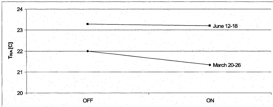
Figure 6.40: Variation of the Return Air Temperature without and with Air Infiltration; Sectors B & C
