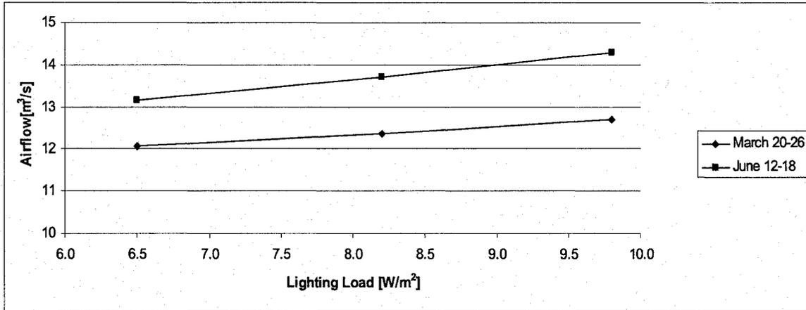
Figure 6.41: Variation of the Supply Airflow Rate with Lighting Load; Sectors B & C
