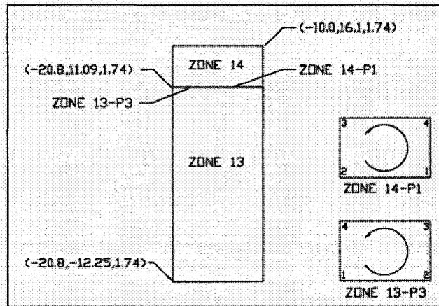
Figure 4.3: Definition of the Partition Wall between two Adjacent Zones
