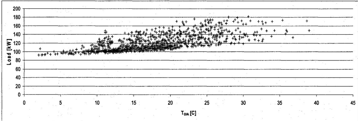
Figure 6.8: Estimated Sector Air-Side Thermal Load versus Outdoor Air Temperature from May 4<sup>th</sup> to June 20<sup>th</sup>; Sectors B & C
