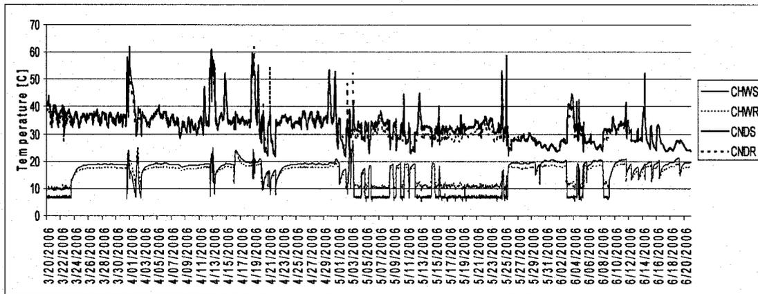
Figure 5.10: Water Temperatures at Chiller CH-3 over the Spring Season
