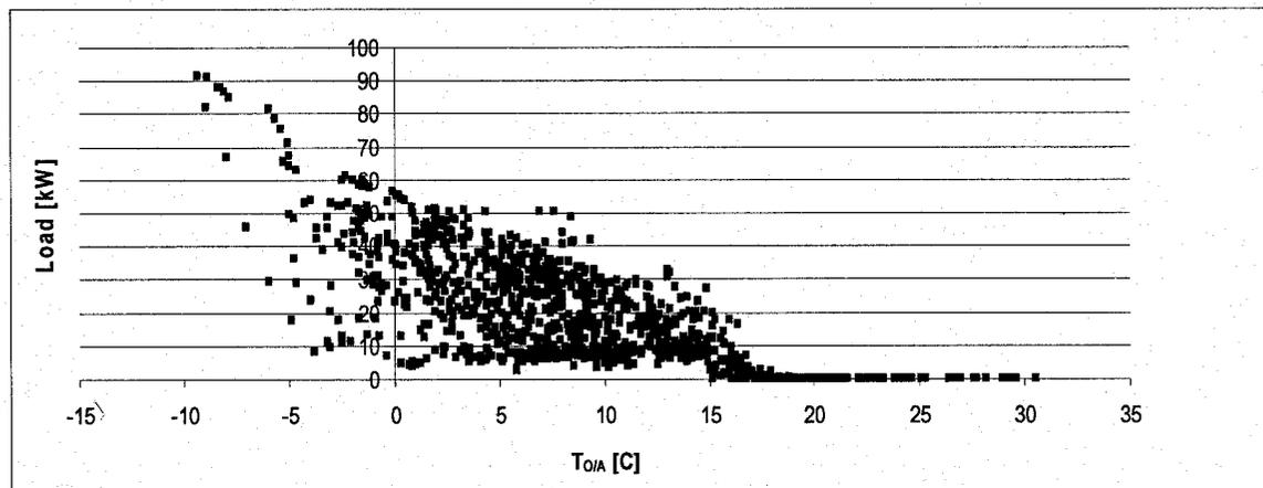
Figure 6.30: Estimated Re-heat and Heating Coils Load versus Outdoor Air Temperature from March 20<sup>th</sup> to May 3<sup>rd</sup>; Sectors B & C
