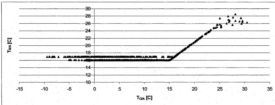
Figure 6.33: Supply Air Temperature versus Outdoor Air Temperature from March 20<sup>th</sup> to May 3<sup>rd</sup>; Sector A
