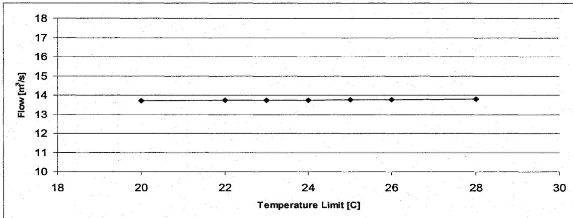
Figure 6.47: Variation of the Supply Airflow Rate with Economizer Cut-Off Temperature; Sectors B & C
