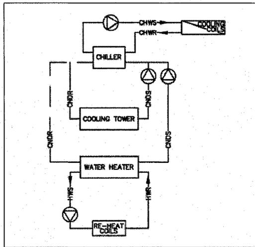
Figure 4.13: Cooling and Reheat Simulation Schematic
