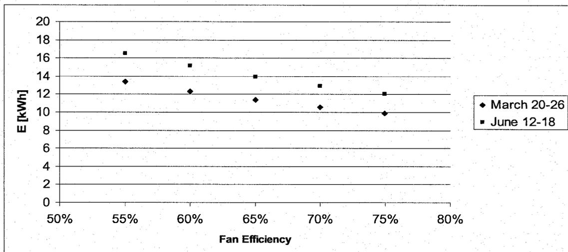
Figure 6.49: Variation of the Supply Fan Electricity Consumption with Fan Efficiency; Sectors B & C
