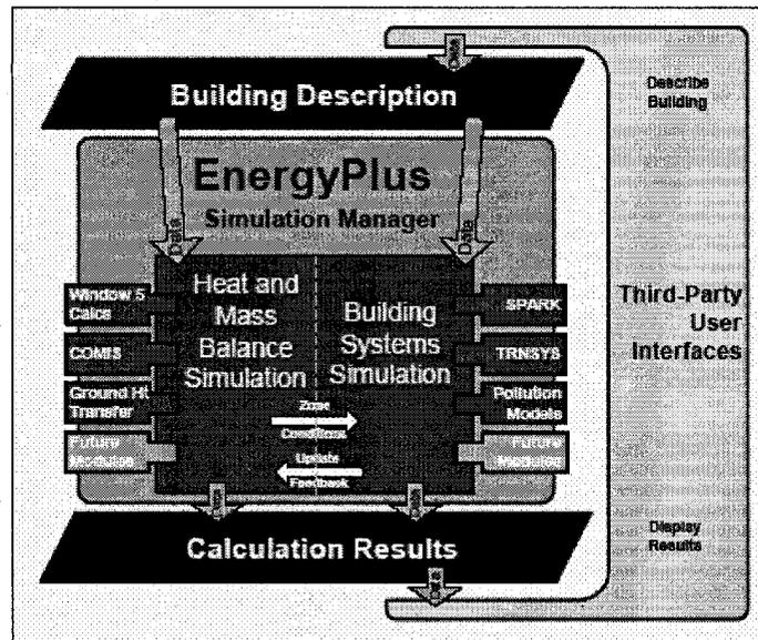
Figure 3.1: Overall Structure of EnergyPlus [23]
