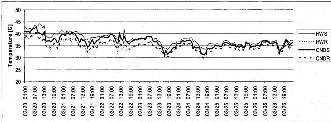
Figure 5.25: HW and CND Water Temperature Variation for the Week of March 20<sup>th</sup> to March 26<sup>th</sup>
