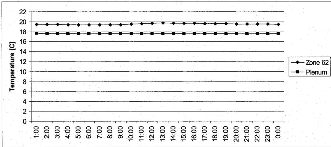
Figure 4.7: Direct Exhaust Plenum and Zone Temperature Variation during the Winter Design Day
