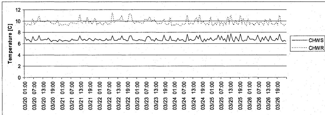
Figure 5.26: Chilled Water Temperature Variation for the Week of March 20<sup>th</sup> to March 26<sup>th</sup>
