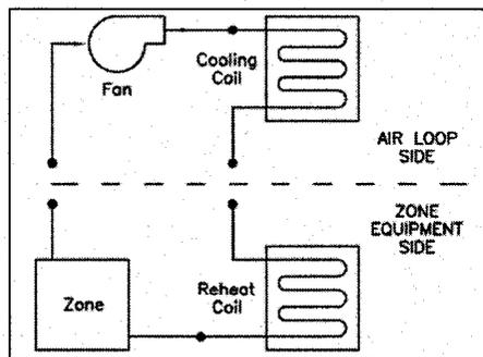
Figure 3.3: Example of Air Loop Schematic [30]
