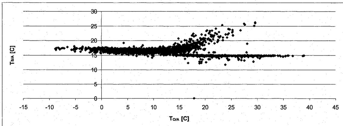
Figure 5.7: Hourly Values of Supply Air Temperature versus Outdoor Air Temperature for the Spring Season; Sector A
