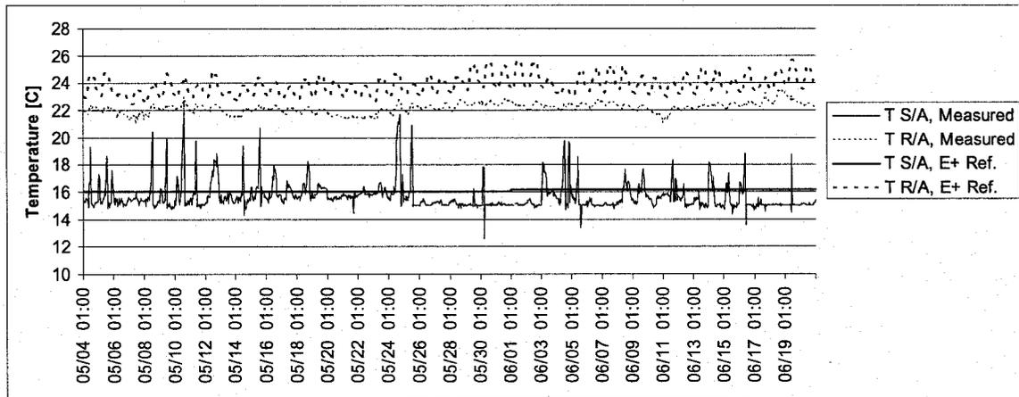
Figure 6.3: Air Temperature Variation from May 4<sup>th</sup> to June 20<sup>th</sup>; Sectors B & C
