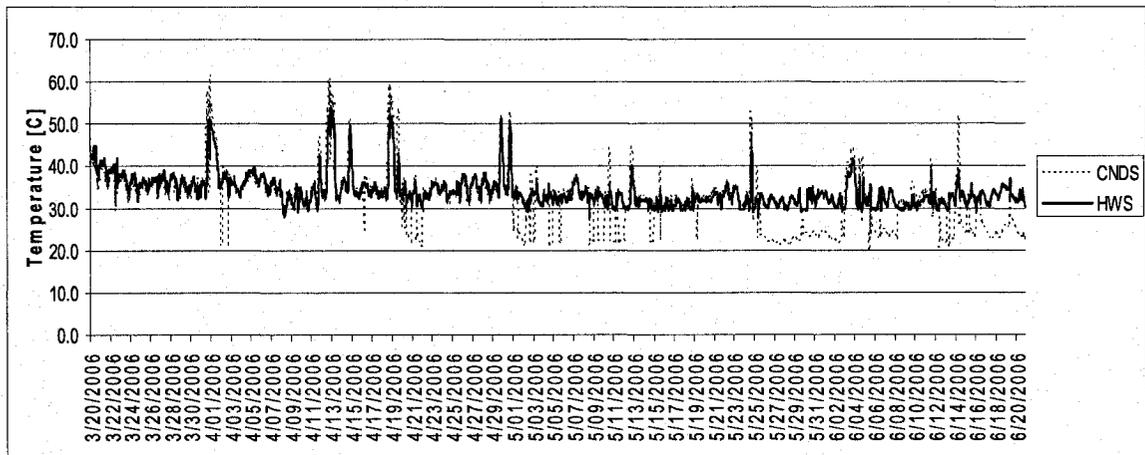
Figure 5.16: Water Temperature of CNDS and HWS over the Spring Season
