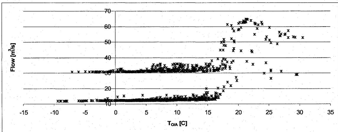
Figure 6.26: Revised Predicted Airflow Rate versus Outdoor Air Temperature from March 20<sup>th</sup> to May 3<sup>rd</sup>; Sectors B & C
