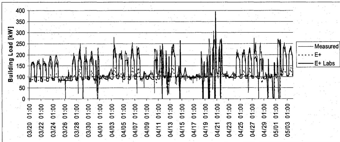
Figure 6.28: Sector Air-Side Thermal Load from March 20<sup>th</sup> to May 3<sup>rd</sup>; Sectors B & C
