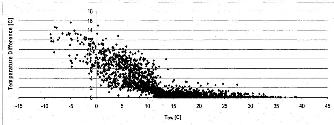
Figure 5.21: Glycol Temperature Difference versus Outdoor Air Temperature over the Spring Season; Sectors B and C
