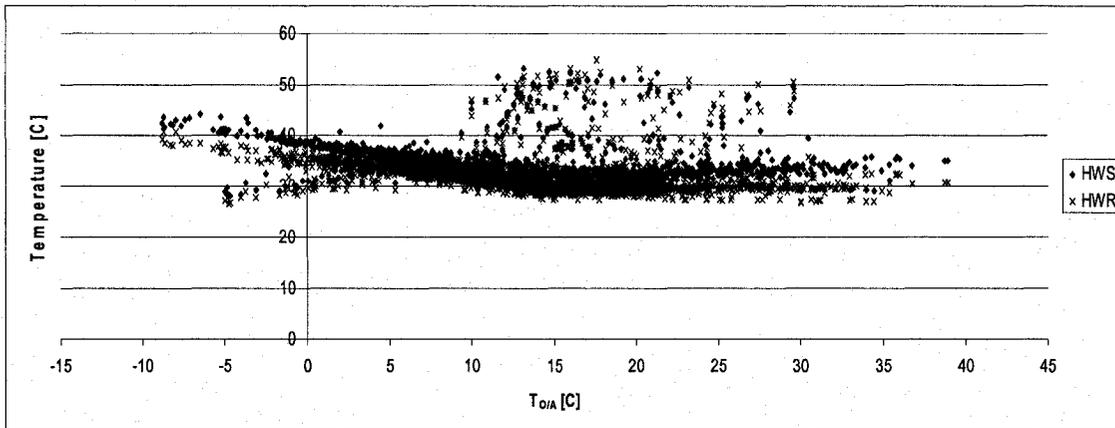
Figure 5.17: Heating Water Temperature versus Outdoor Air Temperature over the Spring Season
