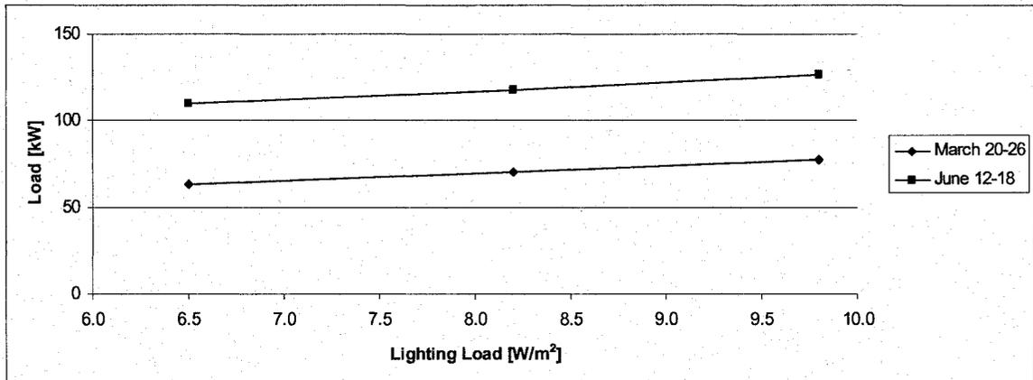
Figure 6.42: Variation of the Cooling Air-Side Thermal Load with Lighting Load; Sectors B & C
