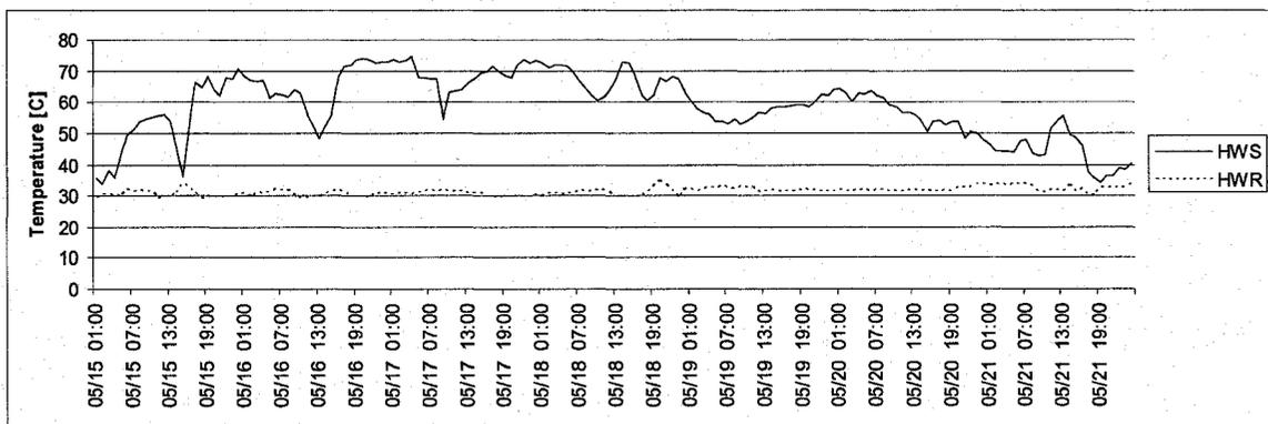
Figure 5.35: Water Temperature Variation for the Week of May 15<sup>th</sup> to May 21<sup>st</sup>
