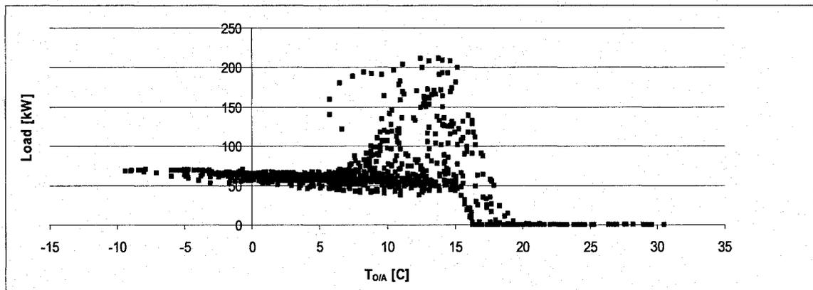
Figure 6.36: Estimated Re-heat and Heating Coils Load versus Outdoor Air Temperature from March 20<sup>th</sup> to May 3<sup>rd</sup>; Sector A
