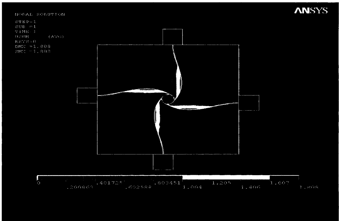
Figure 3.18: Vector Summation of displacement for Model (2c) in ANSYS, under the application of 16.5V or 3.9309 mA
