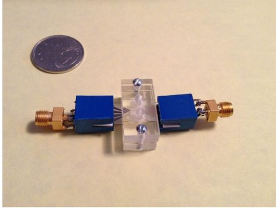
**Figure 7.7: A picture of the second device with the 2 SMA high frequency connectors**
