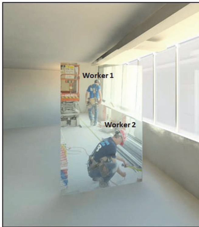
Figure 4-11 Augmenting the BIM Model with Video of Workers and Their IDs
