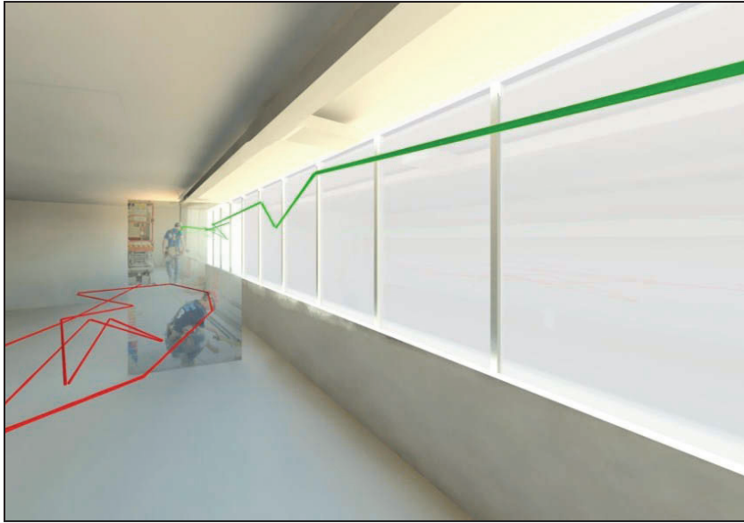
Figure 4-10 Augmenting the BIM Model with Picture of Workers and the Traces of Their Movement
