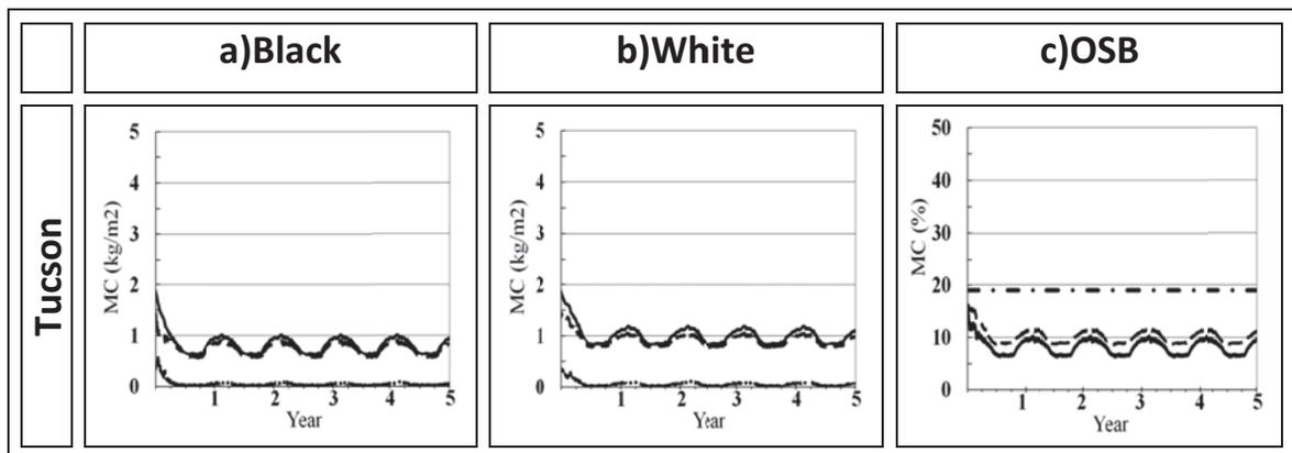
Figure 5-9. Moisture content of typical roofs for residential buildings in Tucson. Column a, b shows black and white roofs moisture contents ( $\text{kg/m}^2$ ): total (—), OSB (■ ■ ■), Mineral Wool (■ ◆ ◆ ■). Column c shows OSB moisture content (%): white roof (■ ■ ■), black roof (—), max allowable MC (19%) (■ ◆ ■)
