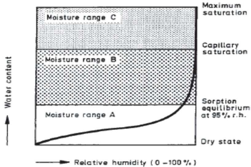
Figure 3-2. Schematic diagram of the moisture storage functions of a porous building material (Künzel, 1995)
