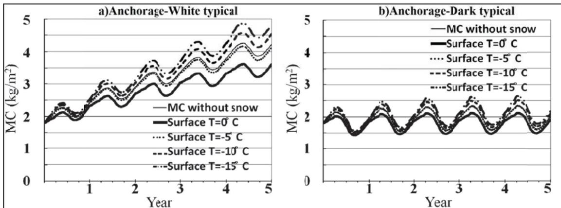
Figure 5-8. Sensitivity analysis on total moisture content of dark and white typical roofs in Anchorage
