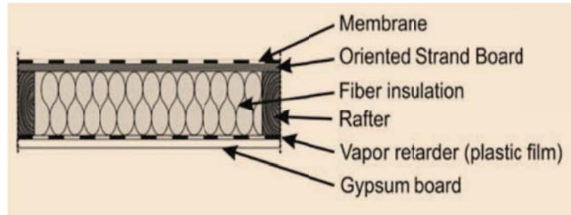
Figure 2-4. Typical European flat roof composition (Bludau, et al., 2008)
