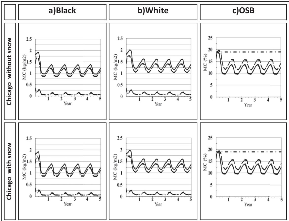
Figure 5-14. Effect of snow on the moisture content of residential building with smart roof composition; Column a, b shows black and white roofs moisture content (kg/m<sup>2</sup>): total (—), OSB (■ ■ ■), Mineral Wool (■ ● ■). Column c shows OSB moisture content (%): white roofs (■ ■ ■), black roofs (—), max allowable MC (19%) (■ ● ■)
