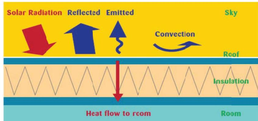
Figure 2-2. Heat transfer through a roof (Cool Roof Design Brief, 2006)
