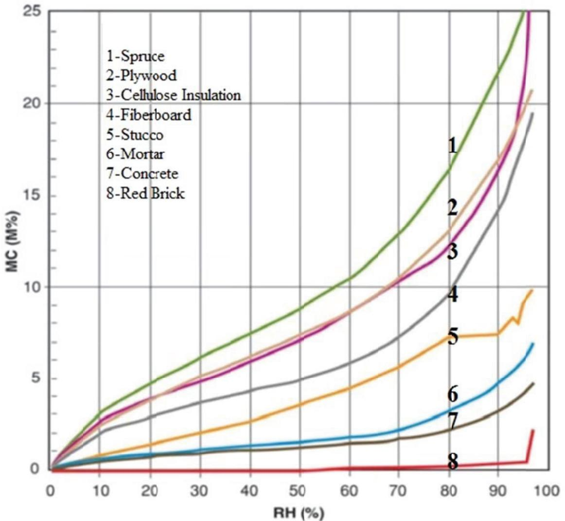
Figure 3-4. Moisture isotherms for different building material (Straube, 2006)
