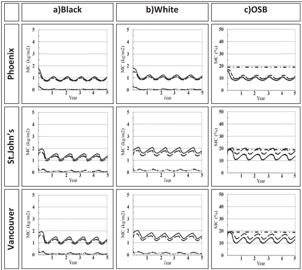
Figure 5-13. Moisture content of smart roofs for residential buildings. Column a, b shows black and white roofs moisture content ( $\text{kg/m}^2$ ): total (—), OSB (---), Mineral Wool (····). Column c shows OSB moisture content (%): white roof (---), black roof (—), max allowable MC (19%) (····)
