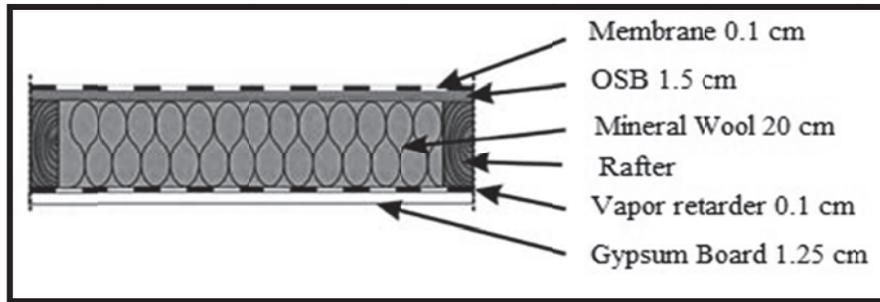
Figure 5-5. Simulated roofing composition for validation of a steady state condition
