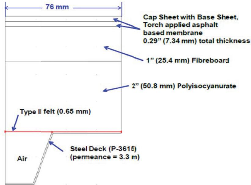
Figure 2-6.A schematic of Modified-Bitumen roofing system (Saber, et al., 2011)
