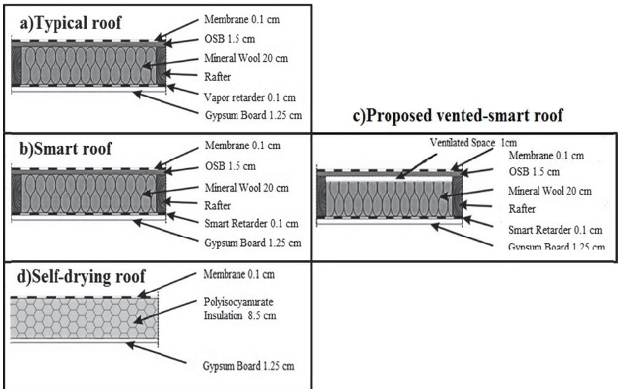
Figure 5-1. Simulated roofing compositions (Bludau, et al., 2008)
