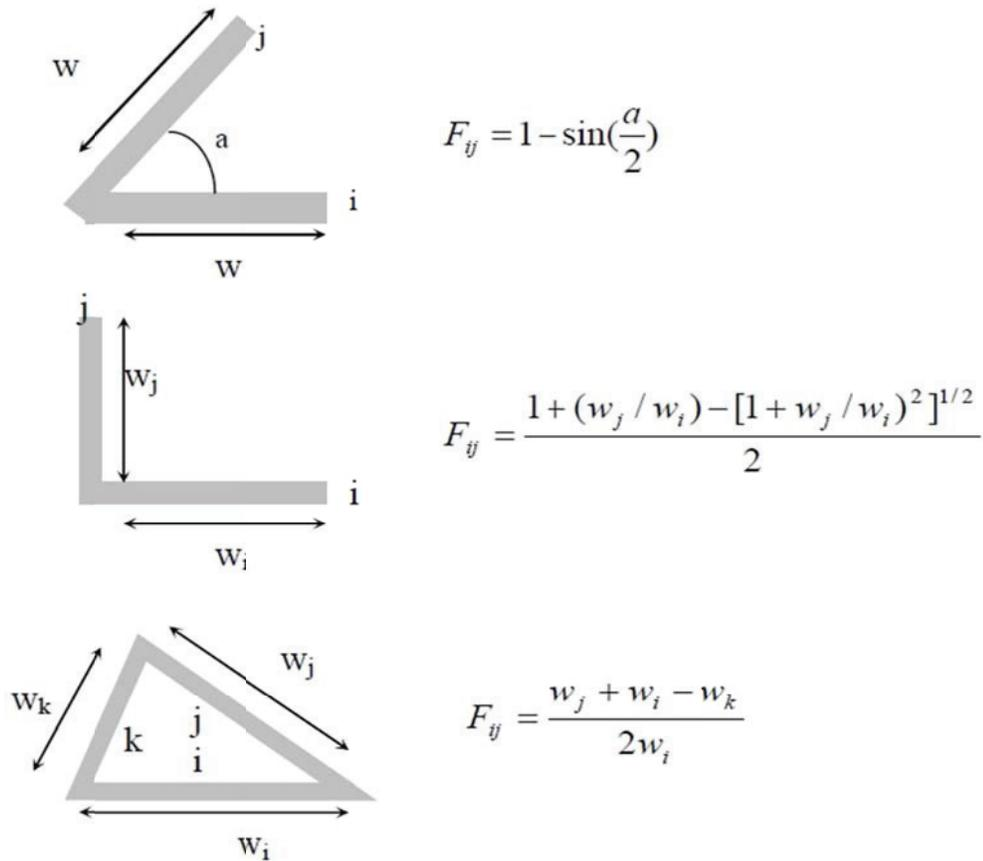
Figure 3-1. View factors for common situations in building enclosures (Hangentoft, 2001)
