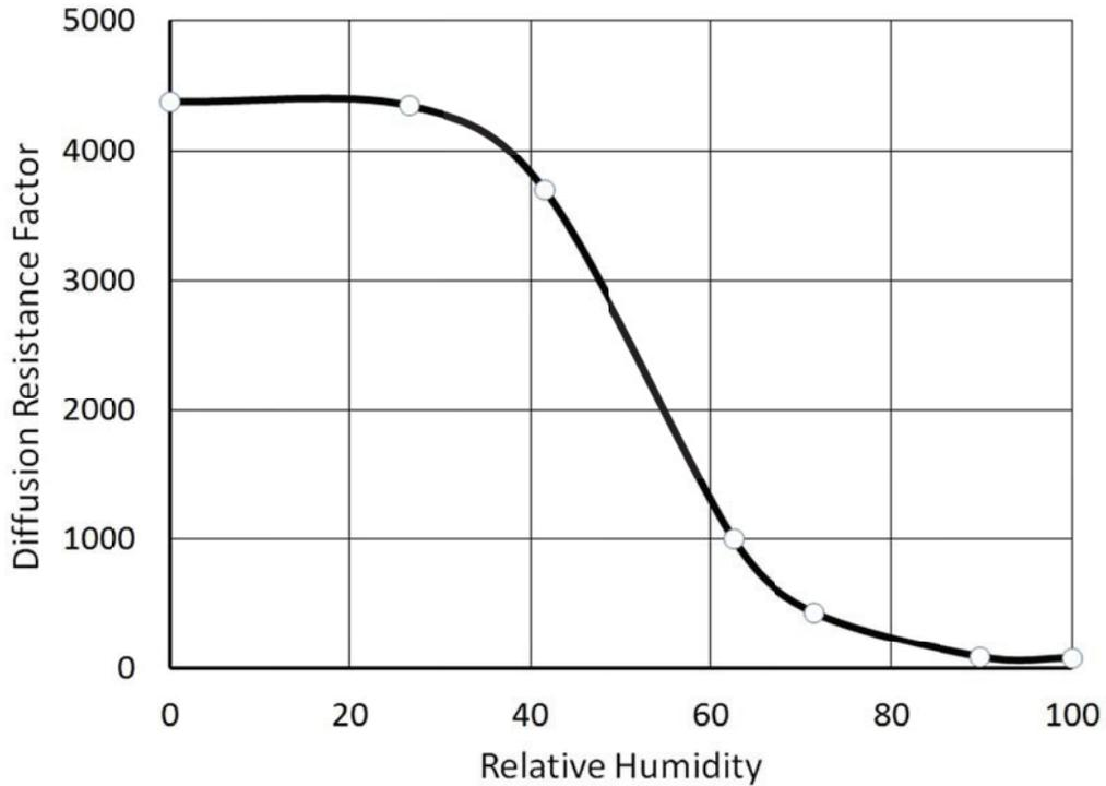
Figure 5-2. Diffusion resistance factor dependency of smart vapor retarder (PA-film) to Relative Humidity (originated from WUFI database)
