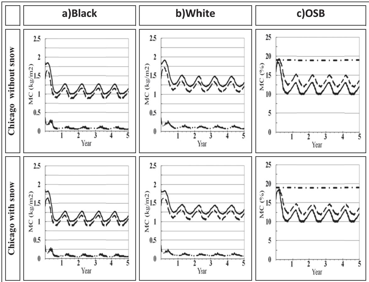
Figure 5-11. Effect of snow on the moisture content of office building with typical roof composition; Column a, b shows black and white roofs moisture content ( $\text{kg}/\text{m}^2$ ): total (—), OSB (■ ■ ■), Mineral Wool (■ ◆ ◆ ■). Column c shows OSB moisture content (%): white roofs (■ ■ ■), black roofs (—), max allowable MC (19%) (■ ◆ ◆ ■)
