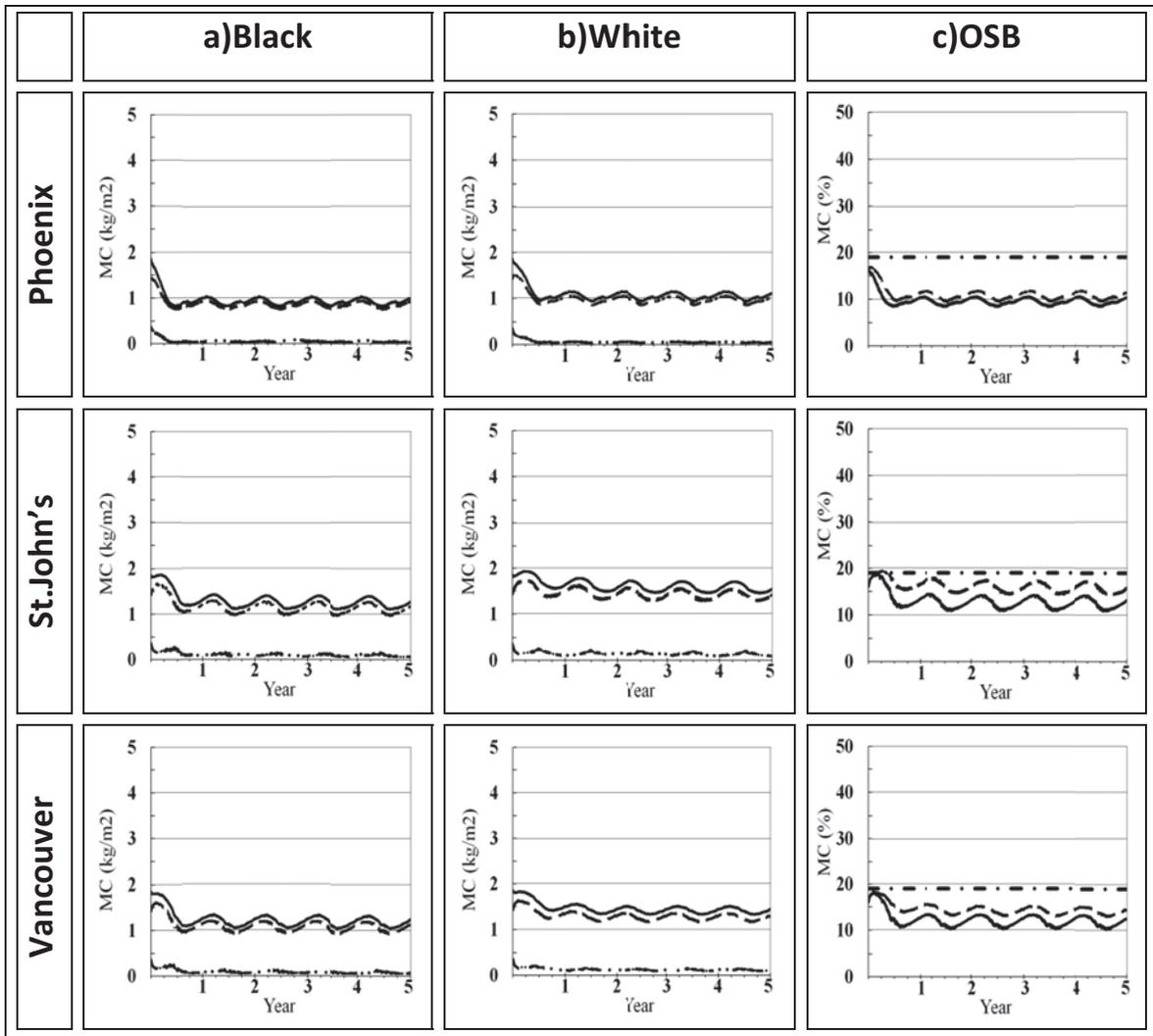
Figure 5-10. Moisture content of typical roofs for office buildings .Column a, b shows black and white roofs moisture content ( $\text{kg/m}^2$ ): total (—), OSB (---), Mineral Wool (-·-·-).Column c shows OSB moisture content (%): white roofs (---), black roofs (—), max allowable MC (19%) (-·-·-)
