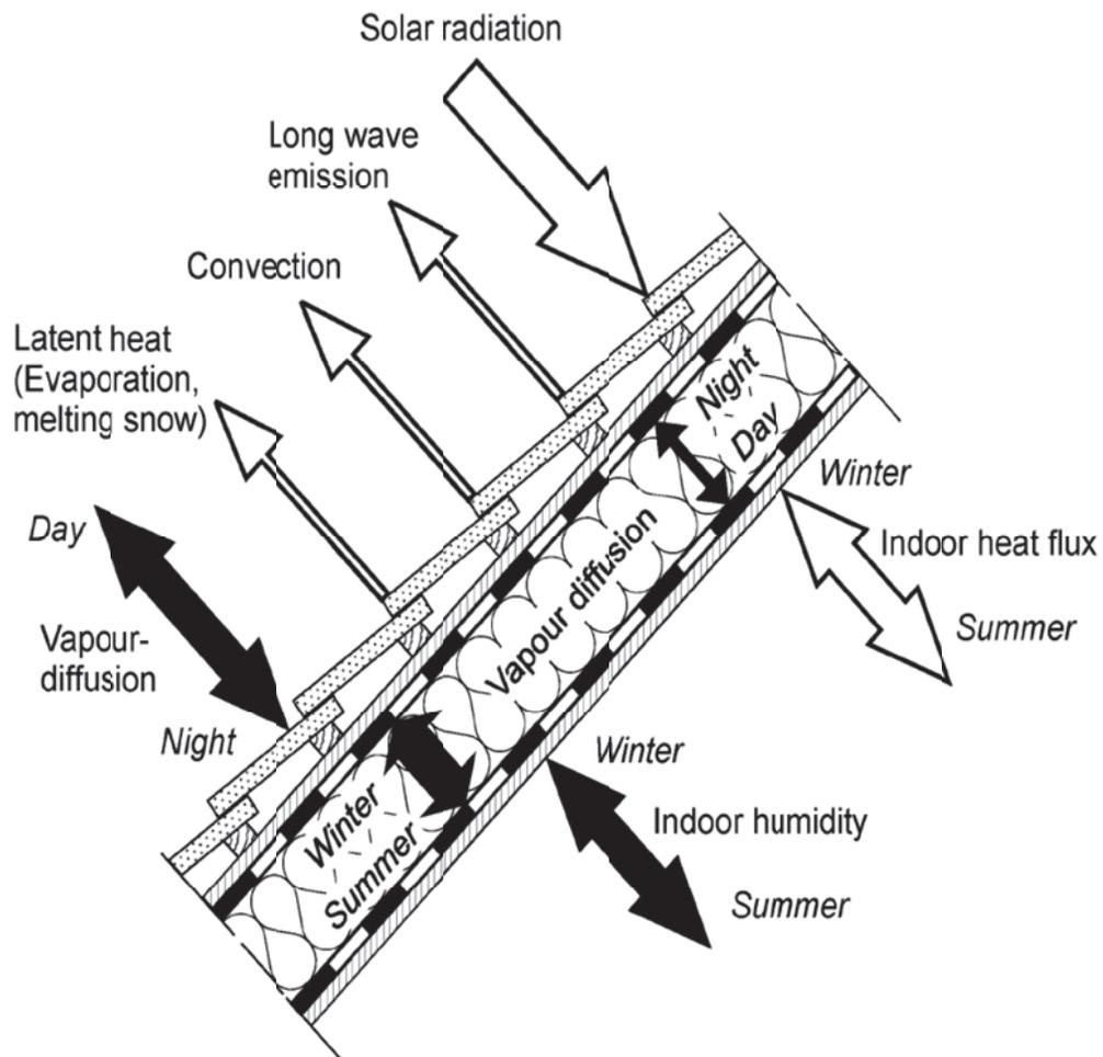
Figure 4-1. Indoor and outdoor hygrothermal loads and fluxes in a sloped roof (Künzel, 2000)
