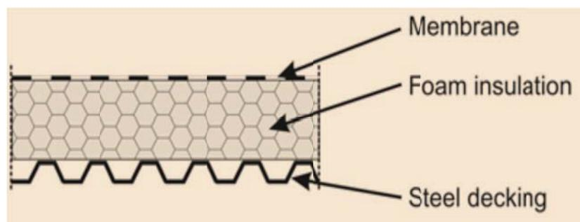
Figure 2-3. Self-drying roof composition (Bludau, et al., 2008)
