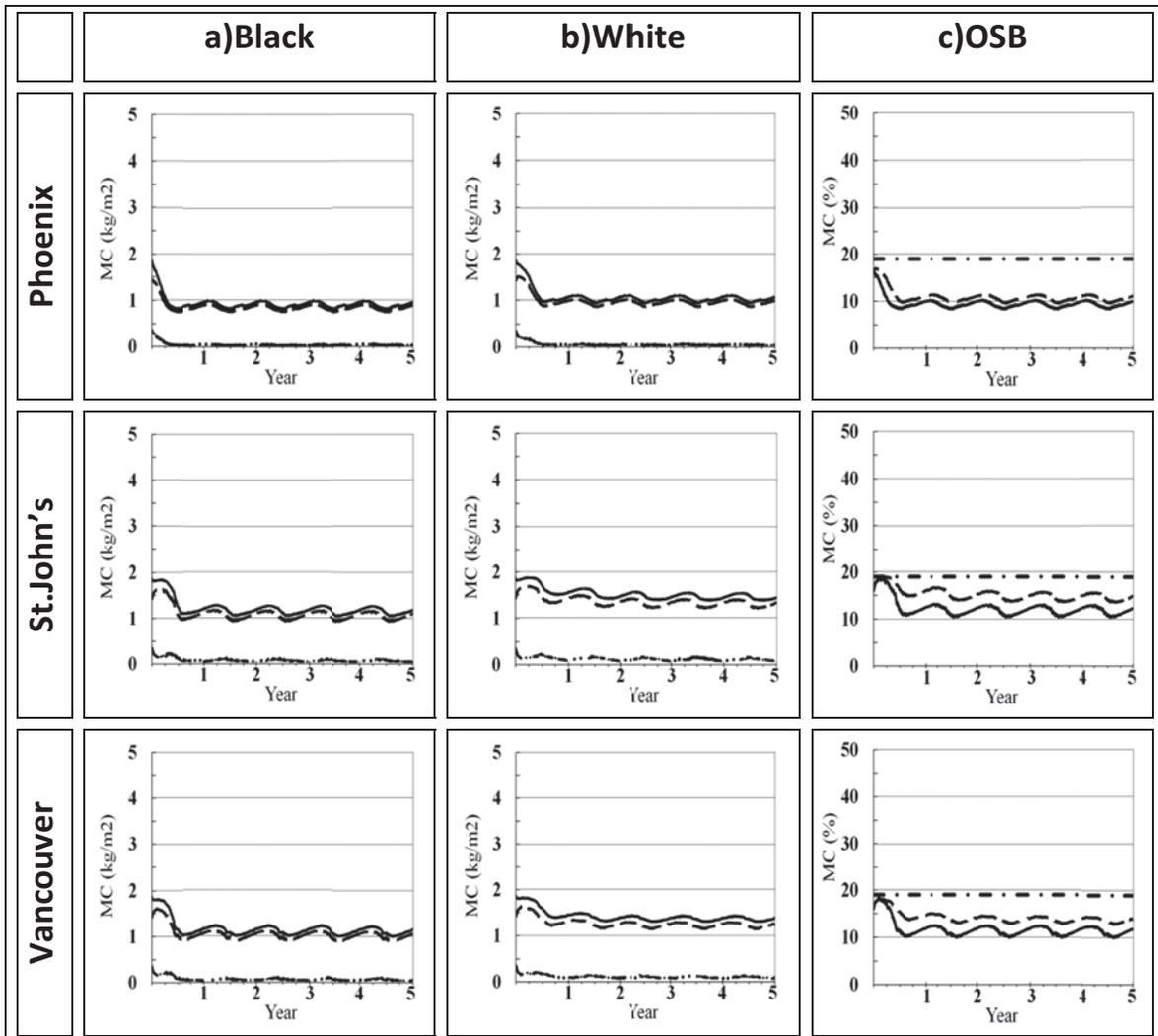
Figure 5-15. Moisture content of smart roofs for office buildings. Column a, b shows black and white roofs moisture content ( $\text{kg/m}^2$ ): total (—), OSB (---), Mineral Wool (····). Column c shows OSB moisture content (%): white roof (---), black roof (—), max allowable MC (19%) (---)
