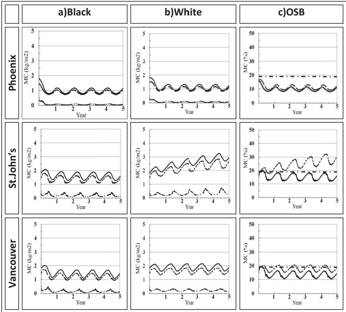
Figure 5-6. Calculated moisture content of typical roofs for residential buildings .Column a, b shows black and white roofs moisture contents ( $\text{kg/m}^2$ ): total (—), OSB (---), Mineral Wool (· · ·).Column c shows OSB moisture content (%): white roof (---), black roof (—), max allowable MC (19%) (· · ·)
