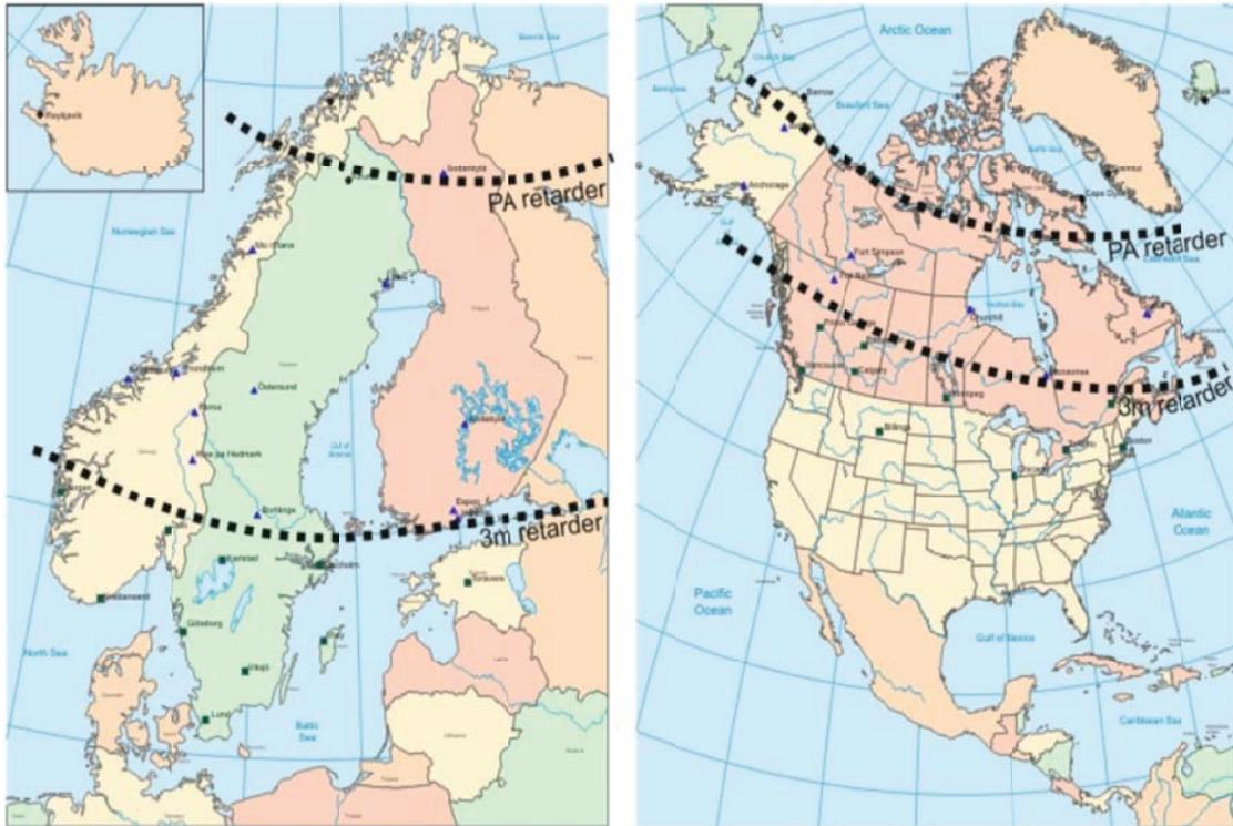
Figure 2-5. Limit curves for the two different vapour retarders in Scandinavia and North America (Bludau & Kunzel, 2009)
