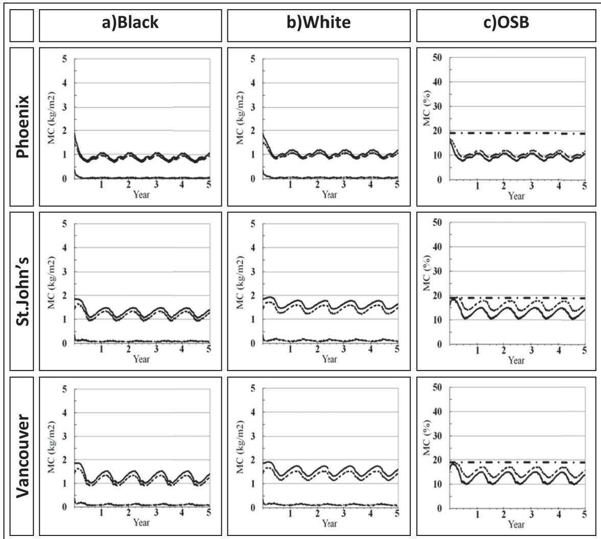
Figure 5-17. Moisture content of vented smart roofs for residential buildings. Column a, b shows black and white roofs moisture content ( $\text{kg}/\text{m}^2$ ): total (—), OSB (■ ■ ■), Mineral Wool (■ ◆ ◆ ■). Column c shows OSB moisture content (%): white roof (■ ■ ■), black roof (—), max allowable MC (19%) (■ ◆ ◆ ■)
