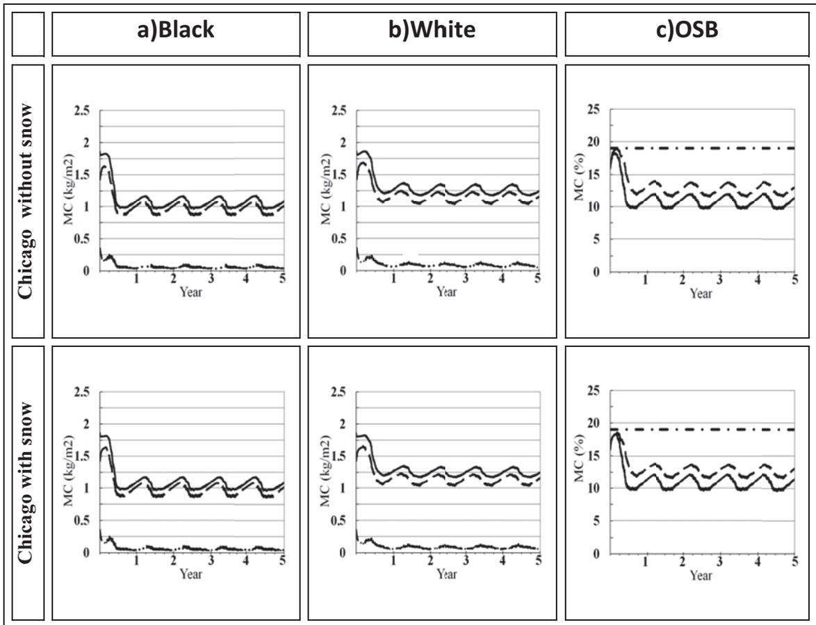
Figure 5-16. Effect of snow on the moisture content of office building with smart roof composition; Column a, b shows black and white roofs moisture content ( $\text{kg}/\text{m}^2$ ): total (—), OSB (■ ■ ■), Mineral Wool (■ ♦ ■). Column c shows OSB moisture content (%): white roofs (■ ■ ■), black roofs (—), max allowable MC (19%) (■ ♦ ■)
