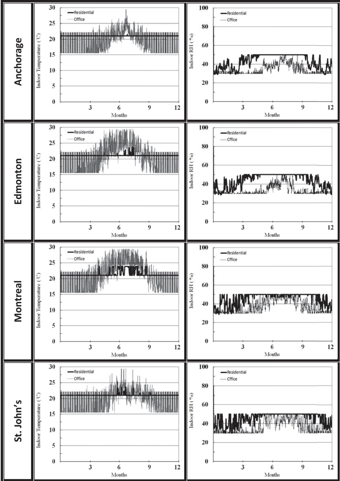
Figure 5-12. Indoor T, RH for residential and office buildings with typical composition roof
