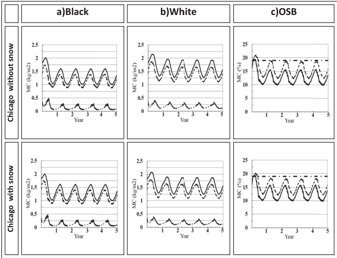
Figure 5-7. Effect of snow on moisture content residential building with typical roof composition; Column a, b shows black and white roofs moisture content ( $\text{kg/m}^2$ ): total (—), OSB (■ ■ ■), Mineral Wool (■ ● ■). Column c shows OSB moisture content (%): white roof (■ ■ ■), black roof (—), max allowable MC (19%) (■ ● ■)
