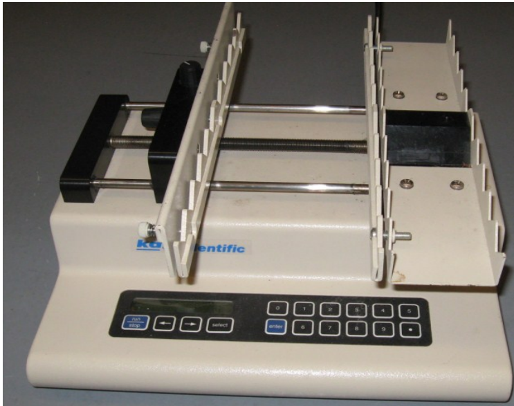
Figure 3.7 Syringe sampler from KD Scientific (model no. 230)
