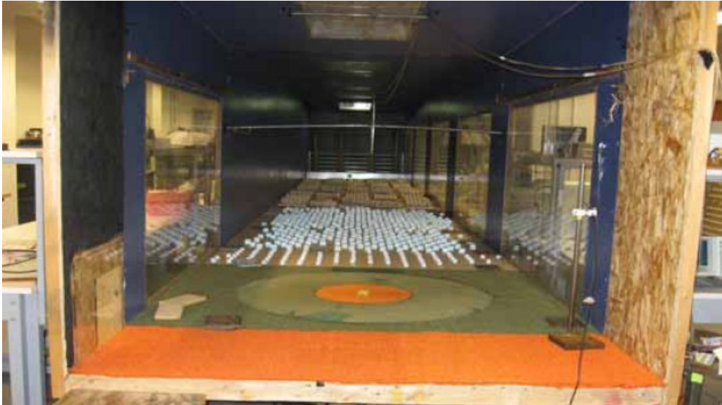
Figure 3.3 Front view section of the Boundary Layer Wind tunnel at Concordia University (from Stathopoulos et al., 2008).
