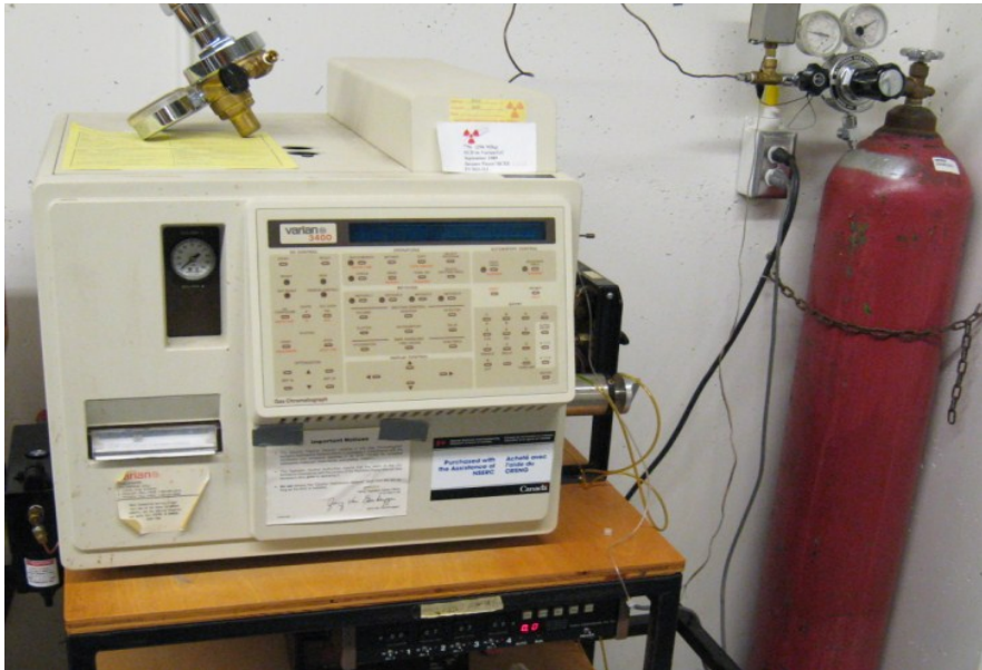
Figure 3.8 Gas chromatograph used for measuring concentration of tracer
