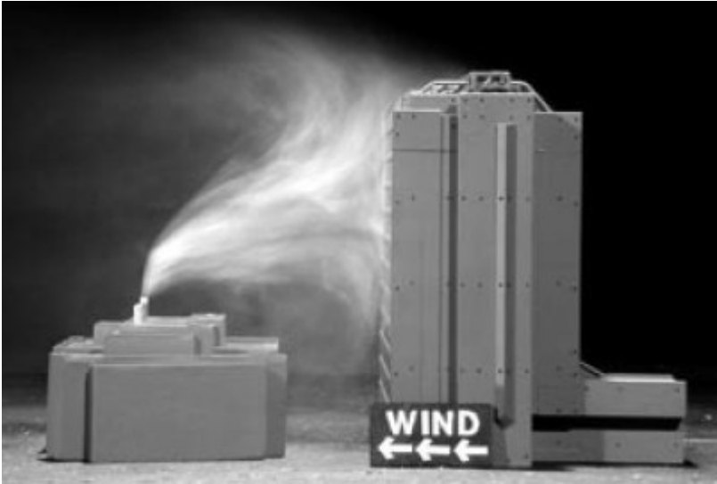
Figure 3.10 Recirculation zone in the wake of a building (from: http://www.epa.gov )
