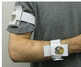
Figure 1.1: Intel "SHIMMER" sensors being worn on a patient's arm [8]
