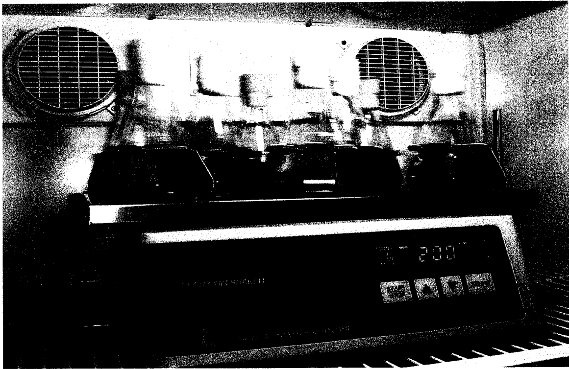
Figure 3.2: Test flasks on INNOVA orbital shaker
