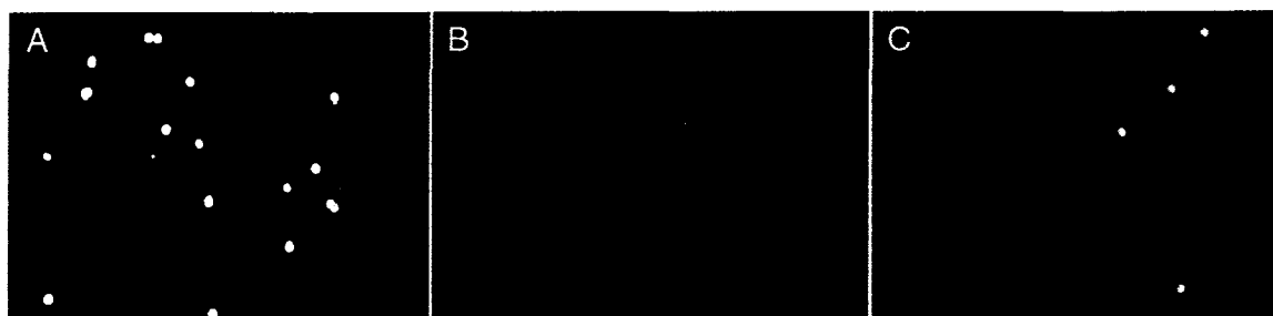
Figure 5.8 Fluorescent images of 8 \mu\text{m} particles in initial solution (A) after filtration with filled capillary (B) or by sedimentation using the “snorkel effect”(C). All images used the same magnification.
