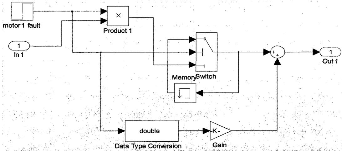
**Figure 6. 4 Simulink block for stuck at current position**
