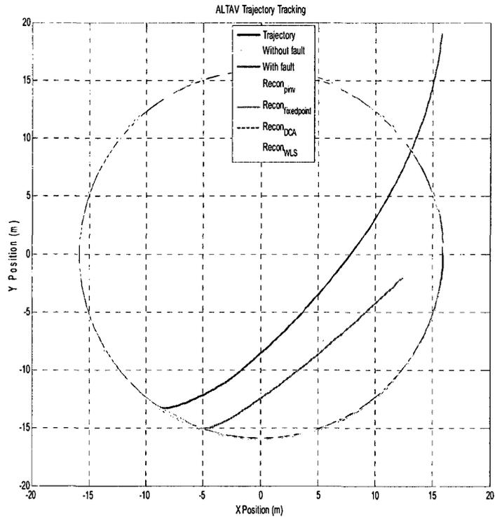
**Figure 7.32 UAV virtual and reallocation tracking trajectory**
