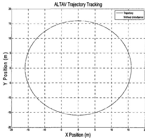
**Figure 7. 6 The circle virtual trajectory vs the desired trajectory**
