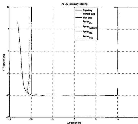
**Figure 7.2 Virtual and actual trajectory diagram (no Gaussian noise)**
