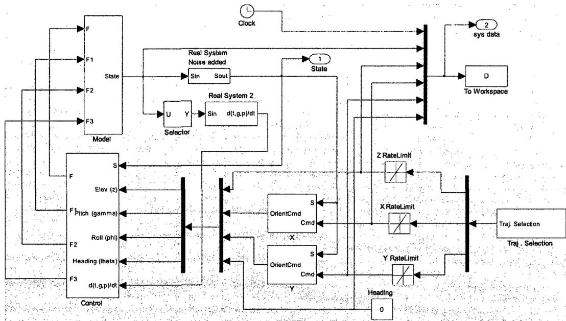
**Figure 4. 2 Simulink block diagram of the ALTAV**
