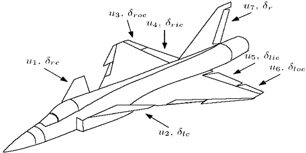
**Figure 5. 1 ADMIRE control surface configurations**
