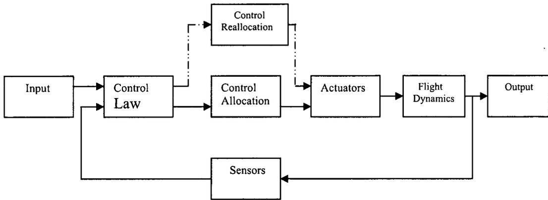
**Figure 1. 1 Simple structure of fault tolerant control system**
