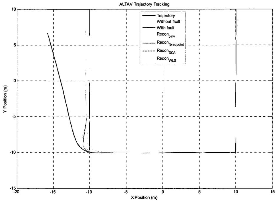
**Figure 7.8 UAV virtual and reallocation tracking trajectories**
