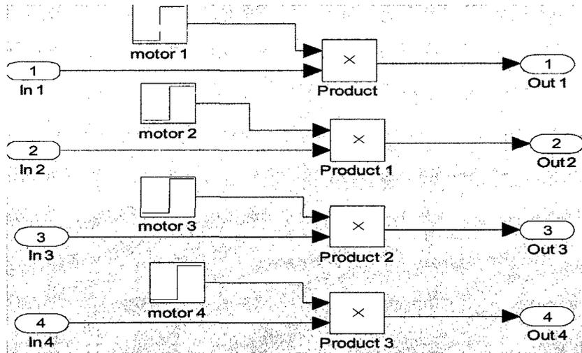
**Figure 6. 3 ALTAV Simulink block of partial loss implementation**
