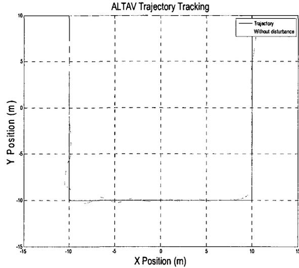
**Figure 7. 5 The square virtual trajectory vs the desired trajectory**
