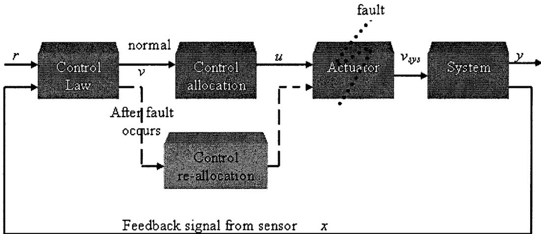
**Figure 2. 2 Control re-allocation block diagram**
