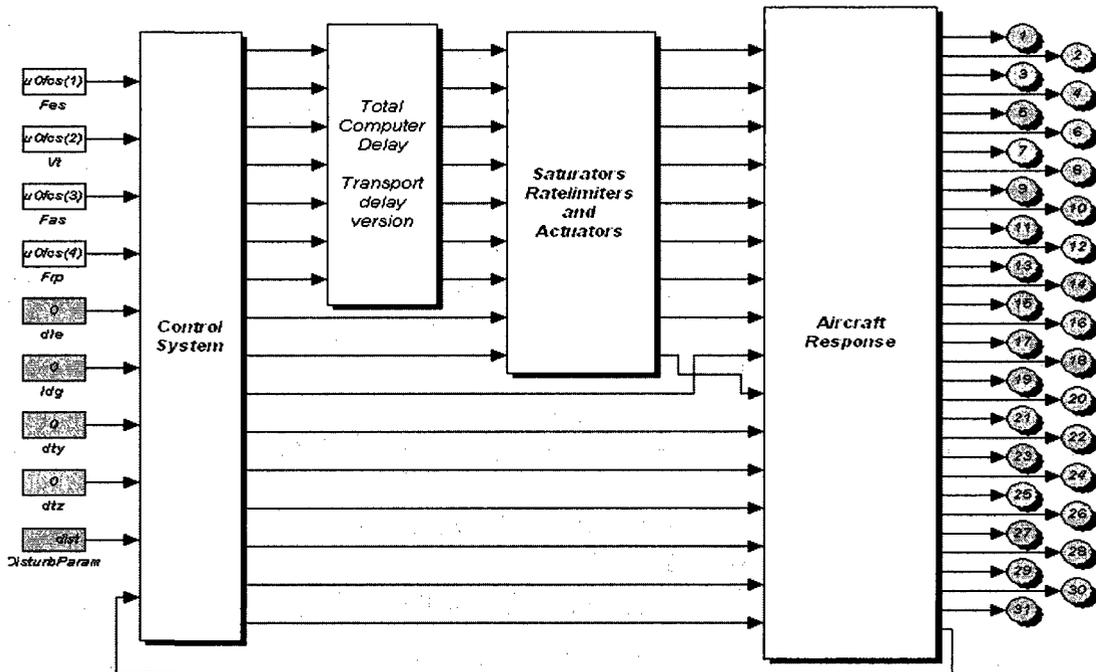
Figure 5. 2 Simulink block diagram of the ADMIRE
