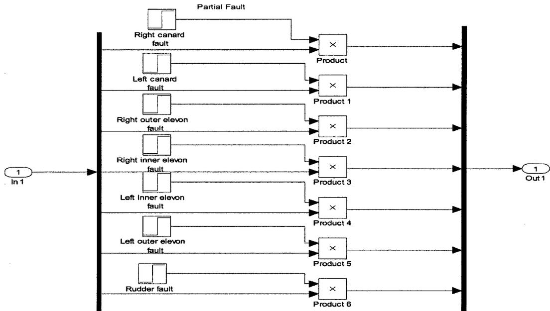
**Figure 6. 9 ADMIRE Simulink block of partial loss implementation**
