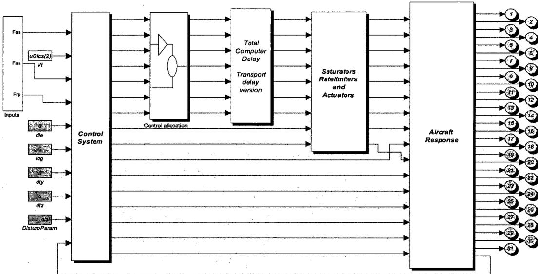
**Figure 6. 8 ADMIRE Simulink with control reallocation block**
