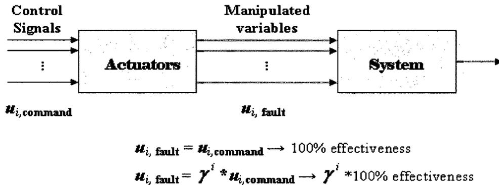
**Figure 2. 3 Actuator failures by control effectiveness factor**
