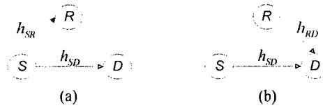
Figure 2.2: Protocol I: (a) the first time slot, (b) the second time slot.
