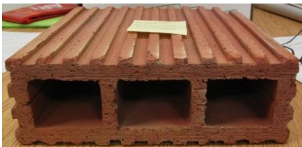
3.1.4 Produced in Pointe-Claire: fire proof terracotta building blocks (photo: Anja Borck).
