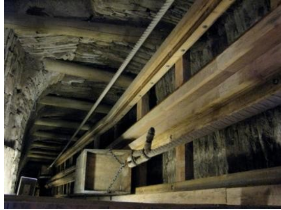
3.6.3.5 + 3.6.3.6 Reconstructed horse gin Rudolphschacht Lauta, near Marienberg, Saxony, used for the vertical transportation of loads inside the mine shaft. They were once a common feature at farms and in mining industries, in Germany all but one disappeared (photos: Anja Borck).
