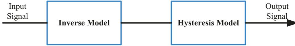
Figure 2.2: Inverse feedforward controller for hysteresis nonlinearity.
