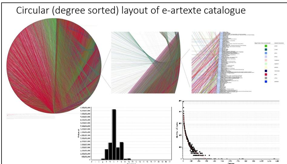
The graph shows the relationship between node degree and the number of nodes in the network. Networks have been found to have a 'scale-free property' when a power law relationship between node degree and the number of nodes in the network follows this type of
