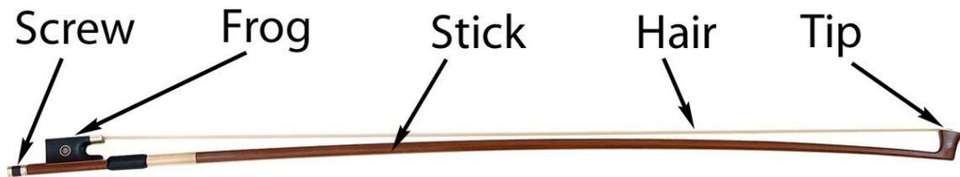
Figure 4.1 Parts of the violin bow.<sup>31</sup>
