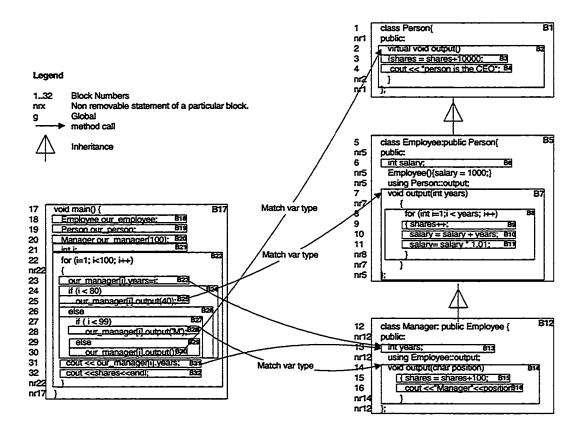
Figure 19: Function prototype matching
