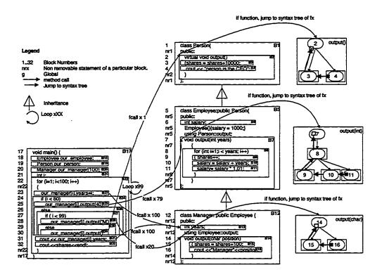
Figure 22: Criterion based hybrid program slicing
