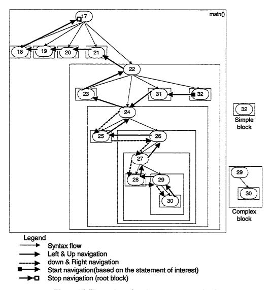
Figure 15: Illustration of static syntax tree navigation.
