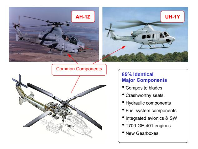
Figure 2.52 Bell AH-1Z & UH-1Y Systems & Components Commonality (Birkholz, 2001)
