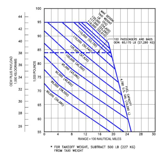
3.2.2 PAYLOAD/RANGE FOR LONG-RANGE CRUISE MODEL 737-200 (JT8D-9/9A ENGINES)
