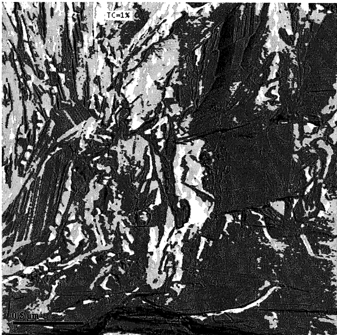
Figure 9.12 Microstructure of coating color with 1% of total charge of inhibitor.
