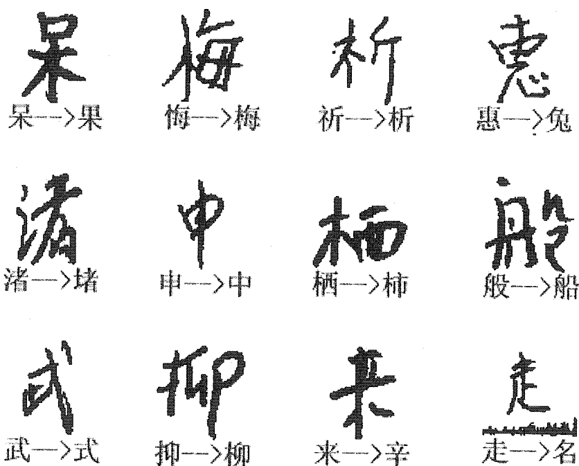
Figure 28: A part of misclassified patterns on ETL test set. The first character on the bottom specifies the original label. The second character is the recognized label.
