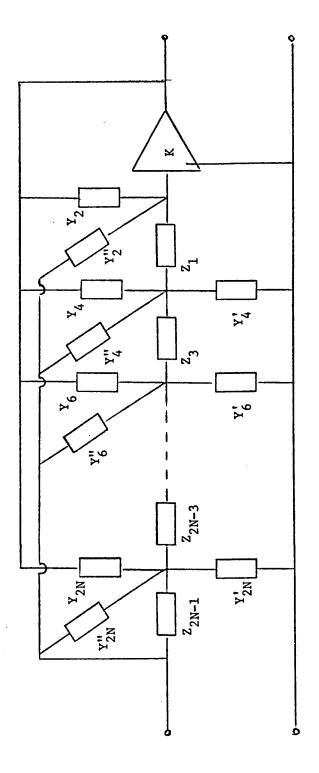
FIGURE 1.1 Multiple loop feedback network with feedforward constrained by an operational amplifier.
