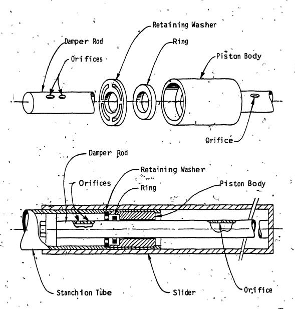
Fig. 2.5: Valving Mechanism of a 35 mm Betor Fork Leg
