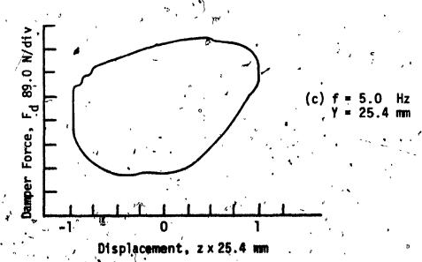
Fig. 3.9: Front Fork - Experimental Results
