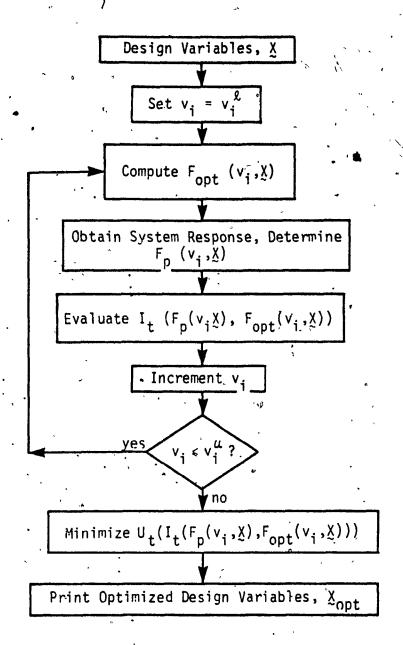
Fig. 6.2: Flowchart of the Optimization Procedure-Time Domain
