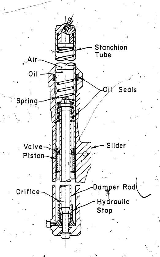
Fig. 2.2: Cross-Sectional View of a 38 mm Marzocchi Fork Leg
