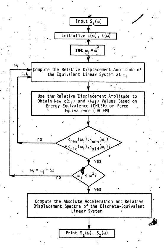
Fig. 7.9: Flowchart for the Discrete-Harmonic Linearization (DHL) Method
