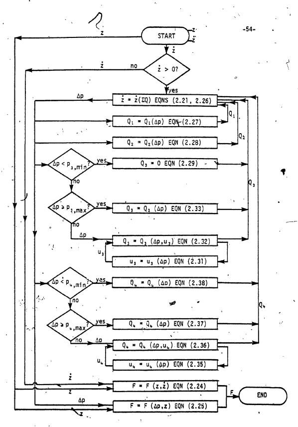
Fig. 3.4: Flowchart for the Rear Shock Absorber Model
