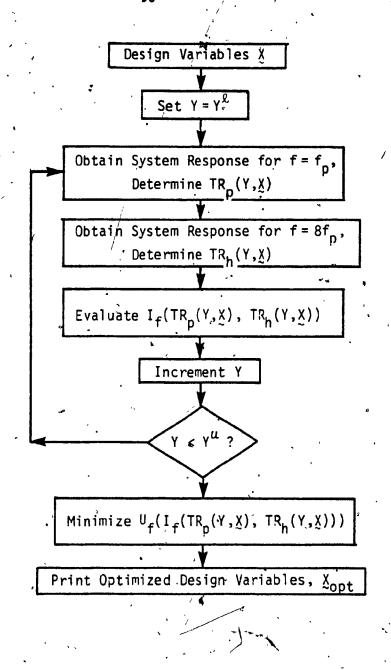
Fig. 6.1: Flowchart of the Optimization Procedure-Frequency Domain
