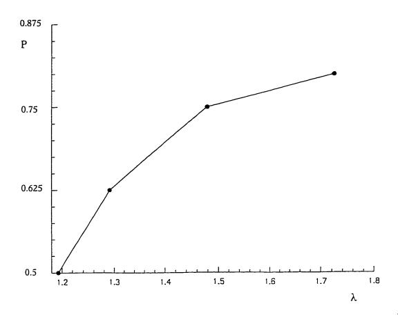
Fig. 5.1a Dimensionless pressure vs principal stretch  $\lambda$ , Varga material
