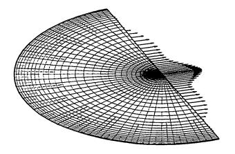
Fig. 5.9h Distribution of principal Piola stress  $w_{\mu}$  along a meridian passing through zone-centered points; reference configuration
