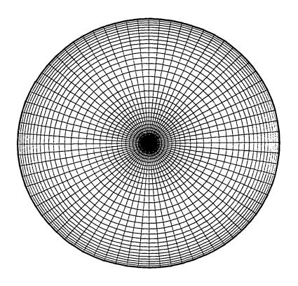
Fig. 5.9a Circular membrane; meshed reference configuration
