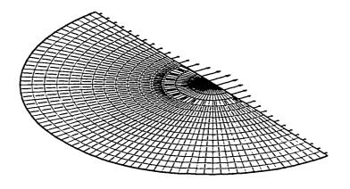
Fig. 5.7g Distribution of principal Piola stress  $w_{\lambda}$  along a meridian passing through zone-centered points; reference configuration
