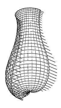
Fig. 5.11d Distribution of principal Cauchy stress  $w_{\mu}\lambda^{-1}$  along a generatrix passing through zone-centered points
