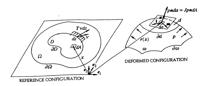
Fig. 2.1 Equilibrium of the region  $D \subset \Omega$  of the membrane
