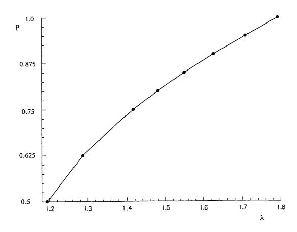
Fig. 5.1b Dimensionless pressure vs principal stretch  $\lambda$ , Mooney-Rivlin material
