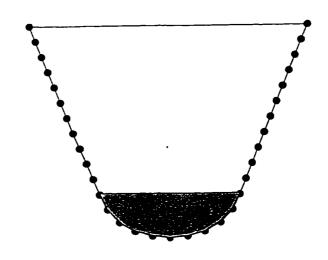
Fig. 5.7b Cross-section through a meridian of the deformed configuration; liquid level shown
