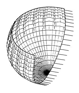
Fig. 5.6c Distribution of principal stretch  $\,\lambda\,$  along a meridian passing through zone-centered points
