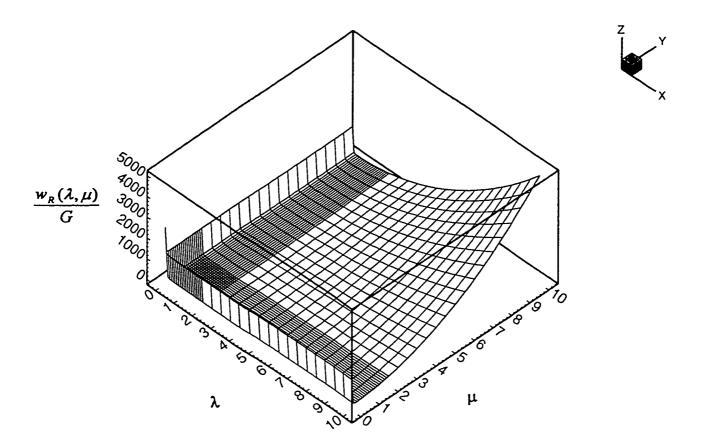
Fig. 5.3a Original Mooney-Rivlin strain energy function,
