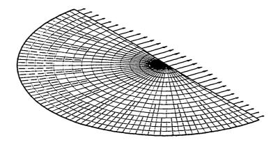
Fig. 5.6g Distribution of principal Piola stress  $w_{\lambda}$  along a meridian passing through zone-centered points; reference configuration
