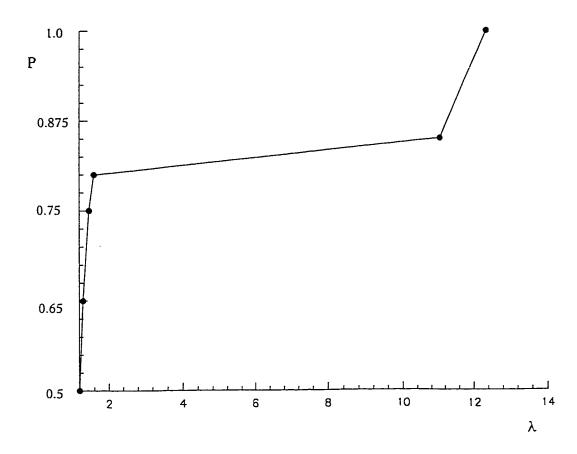
Fig. 5.1d Dimensionless pressure vs principal stretch  $\lambda$ , Ogden material
