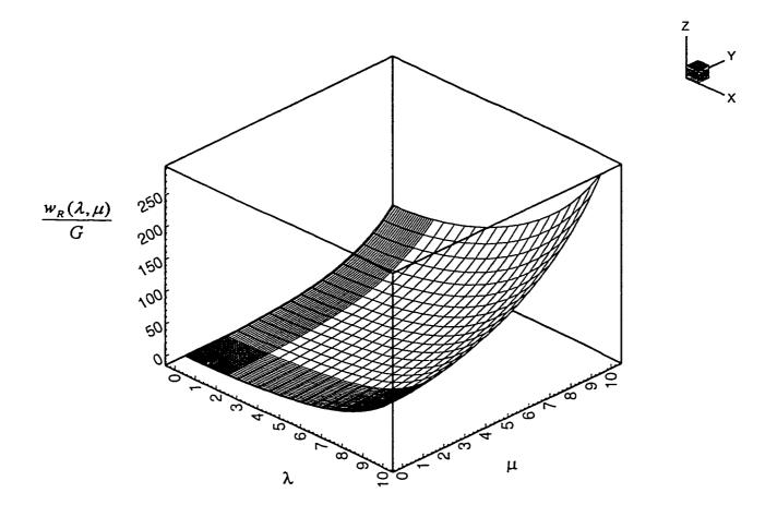
Fig. 5.5b Relaxed Ogden strain energy function,
