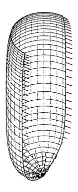
Fig. 5.10e Distribution of principal Cauchy stress  $w_{\mu} \lambda^{-1}$  along a generatrix passing through zone-centered points
