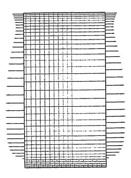
Fig. 5.11f Distribution of principal Piola stress  $w_{\mu}$  along a generatrix passing through zone-centered points; reference configuration
