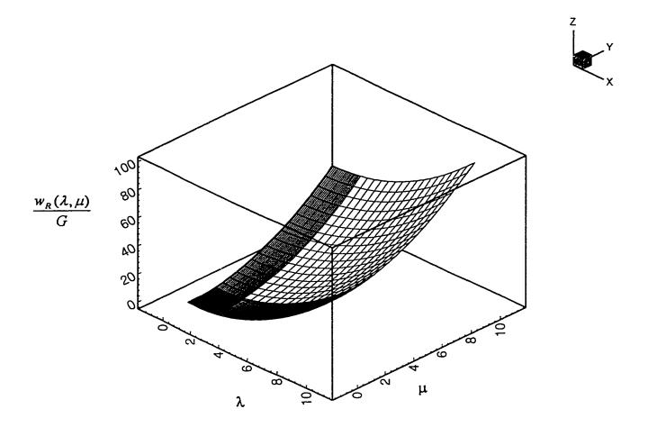
Fig. 5.4b Relaxed neo-Hooken strain energy function,
