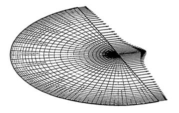
Fig. 5.9g Distribution of principal Piola stress  $w_{\lambda}$  along a meridian passing through zone-centered points; reference configuration
