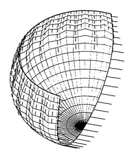
Fig. 5.6d Distribution of principal stretch  $\,\mu$  along a meridian passing through zone-centered points
