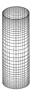
Fig. 5.10a Cylindrical Mooney-Rivlin membrane; meshed reference configuration
