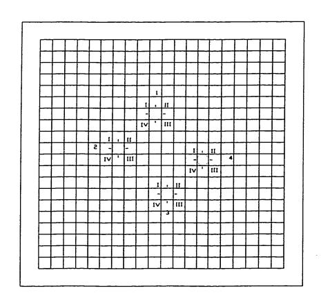
Fig. 6.1d Experimental model of square membrane; location of testing dots shown
