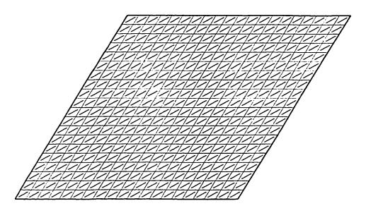
Fig. 6.1b Square membrane subjected to shearing (35°)
