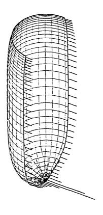
Fig. 5.10d Distribution of principal Cauchy stress  $w_{\lambda} \mu^{-1}$  along a generatrix passing through zone-centered points
