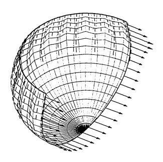
Fig. 5.6e Distribution of principal Cauchy stress  $w_{\lambda} \mu^{-1}$  along a meridian passing through zone-centered points
