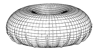
Fig. 5.9c Circular Ogden membrane simultaneously subjected to internal uniform pressure and external pressure loading of a hydrostatic type, combined with a 50% contraction of the boundary
