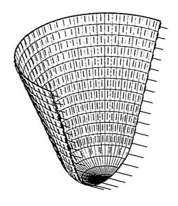
Fig. 5.7d Distribution of principal stretch  $\,\mu$  along a meridian passing through zone-centered points
