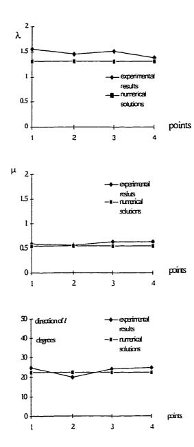
Fig. 6.1i Comparison of numerical results and experimental solutions; shearing angle of 45°
