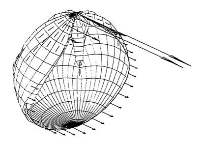
Fig. 5.8b Distribution of principal Cauchy stress  $w_{\lambda} \mu^{-1}$  along a meridian passing through zone-centered points
