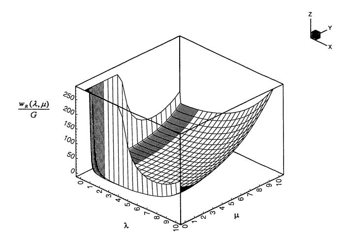
Fig. 5.5a Original Ogden strain energy function,
