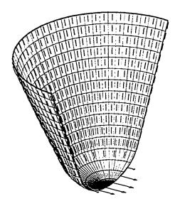
Fig. 5.7f Distribution of principal Cauchy stress  $w_{\mu} \lambda^{-1}$  along a meridian passing through zone-centered points
