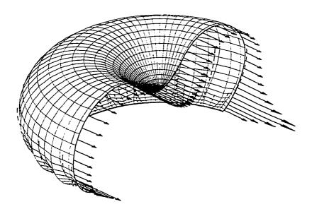
Fig 5.9e Distribution of principal Cauchy stress  $w_{\lambda}\mu^{-1}$  along a meridian passing through zone-centered points
