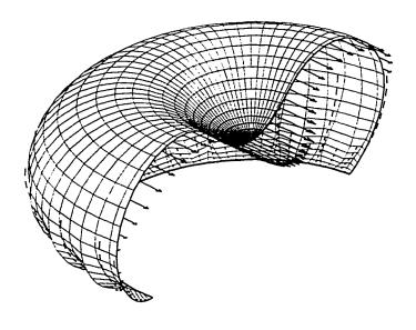
Fig. 5.9f Distribution of principal Cauchy stress  $w_{\mu}\lambda^{-1}$  along a meridian passing through zone-centered points
