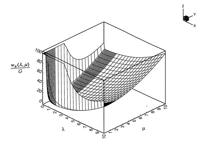
Fig. 5.4a Original neo-Hooken strain energy function,
