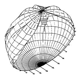
Fig. 5.8c Distribution of principal Cauchy stress  $w_{\mu} \lambda^{-1}$  along a meridian passing through zone-centered points
