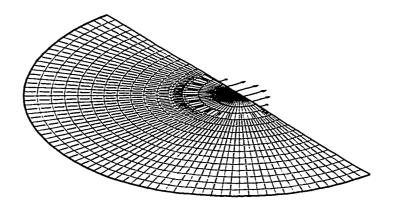
Fig. 5.7h Distribution of principal Piola stress  $w_{\mu}$  along a meridian passing through zone-centered points; reference configuration
