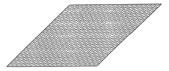
Fig. 6.1c Square membrane subjected to shearing (45°)
