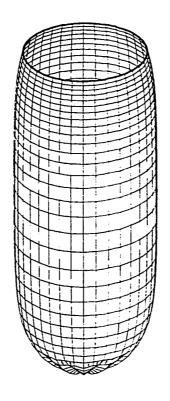
Fig. 5.10c Cylindrical Mooney-Rivlin membrane, subjected to uniform pressure,
