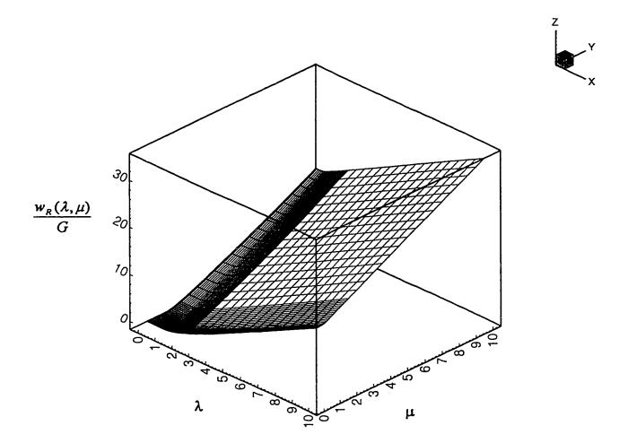
Fig. 5.2b Relaxed Varga strain energy function,
