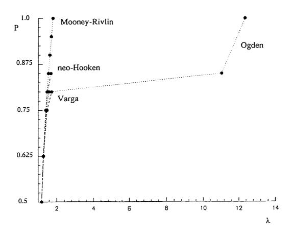
Fig. 5.1e Dimensionless pressure vs principal stretch  $\lambda$ , Varga, Mooney-Rivlin, neo-Hooken, Ogden material
