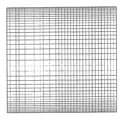
Fig. 5.10b Square Mooney-Rivlin membrane; meshed reference configuration
