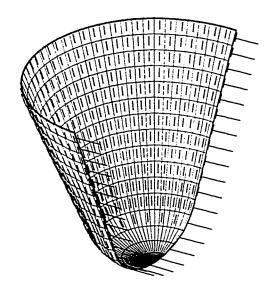
Fig. 5.7c Distribution of principal stretch  $\,\lambda\,$  along a meridian passing through zone-centered points
