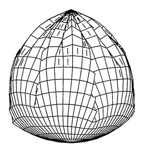
Fig. 5.8a Circular Mooney-Rivlin membrane totaly subjected to hydrostatic pressure, combined with a 100% contraction of boundary
