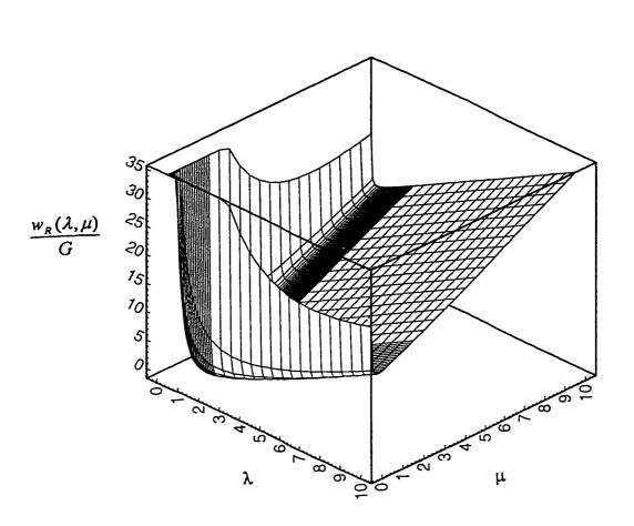
Fig. 5.2a Original Varga strain energy function,
