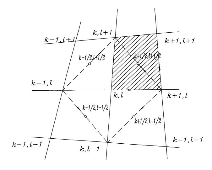
Fig. 3.1 Mesh for spatial discretization, with integration paths used in Green's theorem differencing method
