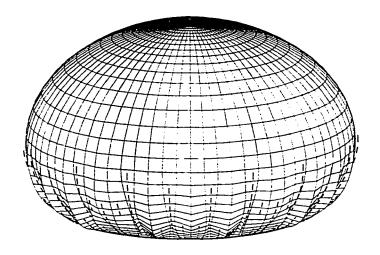
Fig. 5.9b Circular Ogden membrane totally subjected to a uniform pressure, combined with a 50% contraction of the boundary
