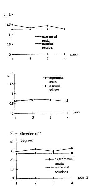
Fig. 6.1h Comparison of numerical results and experimental solutions; shearing angle of 35°
