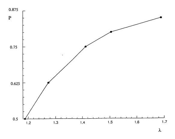
Fig. 5.1c Dimensionless pressure vs principal stretch  $\lambda$ , neo-Hooken material
