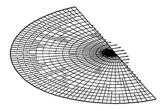
Fig. 5.8e Distribution of principal Piola stress  $w_{\mu}$  along a meridian passing through zone-centered points; reference configuration
