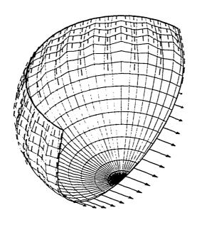
Fig. 5.6f Distribution of principal Cauchy stress  $w_{\mu}\lambda^{-1}$  along a meridian passing through zone-centered points
