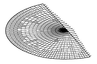
Fig. 5.8d Distribution of principal Piola stress  $w_{\lambda}$  along a meridian passing through zone-centered points; reference configuration
