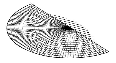
Fig. 5.6h Distribution of principal Piola stress  $w_{\mu}$  along a meridian passing through zone-centered points; reference configuration
