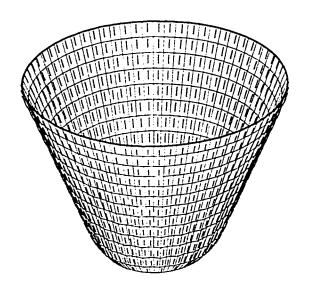
Fig. 5.7a Circular Ogden membrane partly subjected to hydrostatic pressure, combined with a 50% contraction of boundary
