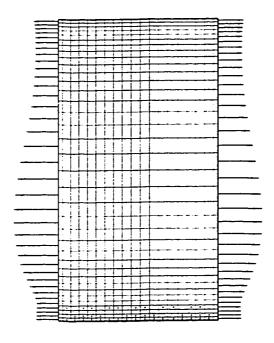
Fig. 5.11e Distribution of principal Piola stress  $w_{\lambda}$  along a generatrix passing through zone-centered points; reference configuration
