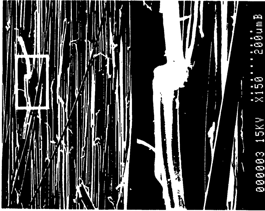
Figure 4.17c. SEM of the fracture surface of AC40-66 laminate exposed to 87°C/84% (MC=0.18%) at X150 and X750.
