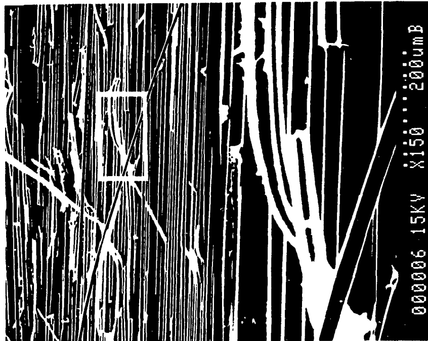
Figure 4.17f. SEM of the fracture surface of AC40-66 laminate exposed to 127°C/84% (MC=0.08%) at X150 and X750.
