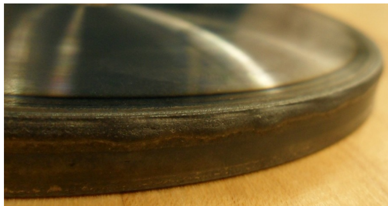
Fig 4.15 Remarkable distortion on disc #1 lateral face due to the most input IH Energy
