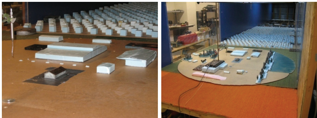
Figure 4.9 Test building and surroundings model placed in the wind tunnel.
