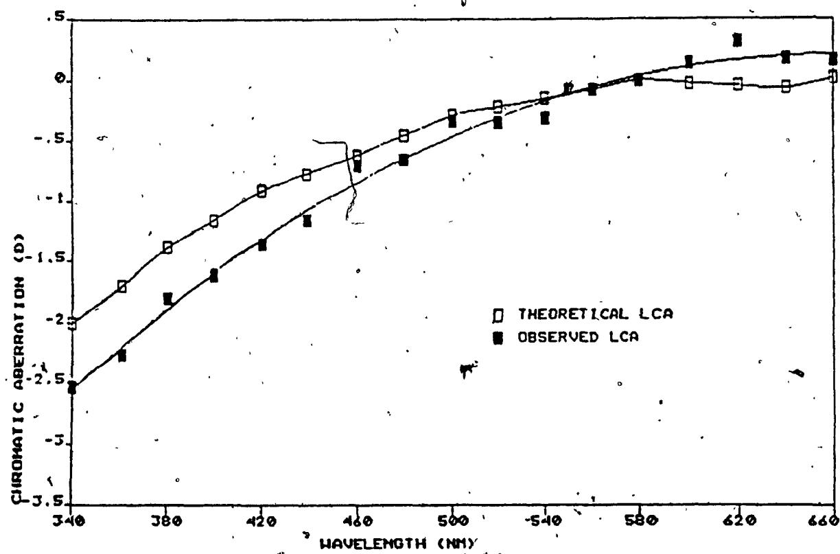
Figure 10. The theoretical and observed comparison for observer SH.
