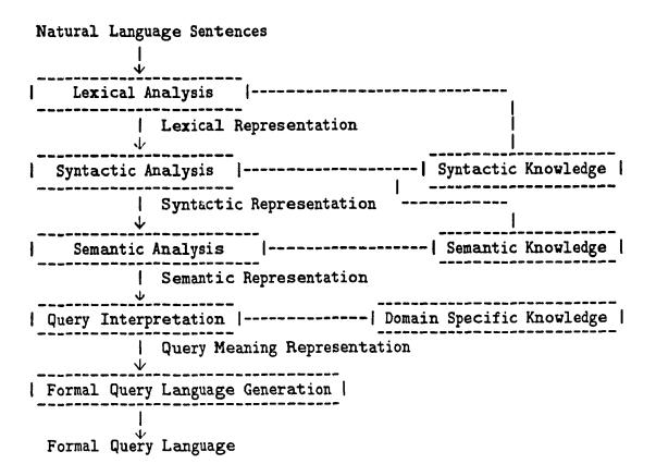
Figure 2.1: General Design Architecture of a Natural Language Interface to Database Query System
