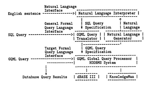
Figure 5.1: Enhanced Architecture of MIDBMS System
