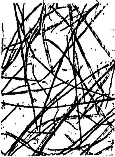
Fig. 1-1 Unbeaten soft-wood fibers.
