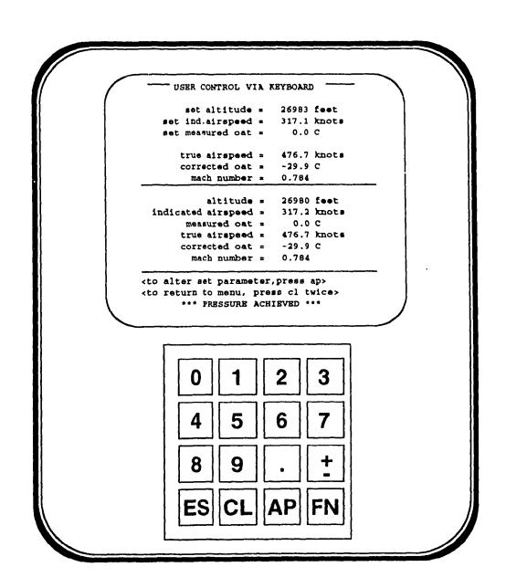
6) You are still going through the process to pressurize the system. You want to pressurize to 30000 feet, 250 knots and 10 degrees C.
