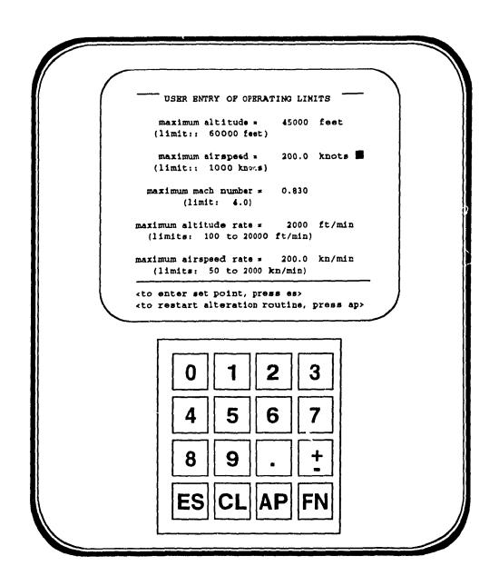
1) You are on the User Entry of Operating Limits page. The cursor is flashing on the maximum airspeed line. The value that is displayed (200.0) does not need to be changed. How do you move on to change the mach number value?
