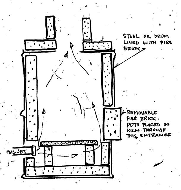
Figure 3. Diagram of Simple Up-Draught Raku Kiln
