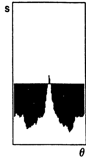
(d3) result of matching (d2) against fig. 5.1(b1), peak found at (\theta, score) = (88^\circ, 20) ;
