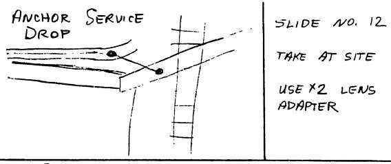
TOGETHER WITH A HELPER THE LINE FROM THE POLE IS ANCHORED TO THE BUILDING IN A TEMPORARY ARRANGEMENT, ENSURE THE ANCHOR CAN SAFELY HOLD THE WIRES SINCE FN UNTIMELY RELEASE COULD BE FATAL.
