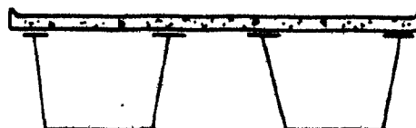
- two separate boxes concrete deck
