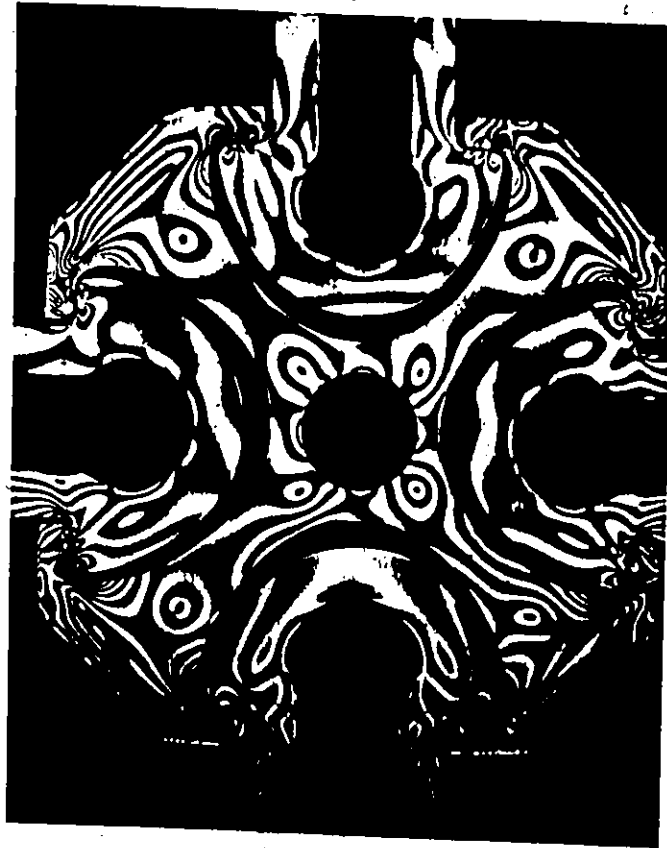
FIGURE 4.26 STRESSES IN ONE DESIGN OF THE FOUR-WAY EXTRUSION LOADED IN FOUR DIRECTIONS
