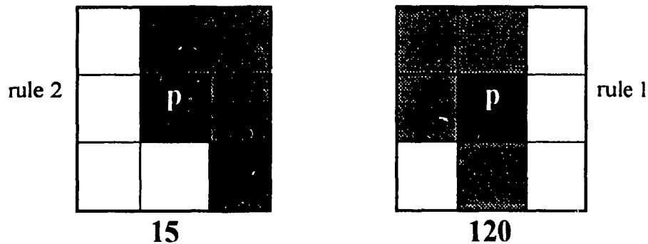
Figure 25: 2 templates from Chin's thinning set favoring diagonal over straight lines.
