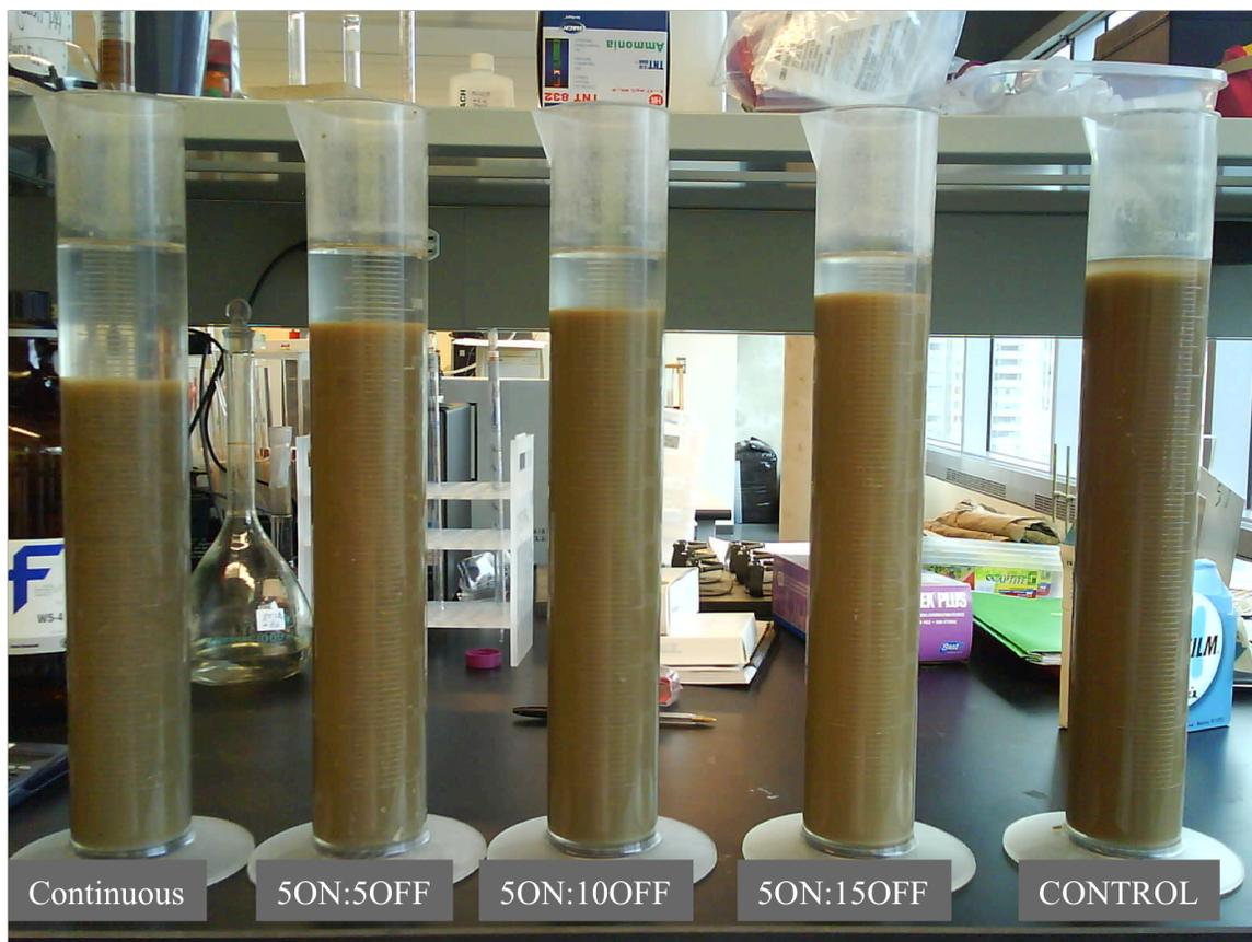
Figure A-1 Sample picture of variations in SVI after 48 hours of operation among different electrical modes
