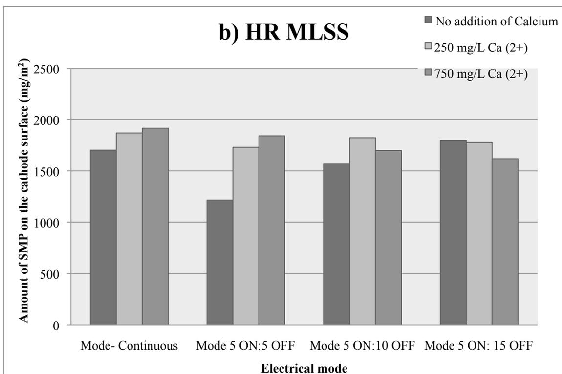
Figure 4-39 Amount of SMP desorbed from cathode surface (mg/m<sup>2</sup>) a) LR MLSS b) HR MLSS
