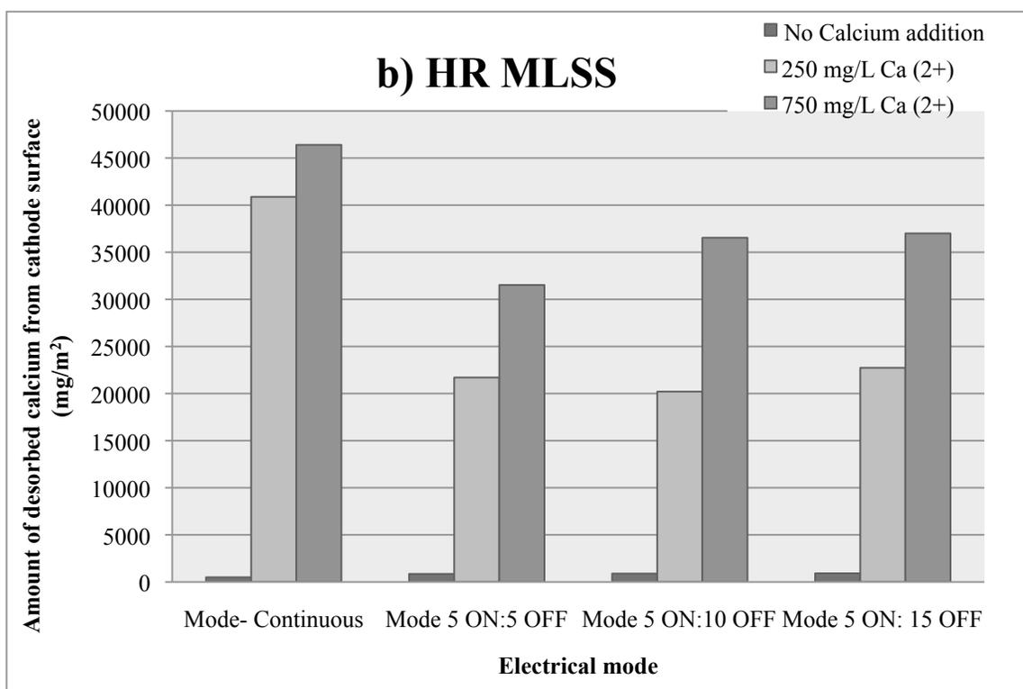
Figure 4-35 Amount of calcium desorbed from cathode surface a) LR MSS b) HR MLSS
