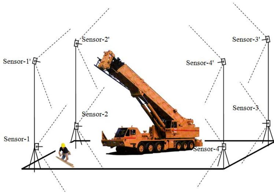
*Figure 3-4 UWB RTLS Used in Crane Operation (Zhang, 2010)*
