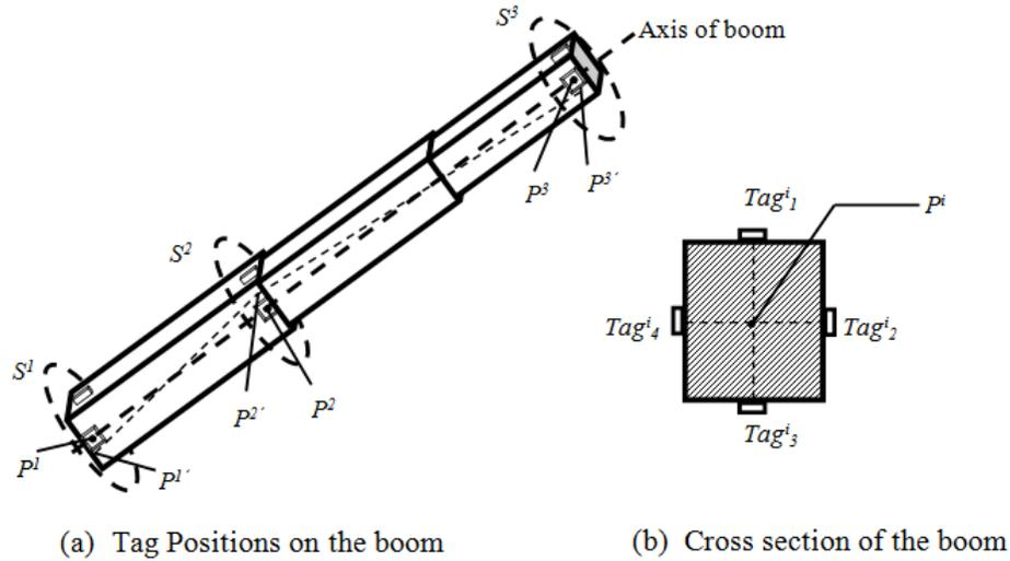
*Figure H-1 Tag Positions in Test of Tracking the Motion of a Crane (adapted from Zhang, 2010)*
