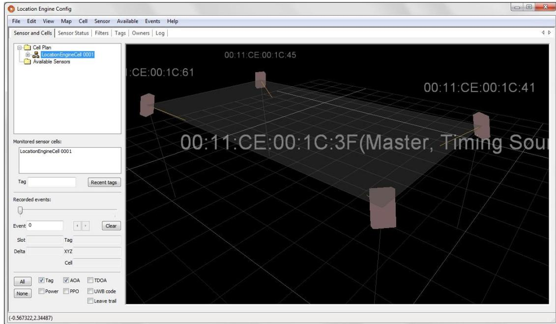
*Figure 5-5 3D View of a Cell in Ubisense Location Engine Configuration*
