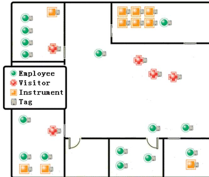
*Figure 3-2 UWB RTLS Use in Employee Monitoring*
