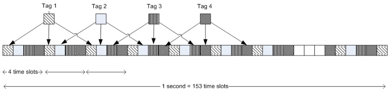
*Figure 3-1 4 Timeslots of Slot Interval for a 160 Hz System (Rodriguez, 2010)*
