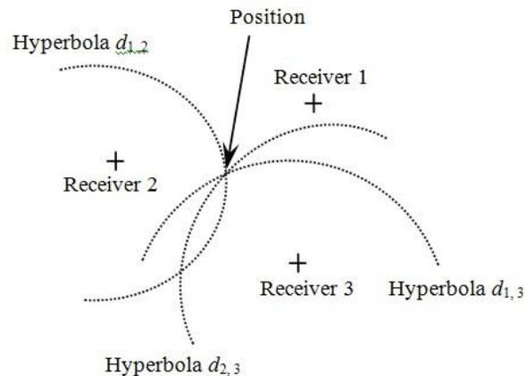
Figure 2-7 TDOA Positioning Principle (Ghavami et al., 2004)
