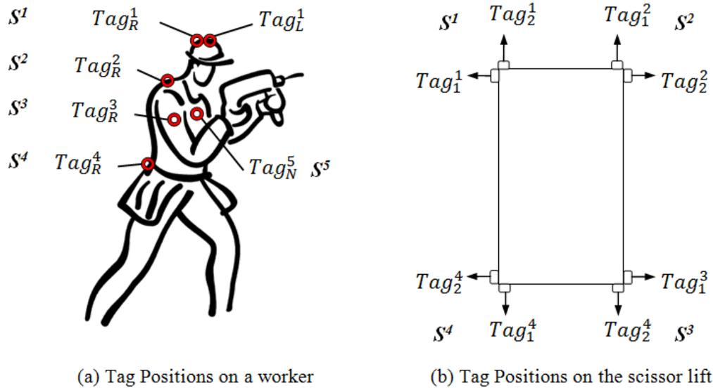
Figure G-1 Tag Positions in Test of Tracking Workers in a Construction Project
