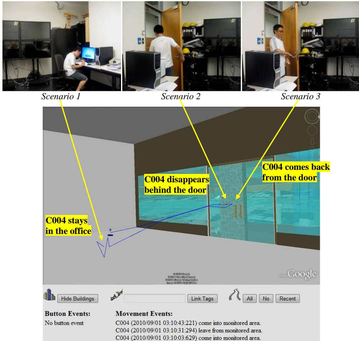
*Figure 6-1 Visualization of Simulated Test of Employee Monitoring*
