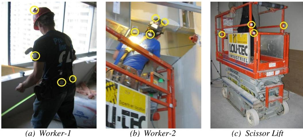
*Figure 6-4 Tag Positions in Test of Tracking Workers in a Construction Project*
