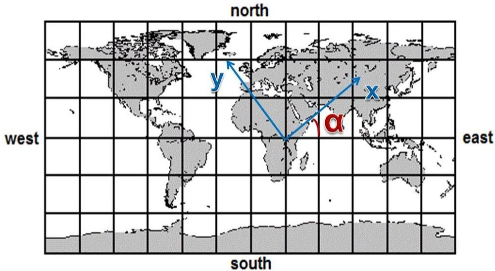
*Figure 5-11 Angle between the X Axis of a Cell and the East Direction*
