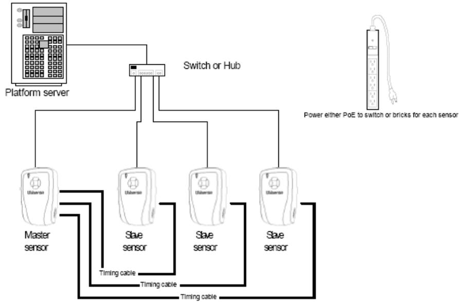
Figure 5-2 Installation of Ubisense Sensors (Ubisense, 2009)
