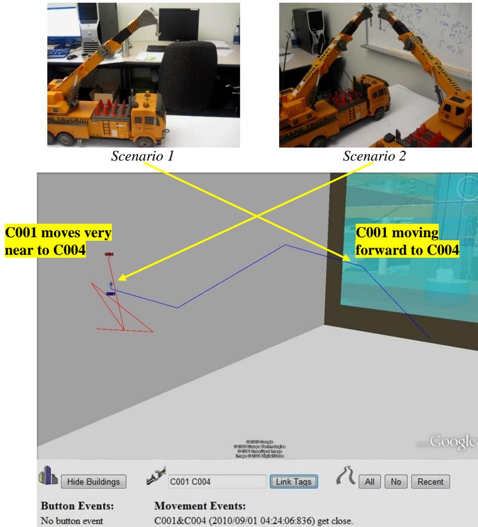
Figure 6-3 Visualization of Simulated Test of Crane Operation
