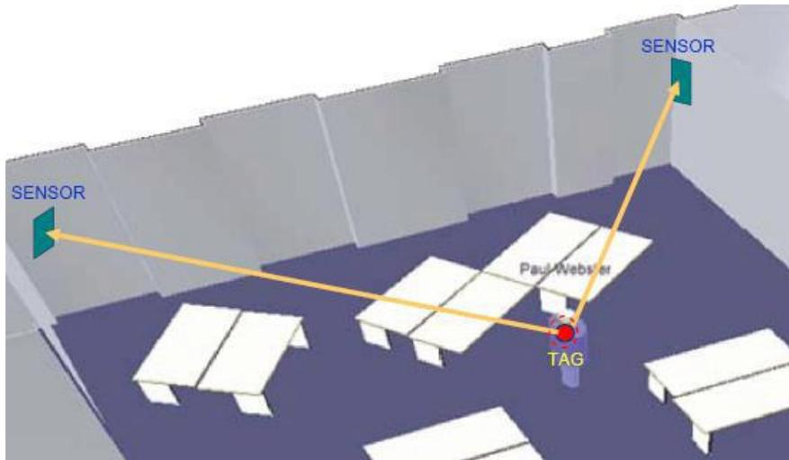
*Figure 2-5 UWB Technology Employed in RTLS*
