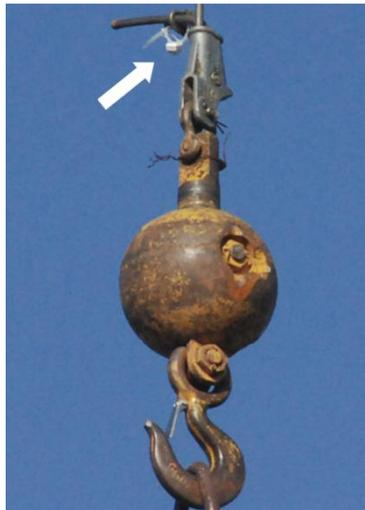
**Figure 2-24: UWB tag on hook (Teizer et al., 2007)**
