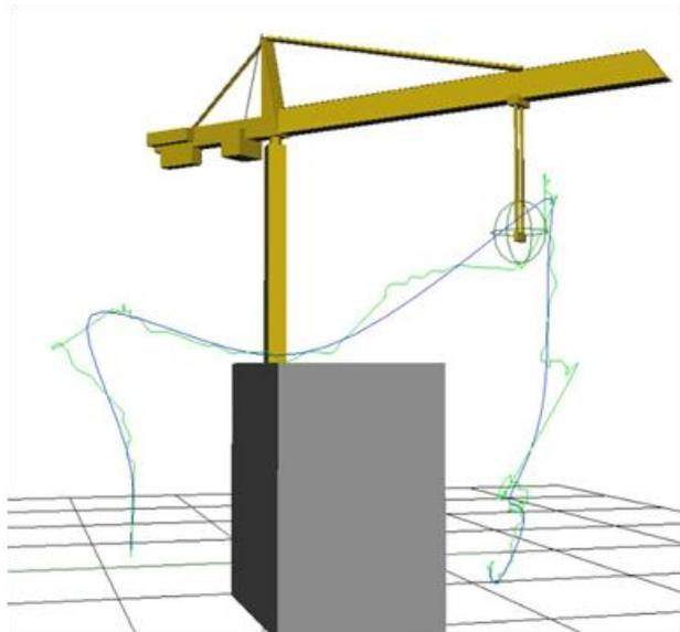
**Figure 5-11: Path trace of the tower crane hook**
