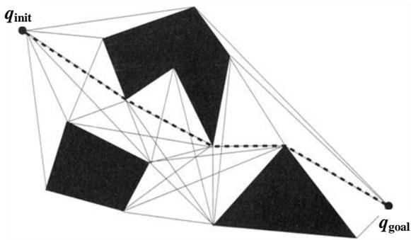
**Figure 2-9: Example of a visibility graph (Choset et al., 2005)**
