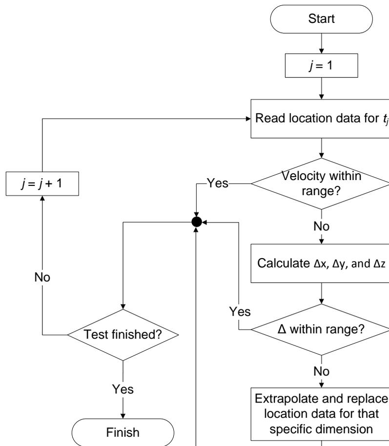
Figure 5-27: Flowchart of near real-time data processing for single tags
