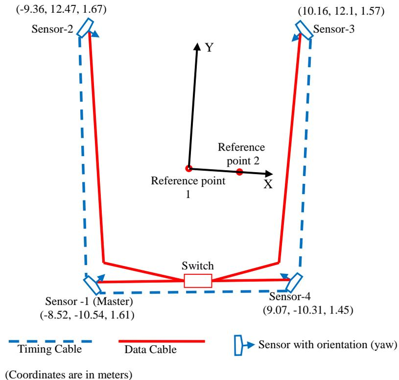
**Figure 5-21: Outdoor setting of sensor cell**
