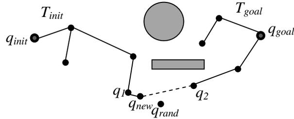
**Figure 4-5: Merging two RRTs (Adapted from Choset et al., 2005)**
