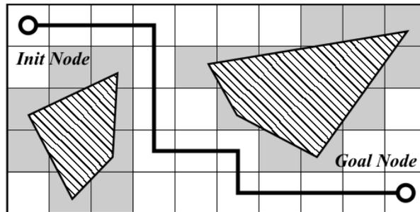
**Figure 2-8: Grid example of A\* algorithm (Adapted from Bruce, 2004)**
