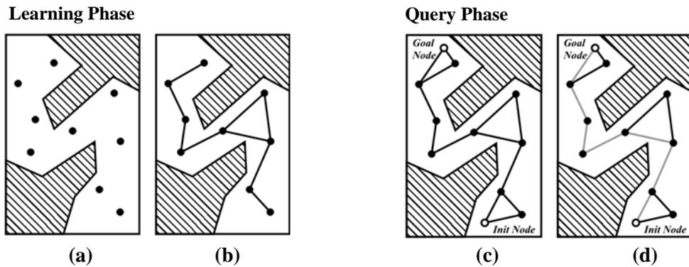
**Figure 2-10: Example of PRM algorithm steps (Adapted from Bruce, 2004)**
