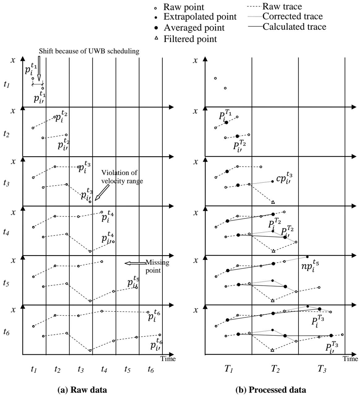
**Figure 5-5: Near real-time data processing of two tags**
