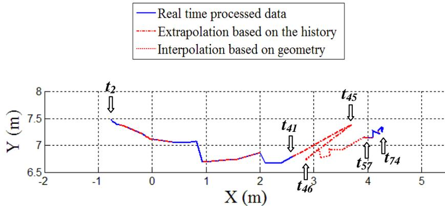
**Figure 5-28: Trace of  $Tag_1^2$  based on extrapolation of its history and interpolation of other two tags**
