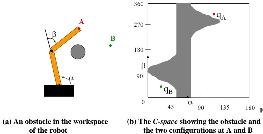
**Figure 2-7:  $C$ -space of a two-link arm robot (Choset et al., 2005)**
