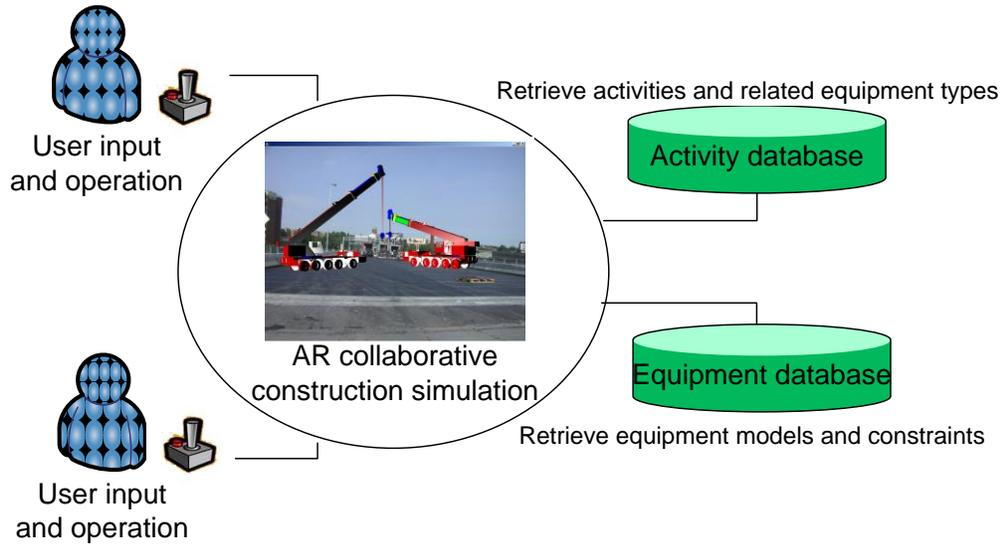
Figure 2-28: Distributed augmented reality system for supporting multi-user interaction using ad-hoc wireless networking (Hammad et al., 2009)
