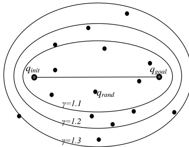
**Figure 4-7: Nodes with different smoothness values**
