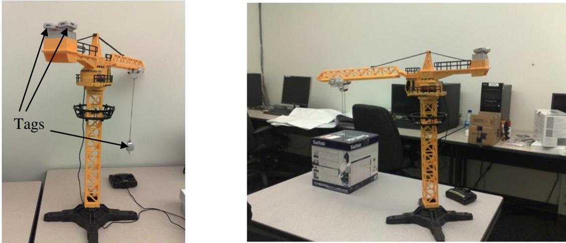
**Figure 5-10: Tower crane model with tags**
