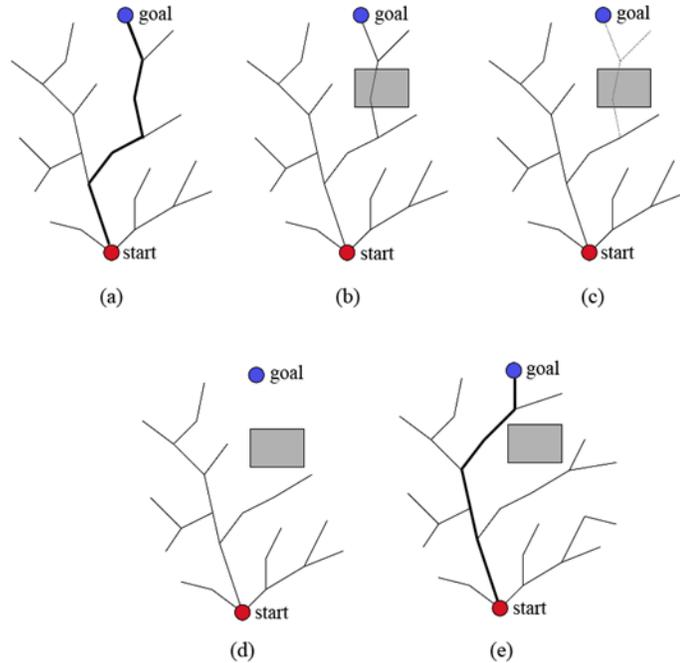
**Figure 4-6: DRRT steps for re-planning (Adapted from Ferguson et al., 2006)**
