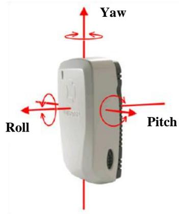
**Figure 3-5: Yaw, Roll and Pitch angles of a sensor (Ubisense, 2010)**
