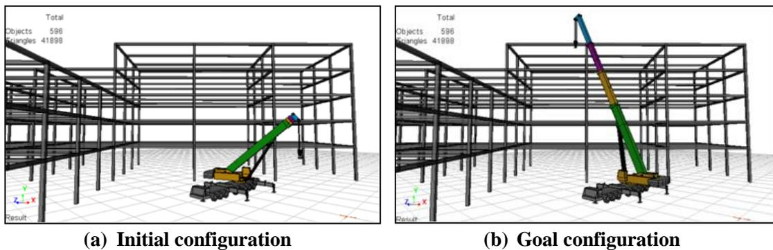
**Figure 4-14: Initial and goal configurations of the crane**
