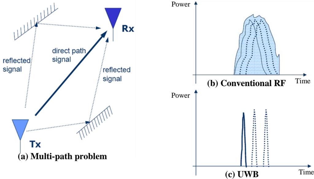
**Figure 2-22: Multi-path problem with conventional RF and UWB (Ubisense, 2010)**
