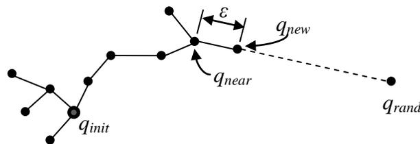
**Figure 4-2: The Extend operation (LaValle and Kuffner, 2001)**
