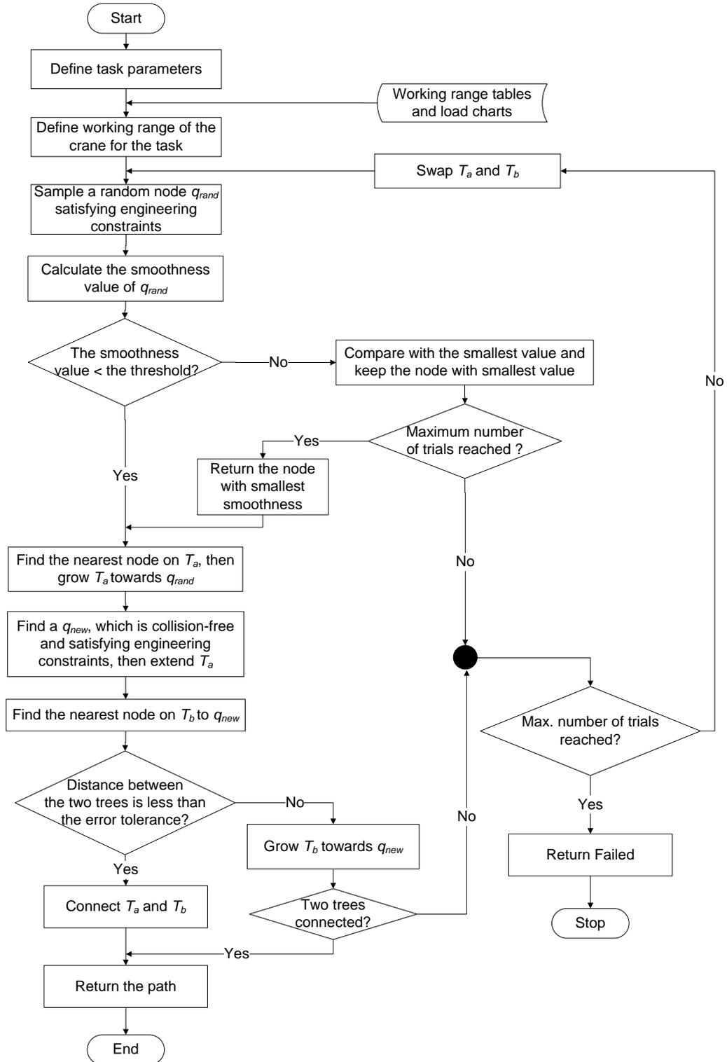
**Figure 4-9: Flowchart of motion planning algorithm RRT-Con-Con-Mod**
