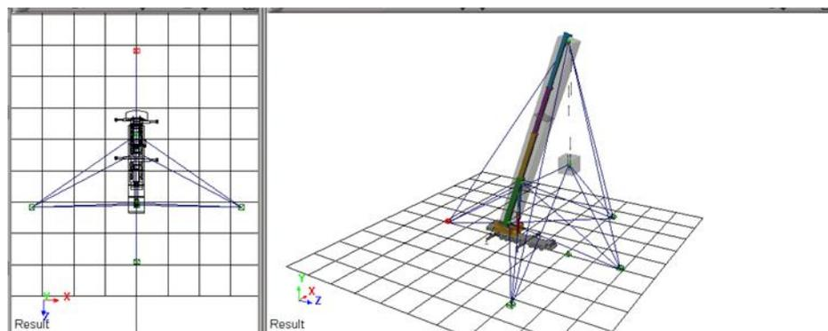
**(c) One sensor facing the back of the crane and three sensors facing its front**
