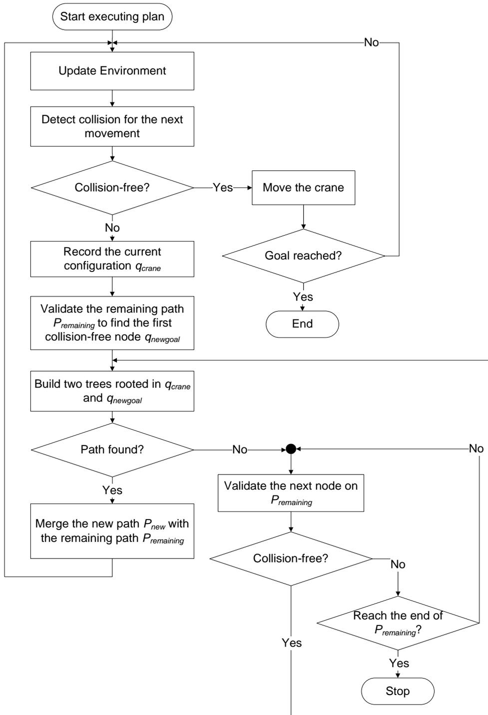
**Figure 4-13: Flowchart of re-planning algorithm DRRT-Con-Con-Mod**
