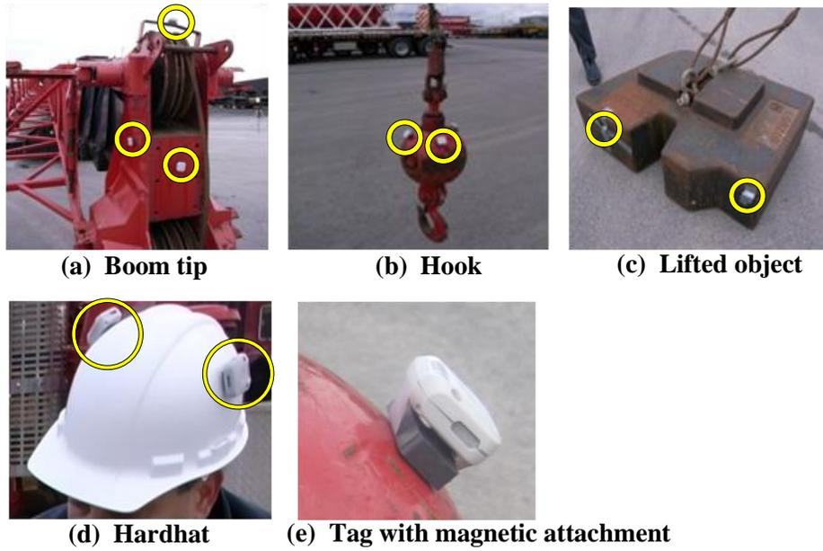
Figure 5-23: Tags attached to different objects
