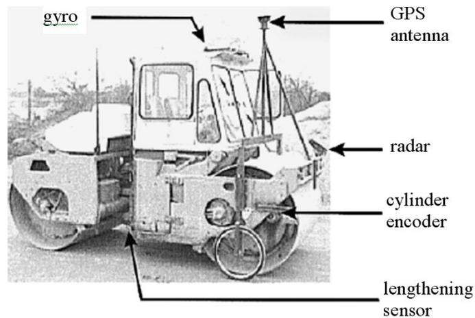
**Figure 2-25: Instrumented compactor (Bouvel et al., 2001)**
