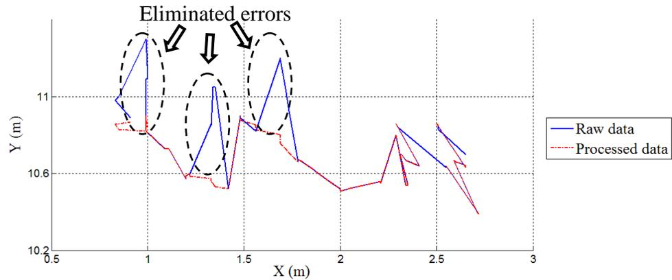
**Figure 5-32: Comparison of traces of  $Tag_1^1$  in X-Y plane before and after correction using post processing**
