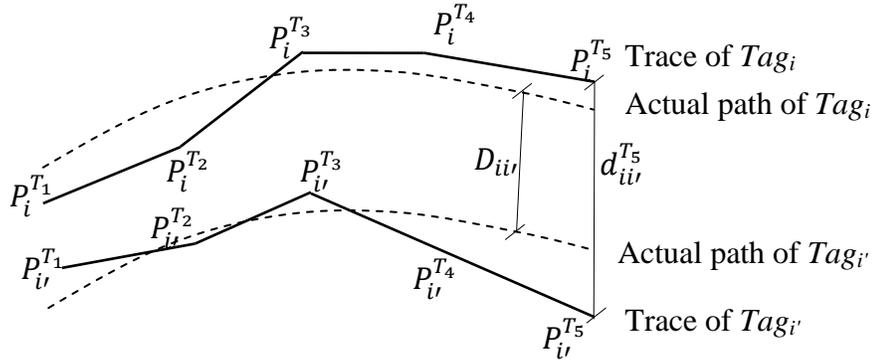
**Figure 5-6: Example of using geometric constraints to detect errors**
