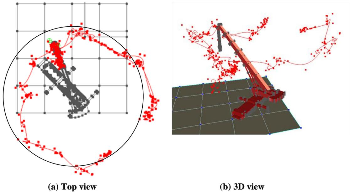
**Figure 6-5: Boom tip trace based on averaging the locations of three tags**
