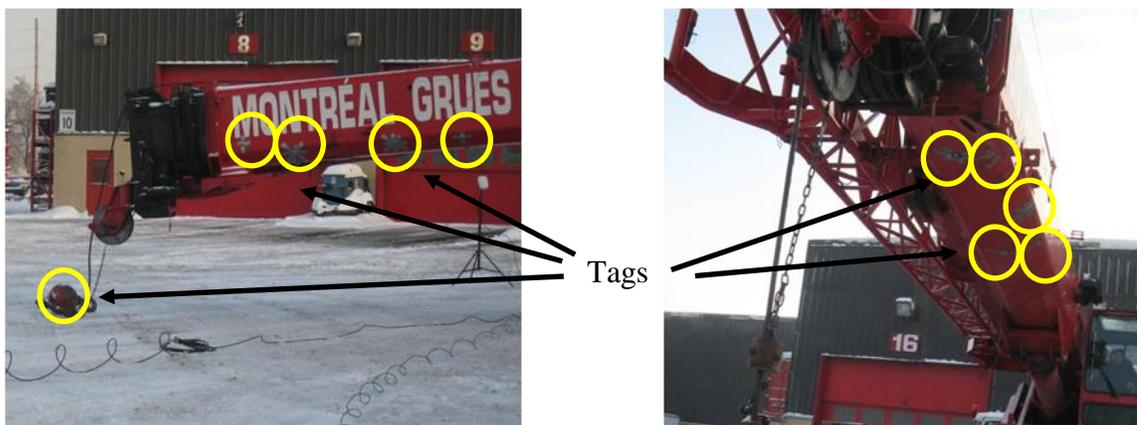
**Figure 5-20: Tags attached to the boom and the hook**
