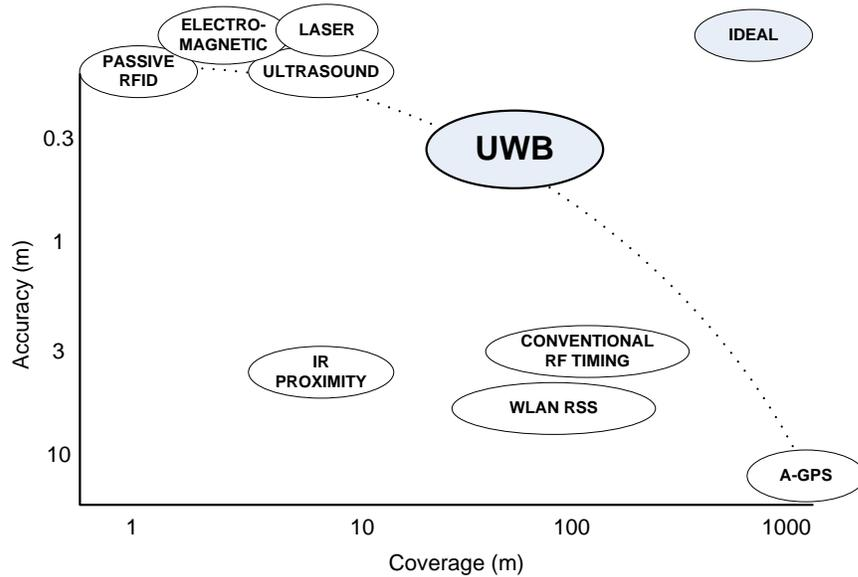
**Figure 2-21: Comparison of location technologies (adapted from Ward, 2007)**
