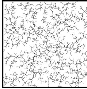
**Figure 2-12: Example of an RRT with 2000 vertices (LaValle and Kuffner, 1999)**
