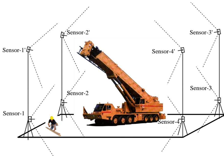
**Figure 5-2: Vertical coverage of sensors at two elevations**
