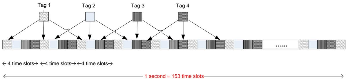
**Figure 3-6: Tag updates for a 160 Hz system with slot interval of 4 time slots**
