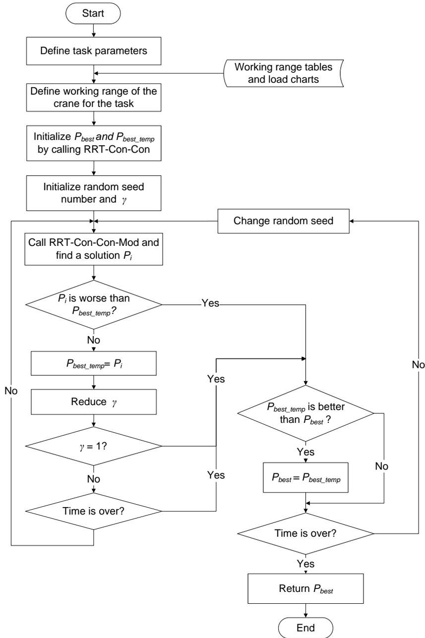
**Figure 4-11: Flowchart of anytime motion planning algorithm**
