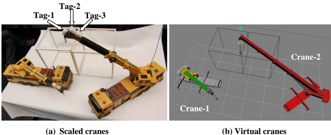
**Figure 6-6: The scaled cranes and their virtual models**
