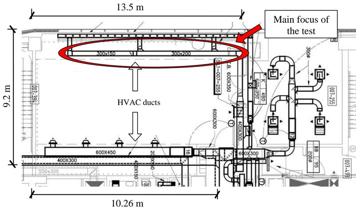
**Figure 5-12: Dimensions of the monitored area**
