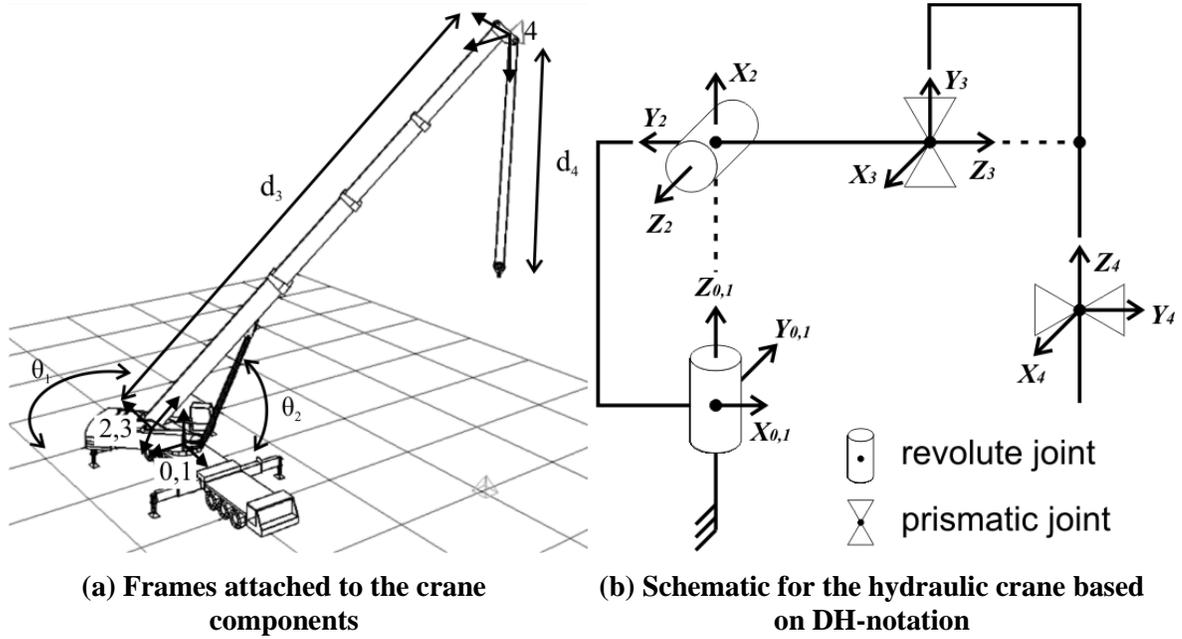
**Figure 3-3: Defining the kinematic structure for a hydraulic crane (AlBahnassi and Hammad, 2010)**
