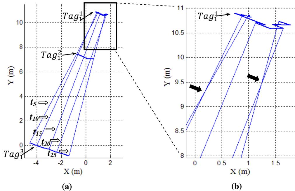
**Figure 5-30: Data processed in real time showing the traces of three tags at different time**
