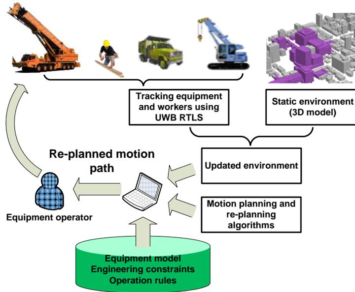
**Figure 3-1: Conceptual near real-time environment updating and intelligent assistance for cranes**
