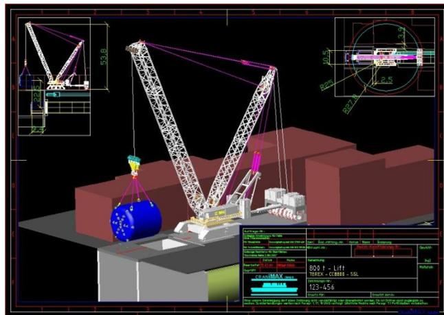
**Figure 2-5: Crane positioned in a 3D environment (Cranimax, 2010)**
