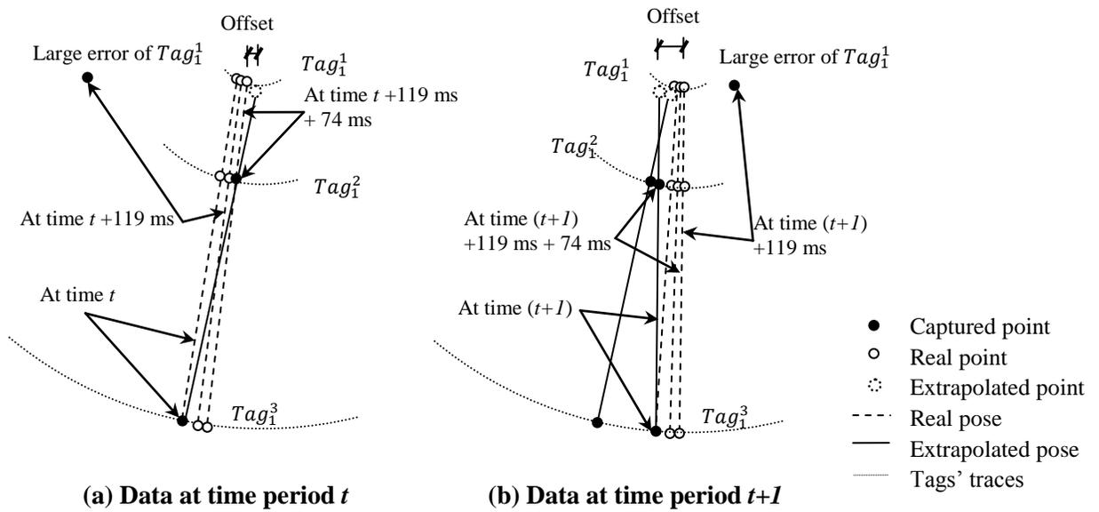
**Figure 5-29: Conceptual figure of extrapolation errors**
