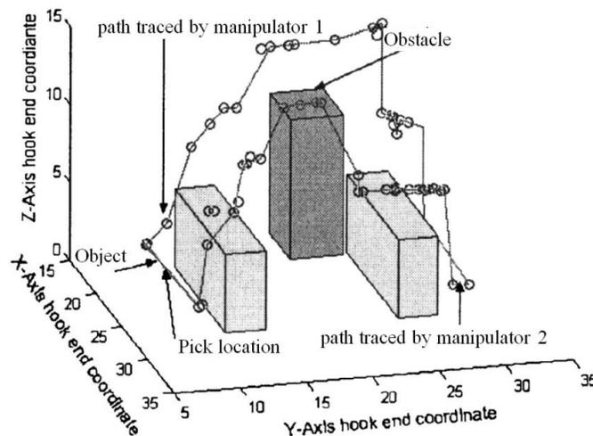
**Figure 2-13: Paths of cooperative manipulators using GA (Ali et al., 2005)**
