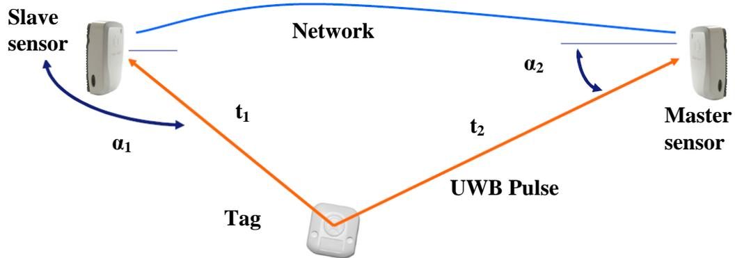
**Figure 2-23: Signals sent to sensors are used to calculate the 3D position of a tag (Ubisense, 2010)**
