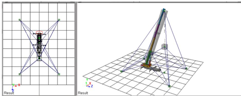
**Figure 5-4: Example of a test setting for monitoring a crane**
