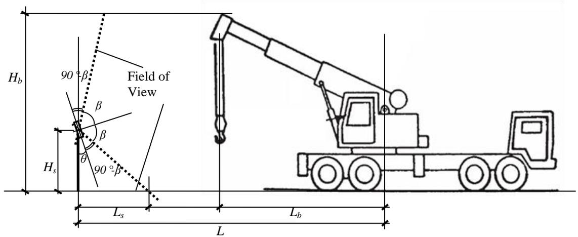
**Figure 5-3: Parameters for defining sensor position and orientation**
