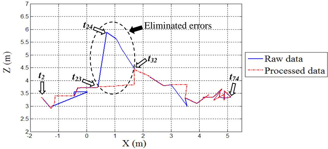
Figure 5-26: Comparison of traces of Tag<sub>3</sub><sup>2</sup> in X-Z plane before and after correction
