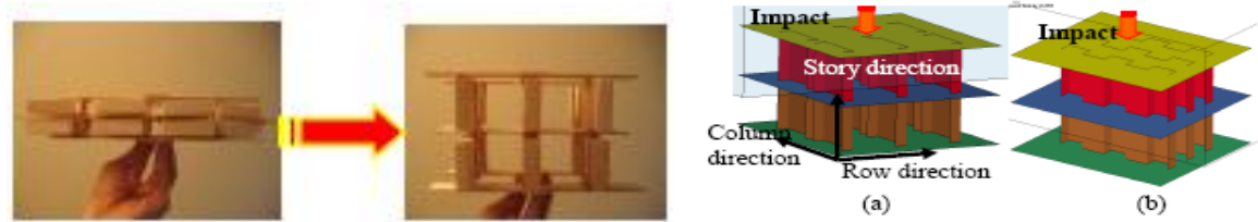
Figure 1.18: A pictorial view (left) and schematics (right) of expandable lattice structure: (a) U-shaped thin walled members; and (b) rectangular jagged members [19]
