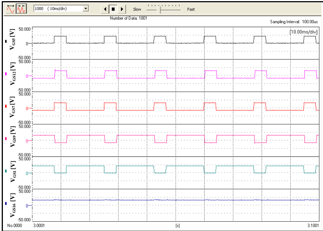
Fig. 4-7. V_{GS} (gate-to-source voltage) of switches S_5 , S_{12} , S_7 , S_9 , S_1 , and S_{16} .
