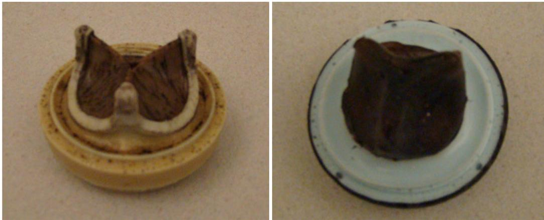
Figure 3.8 (a) Biological aortic pericardial valve; (b) home-made stenotic silicone valve.
