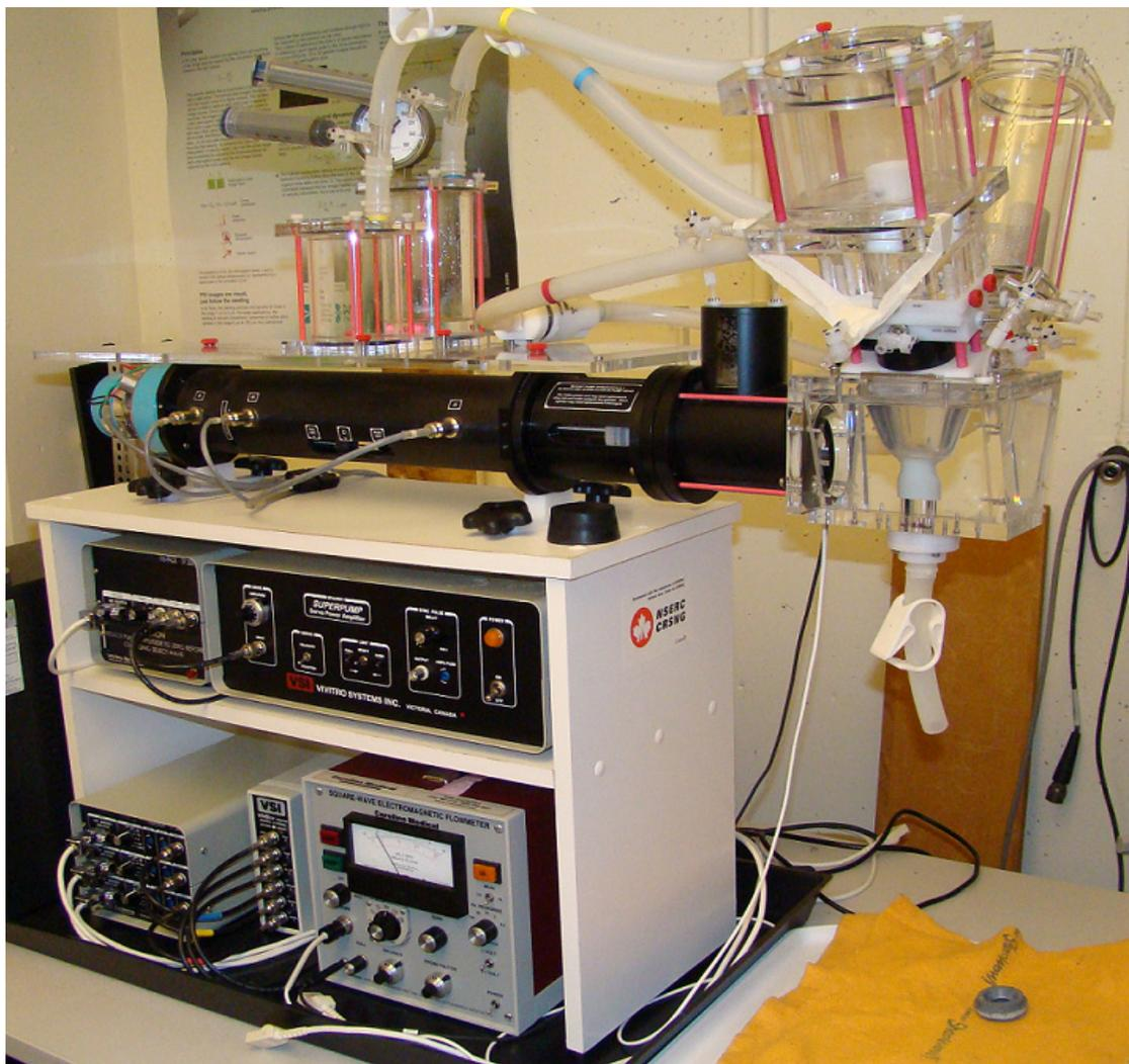
Figure 3.1 Front view of the left heart simulator.
