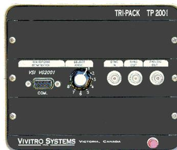
Figure 3.7 Front panel of the waveform generator unit.
